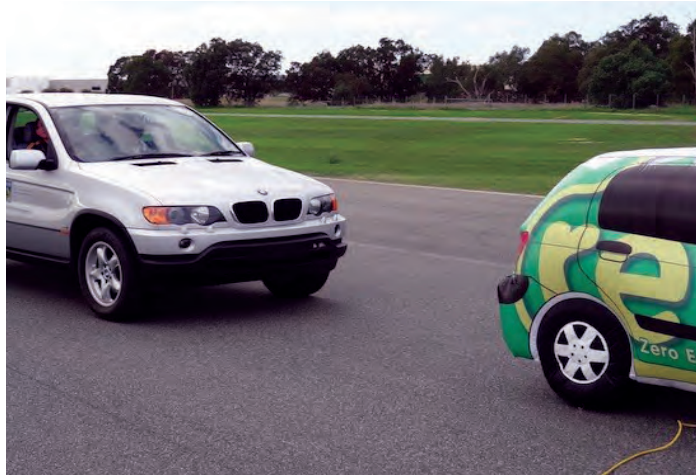
The BMW steer-by-wire in collision avoidance testing
