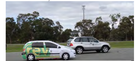
Above and below: The BMW steers autonomously around a stationary vehicle
