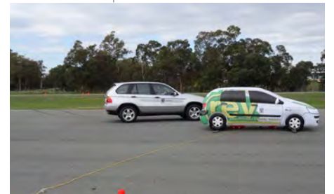
Above and below: The BMW steers autonomously around a stationary vehicle
