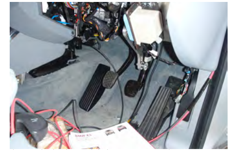
Above: The brake-pedal electric servo in the BMW
