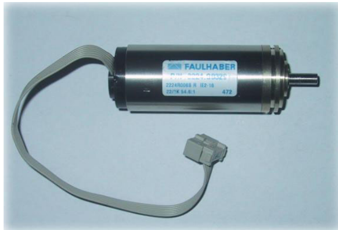
Figure 4.2: Faulhaber DC Motor 2224R006S with inbuilt gearbox and encoders
