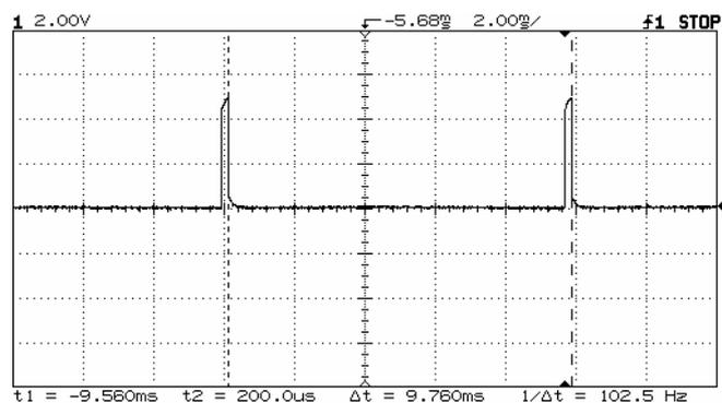
**Figure 6.2: Two pulses separated by approximately 10ms**
