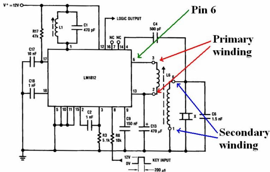
**Figure 6.16: Location of pin 6 and transformer windings on the circuit diagram [14]**
