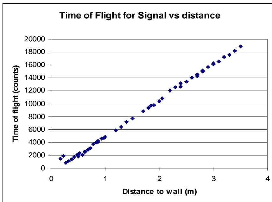
**Figure 6.11: Calculated time of flight over a range of distances for the echo sounder**
