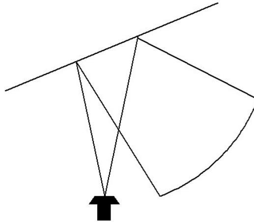
**Figure 7.2: No returned echo at an angle greater than half the beamwidth**
