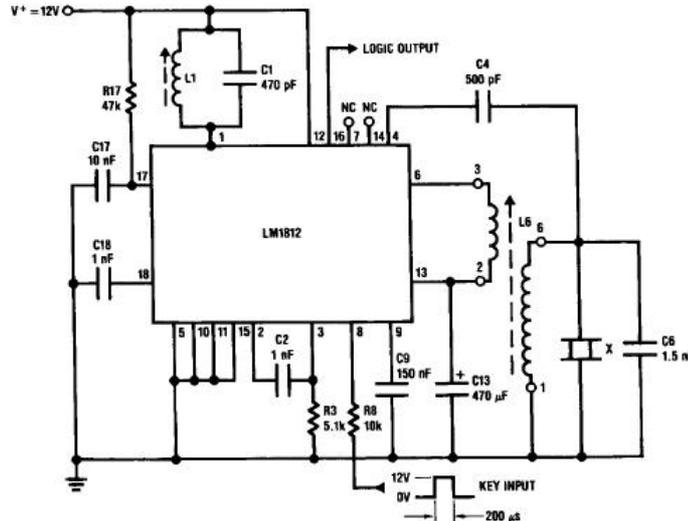
**Figure 4.5: Circuit diagram of the echo sounder circuit design [14]**
