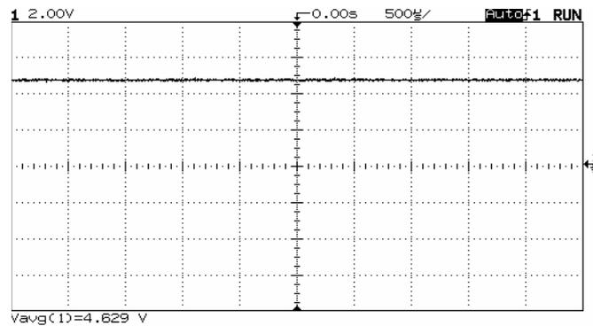
Figure 6.7: Signal when pull down resistor is used
