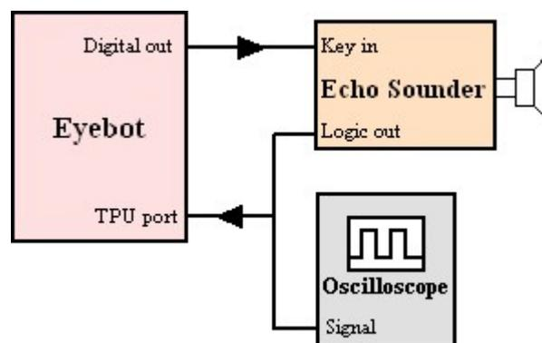
Figure 6.8: The experimental setup for the combined interface
