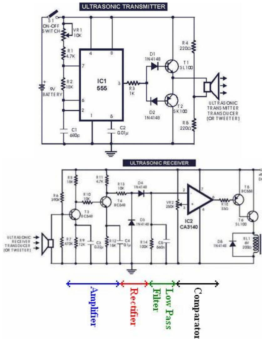
Figure 4.3: Design for an ultrasonic switch [21]
