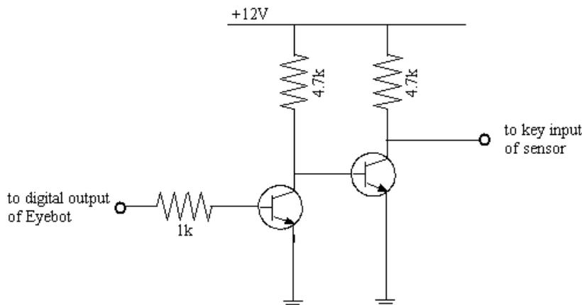
**Figure 6.13: Driver circuit to increase the voltage at the input of echo sounder**
