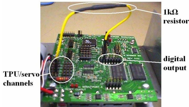
**Figure 6.1: Experimental Setup for testing the Eybot interface**
