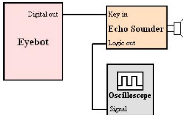
**Figure 6.3: The experimental setup for the echo sounder interface**
