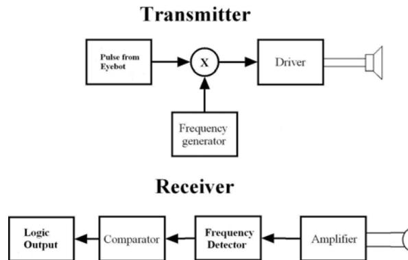
**Figure 2.3: Echo sounder operation flow chart**
