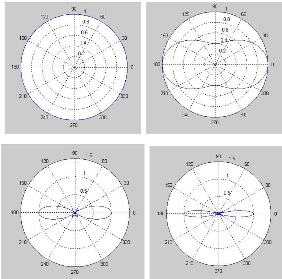
**Figures 2.6 a), b), c) & d): Directivity for transducers of frequencies 5Hz, 40 kHz, 100 KHz and 200 kHz, respectively**
