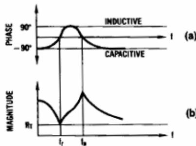
**Figure 2.4: The resonant and anti-resonant frequency of a transducer [14]**
