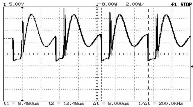
**Figure 6.17: Frequency of LM1812 output**
