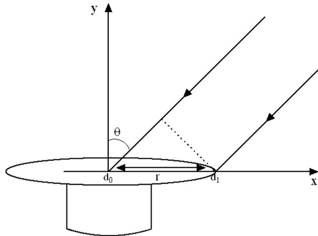
**Figure 2.5: Sound waves being received by a transducer**
