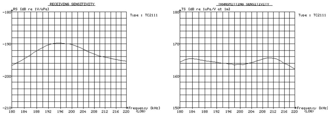
**Figures 4.2 a) & b): Receiver and transmitter sensitivities of a single transducer [19]**
