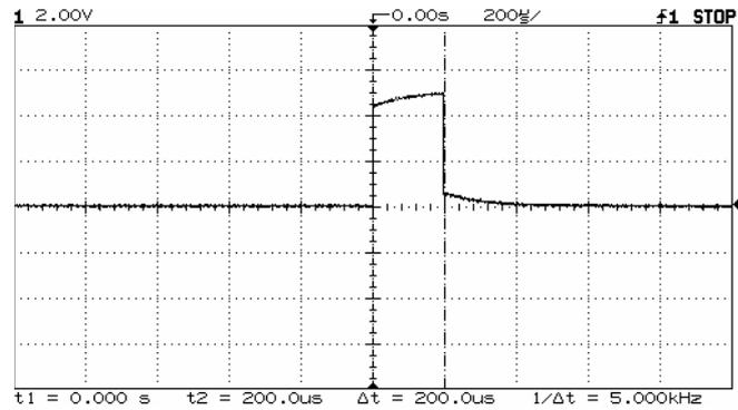
**Figure 5.1: the 200µs pulse sent from the digital output of the Eyebot**
