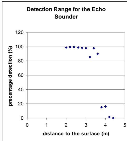
**Figure 6.12: Detection of an echo for different distances**
