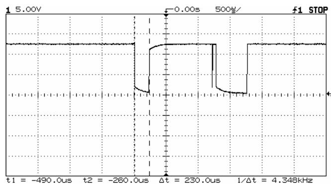
**Figure 6.5: 200µs pulse sent via the digital output, and the transducer is placed in water**
