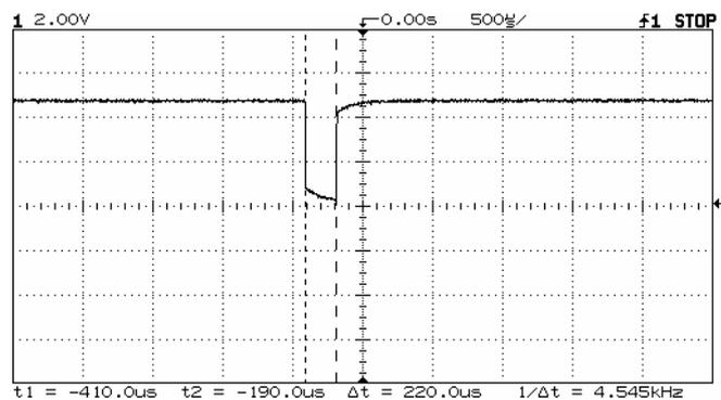
**Figure 6.9: Signal at the TPU channel when the transducer is not in the water**
