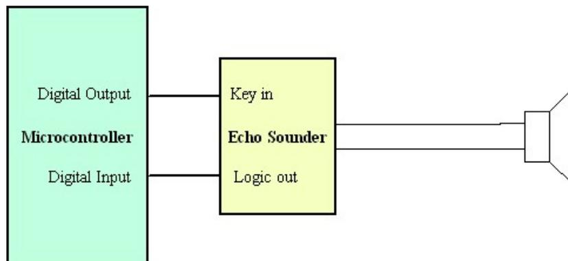
**Figure 4.6: Echo sounder communication lines with a microcontroller**
