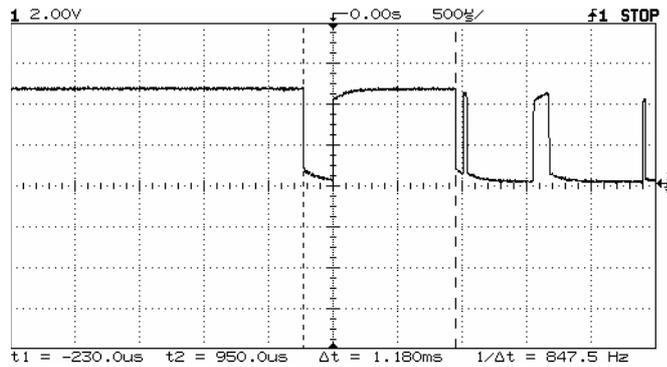
**Figure 6.10: Signal that is received at the TPU channel when the transducer is in the water**
