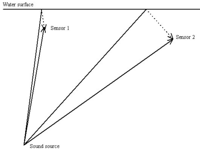
**Figure 2.1: Multipath environments cause ambiguity at the receivers**
