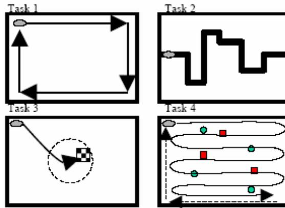
**Figure 3.1: Possible competition tasks including wall following, pipeline following, target finding and obstacle mapping [18]**
