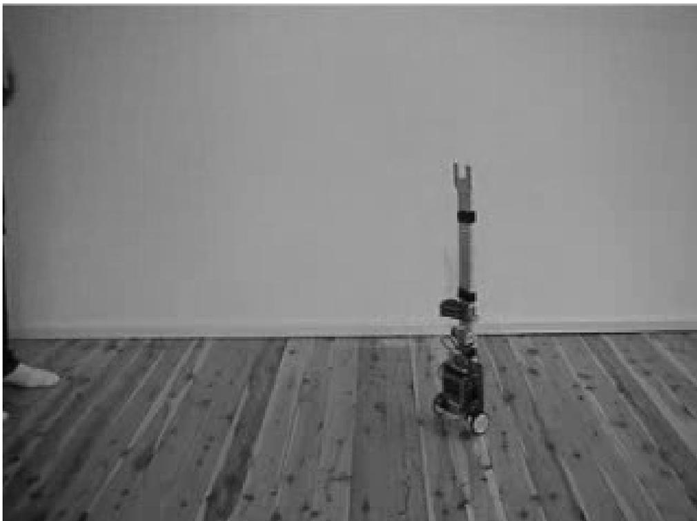
**Figure 5-27 Ballybot robot balances in the dining room, using the gyroscope for active balance and the inclinometer to perform on-line recalibration of the gyro.**
