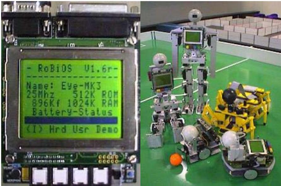
**Figure A-1** The EyeCon controller, together with a collection of some of the mobile “Eyebot” robots using the controller.
