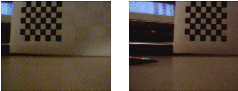
Figure 5.8: Images of an alignment test pattern, captured simultaneously from both cameras on the EyeBot M6.
