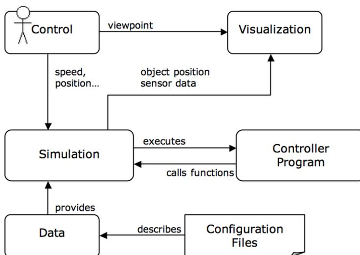
Figure 3.1: Concept of the Simulation System
