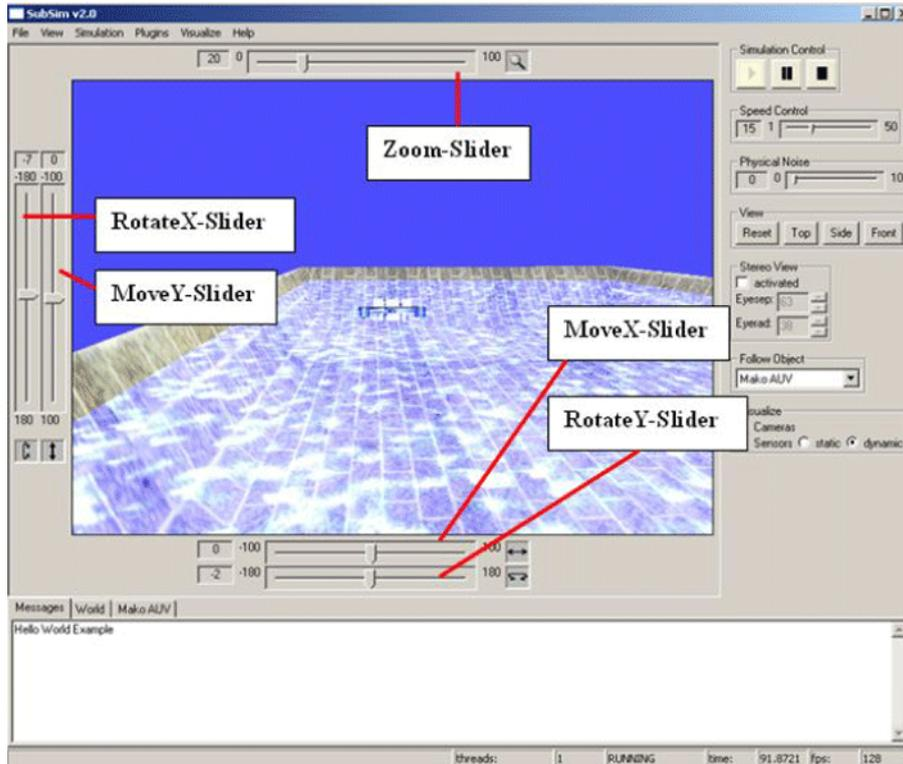
Figure 4.7: The SubSim main frame as Graphical User Interface (GUI)
