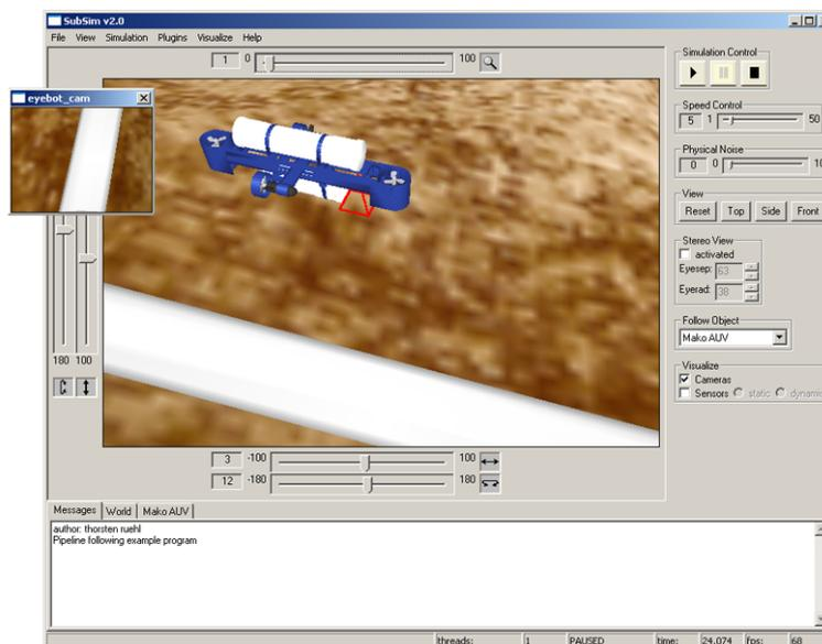
Figure 5.5: The camera frame showing the picture of a down directed camera represented as a red pyramid.
