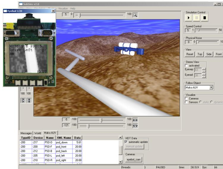
Figure 5.2: Submarine MAKO placed in the environment with the EyeBot Plugin frame loaded.
