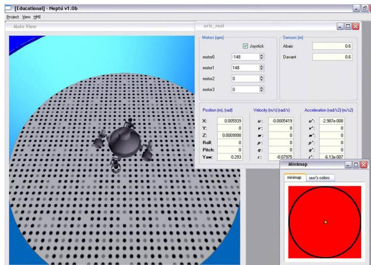
Figure 2.3: Neptune screenshot showing the graphical representation of simulation and sensor data.
