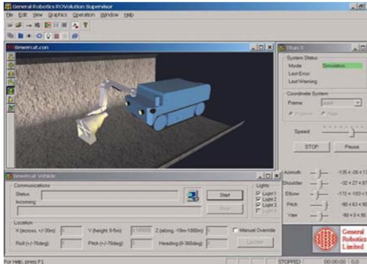
Figure 2.4: DeepWorks screenshot showing a running simulation and the control panels.
