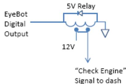
**Figure 3.9 - "Check Engine" relay**
