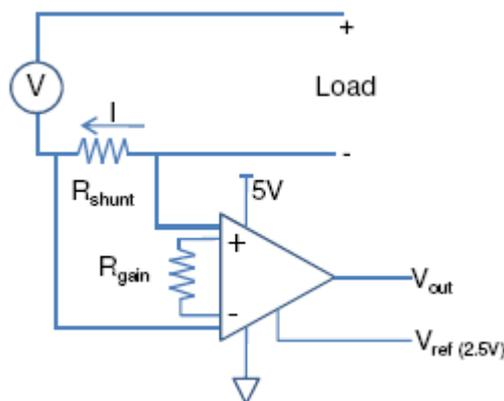
**Figure 3.4 - A current sensor**
