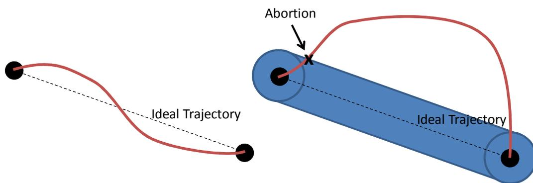
Figure 55 – Left - An individual that does not stray from the ideal trajectory. Right – an individual that exceeds the acceptable variance in trajectory and can be prematurely terminated.
