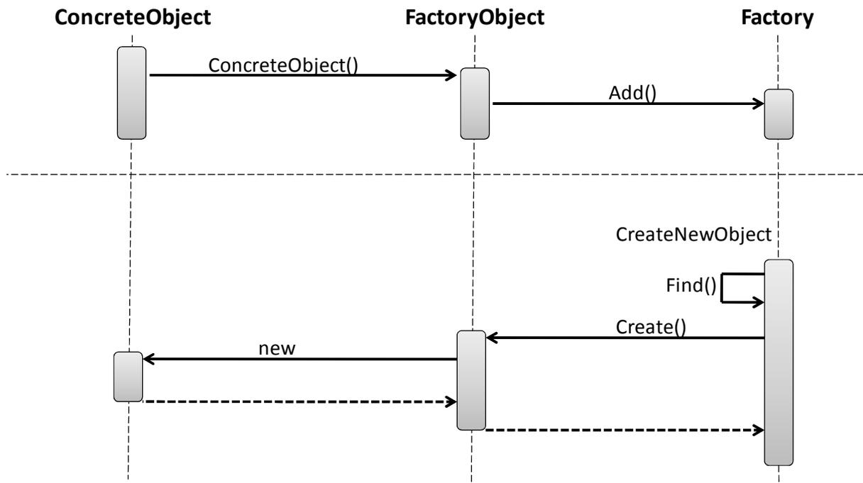
Figure 20 – Sequence diagram for a pluggable factory
