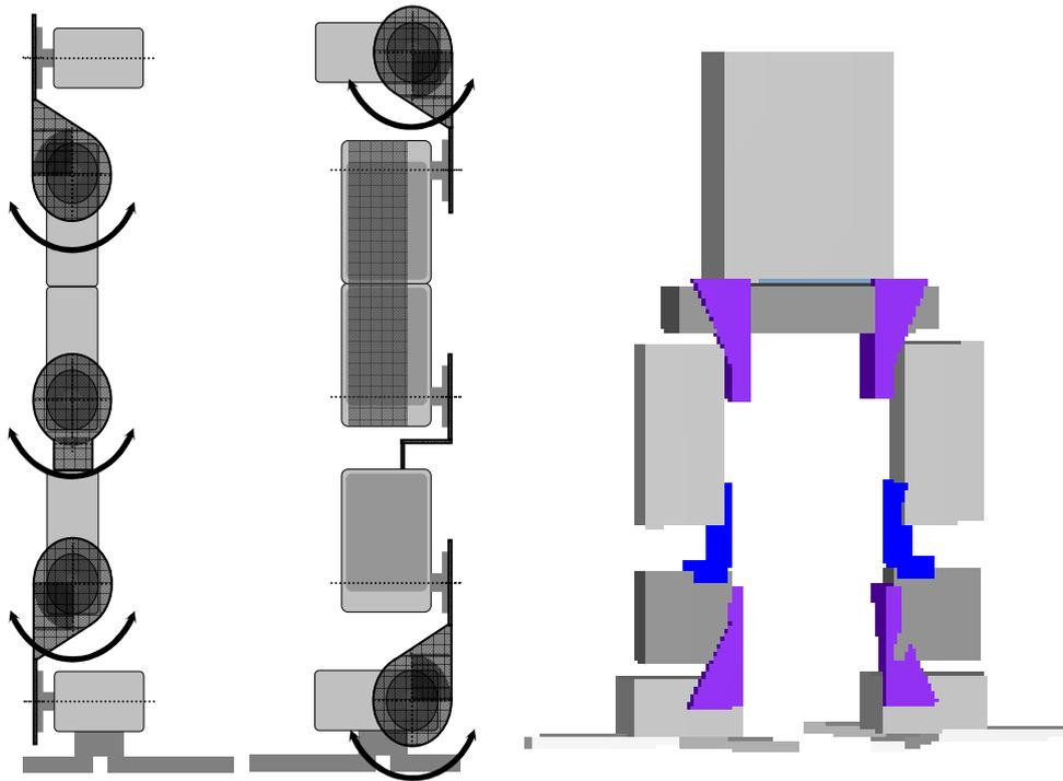
Figure 68 – Leg schematics and simulator model
