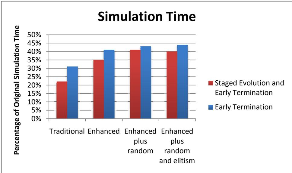
Figure 58 – Percentage of original simulation time required for GA enhancements
