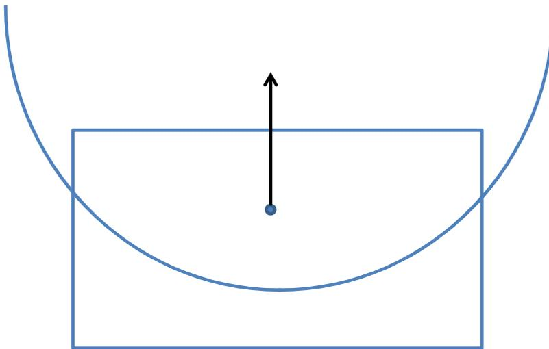
Figure 8 – Contact point and contact normal
