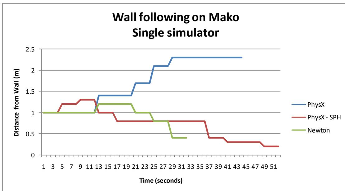
Figure 101 – Mako wall following distance readings for a single simulator evolved controller
