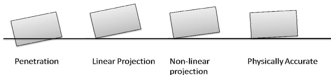
**Figure 60 – Possible collision responses. From left to right: penetration, linear projection, non-linear projection and a physically accurate result.**
