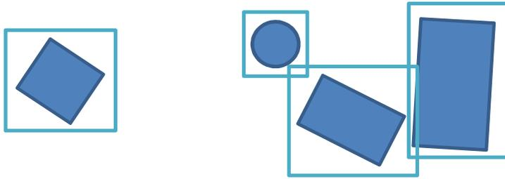
Figure 15 – Broad phase collision detection
