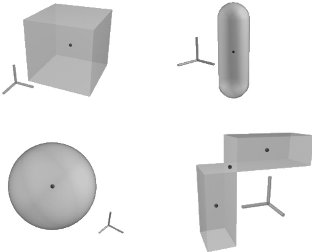
Figure 28 – PAL Dynamic Body Geometries – Top left – box, Top right – capsule, Bottom left – sphere, Bottom right – compound body
