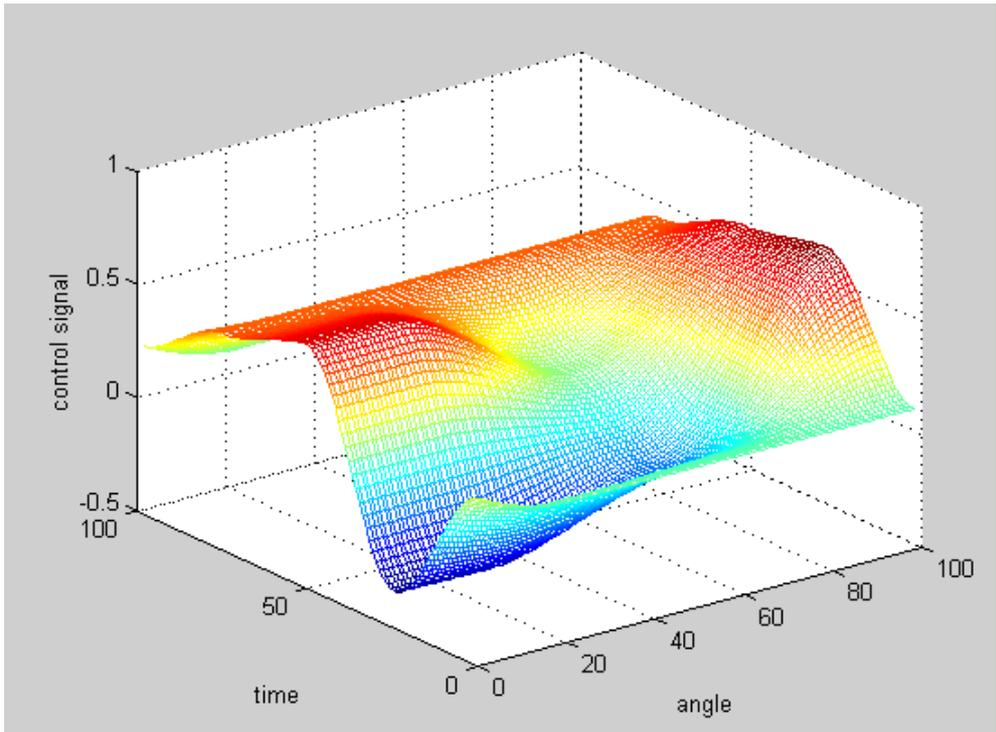
Figure 49 – Two dimensional spline controller output space
