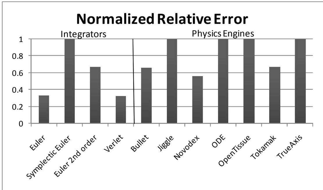
Figure 33 – Positional error from cumulative numerical integrators relative to the ideal case normalized to the Symplectic Euler integrator error
