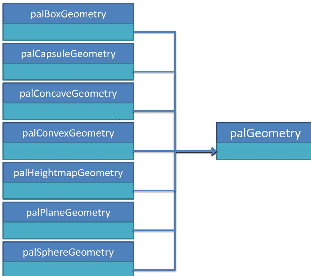
Figure 24 – PAL Geometry types
