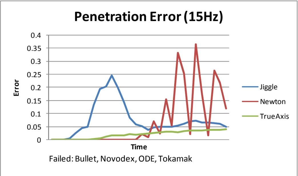
Figure 44 – Collision penetration error over time with an integrator step of 15Hz
