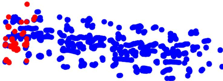
Figure 87 – Foot-ground contact points for a robot controller evolved in only one simulator (left to right). The transferred simulator foot-ground contact points are shown in red.
