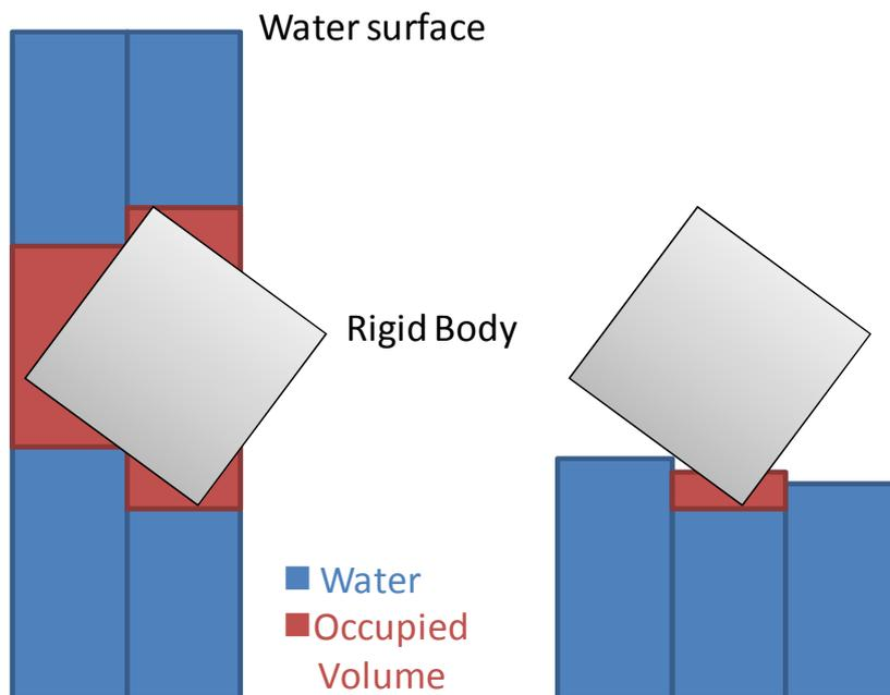
Figure 17 – Buoyancy column
