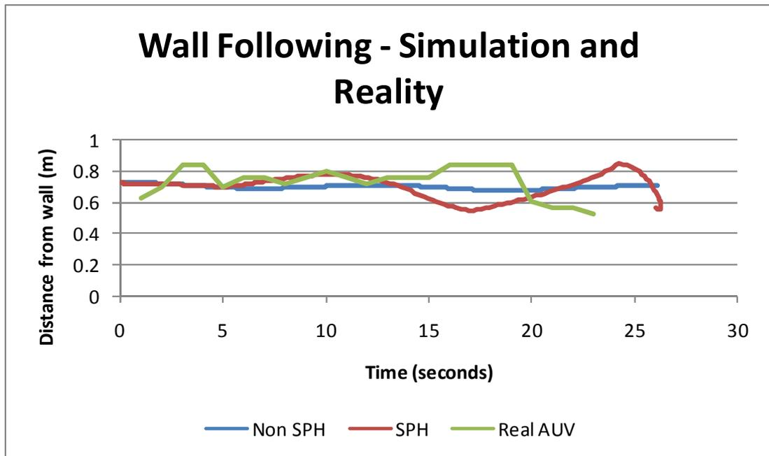
Figure 104. Comparison of distance sensor readings for the two simulation paradigms and the real AUV
