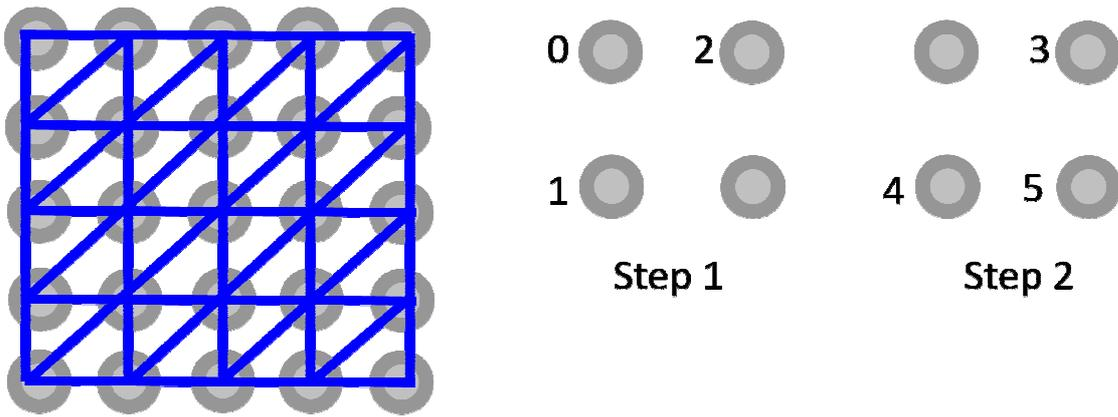
Figure 30 – Left - Triangulated height data, Right – Two step triangulation
