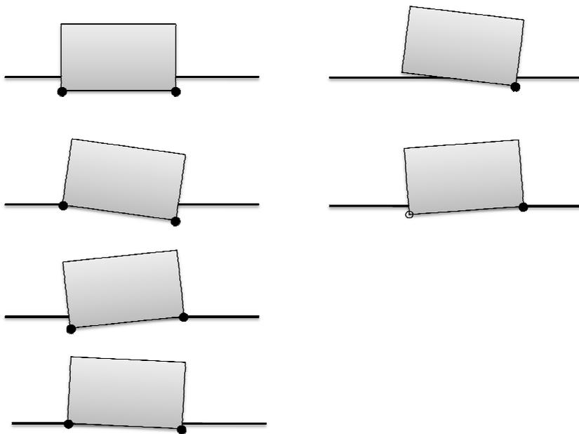
Figure 61 – Contact resolution. Left: repeating resolutions. Right: Missed contact.
