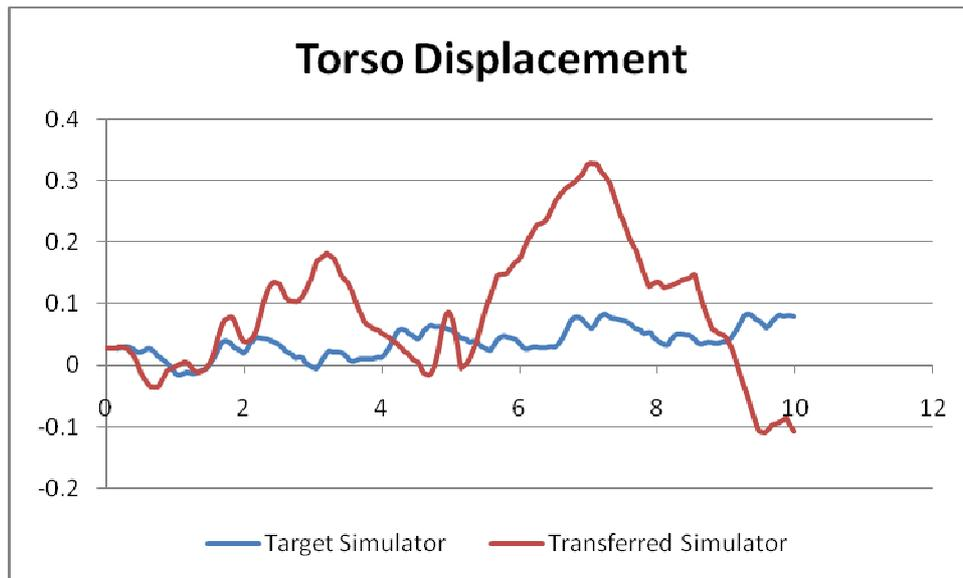
**Figure 90 – Torso displacement from the desired walking position**
