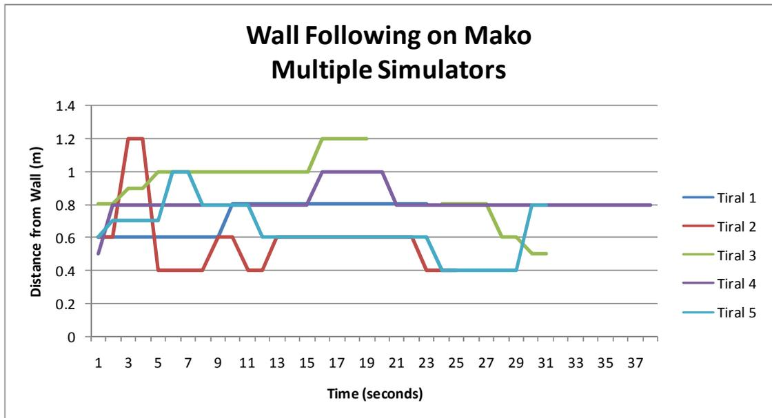
Figure 102 – Mako wall following distance readings for a multi-paradigm simulator
