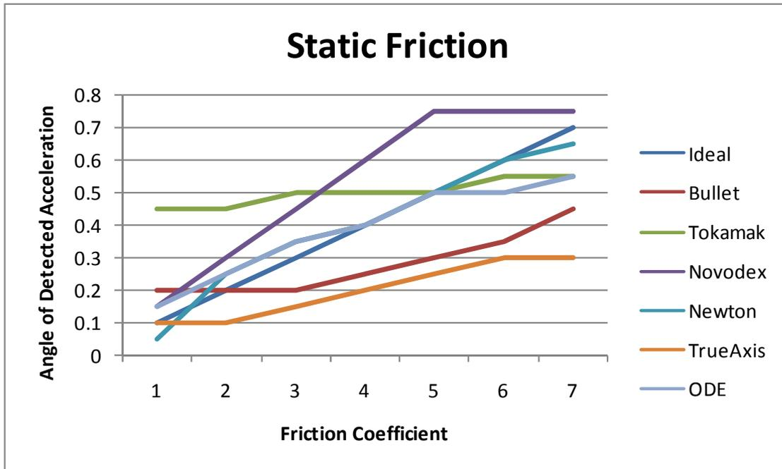
Figure 38 – Angle of the plane at which the body began movement versus the static friction coefficient
