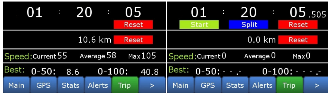
Figure 3-5 Trip information screen, running with automatic timer (left), reset with manual timer (right) The current trip information screen, Figure 3-5 , displays the current speed statistics, a resettable odometer and either a manual or automatic timer, that can be chosen in the tools screen. The current speed is simply the median GPS reading, the average speed is the long running average of the median speed calculated every second, and the maximum speed is determined by checking every second, whether or not the current speed is great than the recorded maximum speed. The fastest 0 to 50 kmh -1 and 0 to 100 kmh -1 are calculated by checking every second whether or not the speed is zero. If not, record the current time and then start checking if the speed is greater than 50 kmh -1 , or greater than 100 kmh -1 , respectively. If the speed is greater than 50 kmh -1 , use the formula defined in Equation 6 Best time calculation , in order to estimate the time when the vehicle reaches 50 kmh -1 . This is because the GPS can be polled at a maximum of once per second, hence the best time needs to be interpolated.
