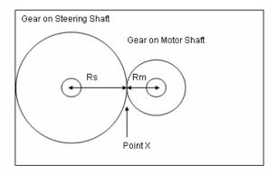
Figure 24: Steering Gear Ratio
