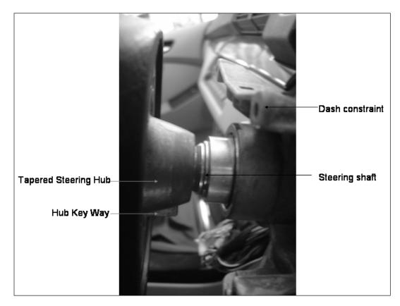
Figure 28: Steering wheel and dash constraint
