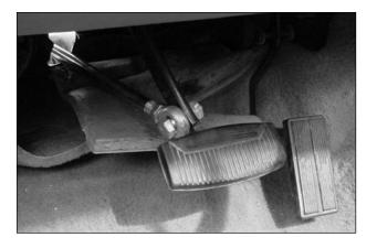
Figure 20: Brake Actuator (Golem 2006)
