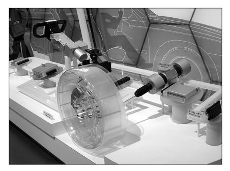
Figure 9: FHI Steer-by-wire Model (Tech-on 2005)
