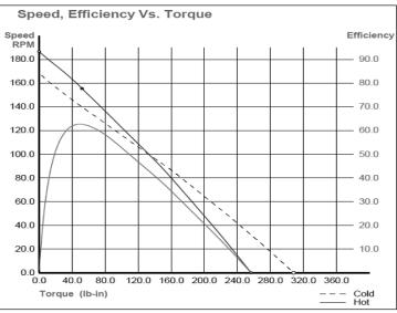
Figure 25: Speed, Efficiency, Torque Curve
