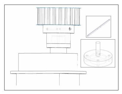
Figure 34: Steering System Shear Pin Arrangement (Inset: Shear Pin (Top), Servo Hub (Bottom))
