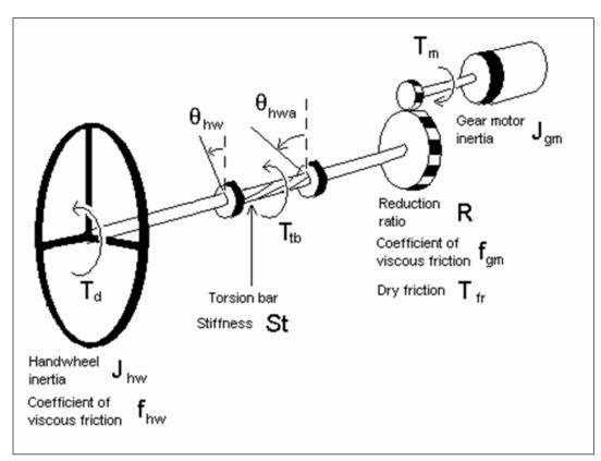
Figure 13: Steering Feedback Model (Gaulino 2006)
