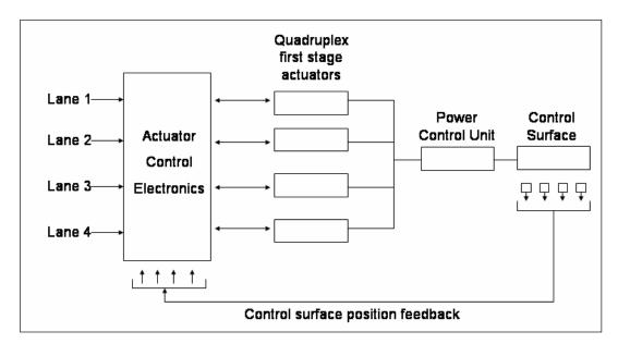
Figure 2: Quadruplex actuation system (Collinson 1999)
