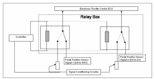
Figure 27: Throttle Control System Overview
