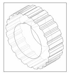
**Figure 29: Machined Timing Pulley**
