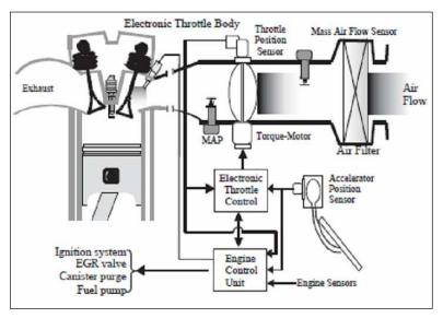
Figure 10: Electronic Throttle Control (Conaster et al. 2002)
