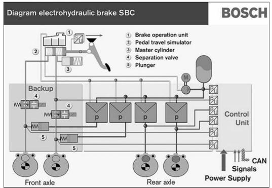
Figure 4: "Sensotronic" Brake Control (Kuhlgatz 2005)
