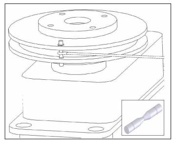
Figure 33: Braking System Shear Pin Arrangement (Inset: Shear Pin)
