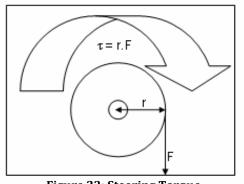
Figure 23: Steering Torque
