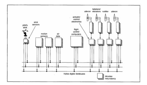
Figure 1: Flight control system bus configuration (Collinson 1999)
