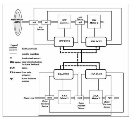
Figure 12: Steer-by-wire system architecture (Wilwert et al. 2007)
