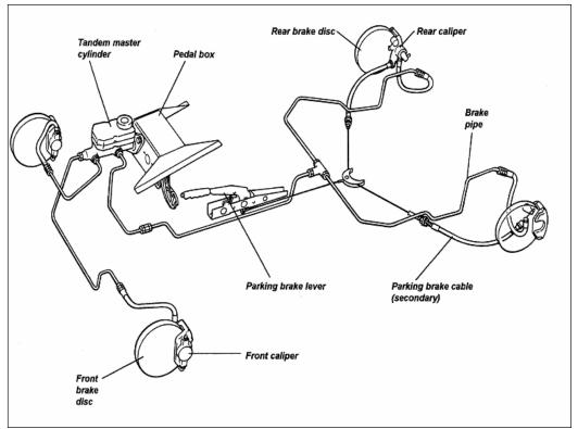
Figure 3: Lotus Elise Brake System Layout (Massey 2001)
