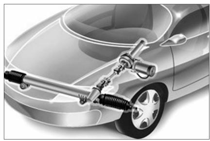
Figure 8: Electric power-assist steering (Delphi 2005)
