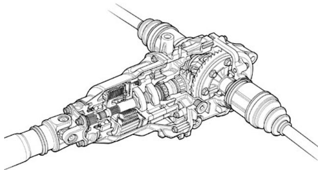
**Figure 5: Internal View of Differential**
