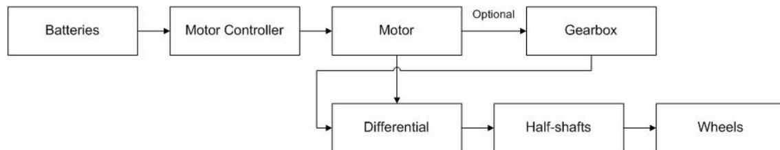
**Figure 3: Power Transfer in Proposed Drivetrain**
