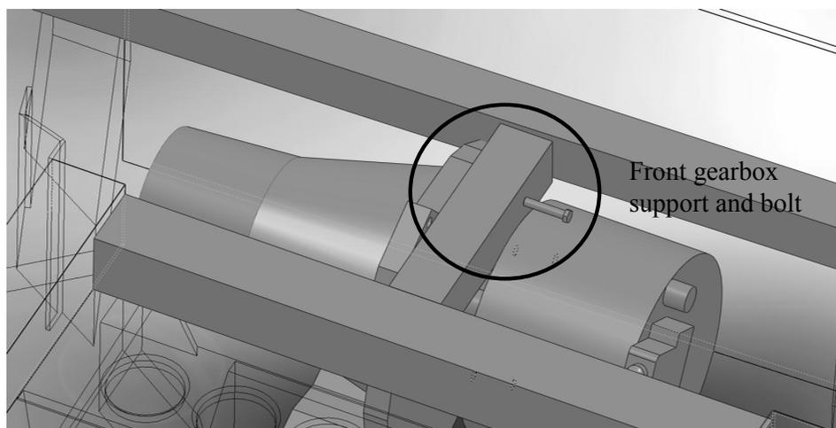
**Figure 19: Front Gearbox Support and Frame**
