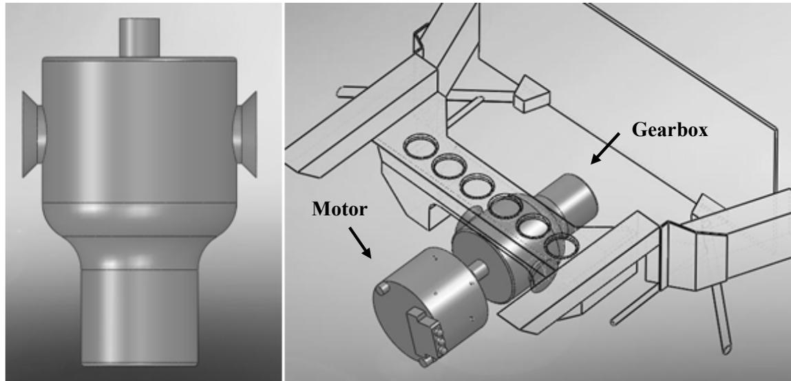
**Figure 12: Rear-engine Gearbox (sketch) and Possible Drivetrain Design**
