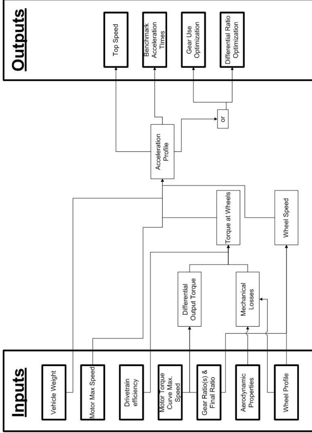
Figure 9: Computational method of Frans Ho's performance model.
