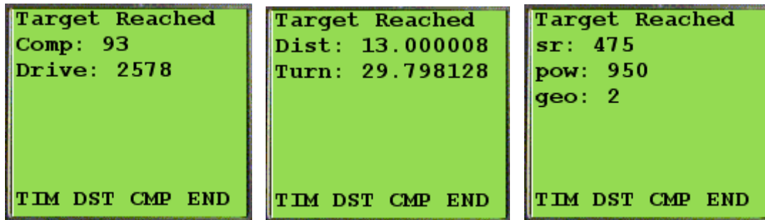
Figure A-3 (a) Left. Computation and driving times. (b) Centre. Total distance traveled and total rotation performed. (c) Right. Calls to the maths library or process-state() in D*.
