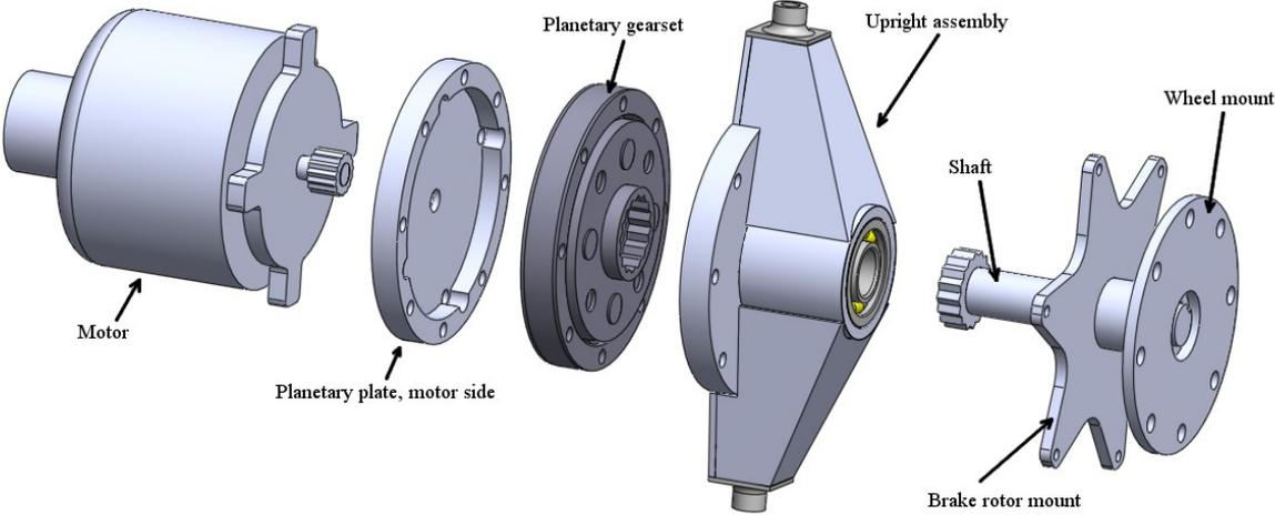
*Illustration 42: Final assembly exploded view*
