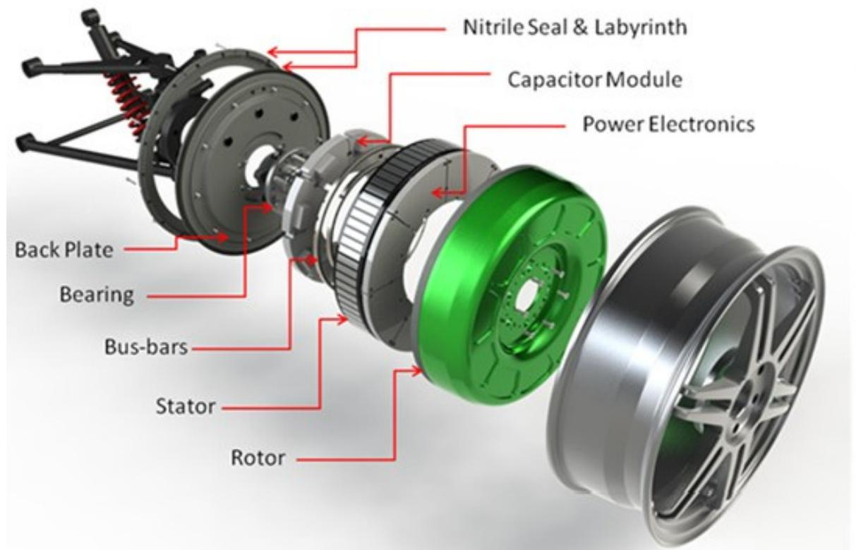
*Illustration 5: Hi-Pa Drive in wheel motor concept*
