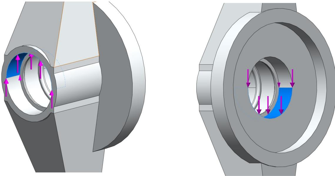
*Illustration 30: Forces on upright due to maximum wheel loading*
