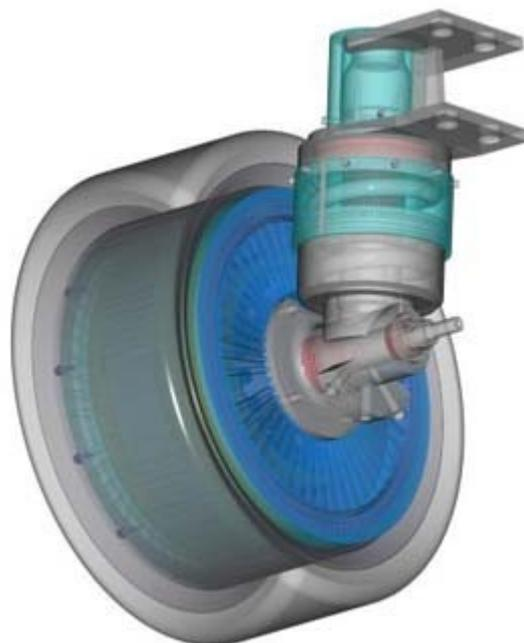
*Illustration 3: e-Traction in Wheel motor*
