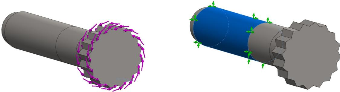
*Illustration 41: Forces and restraints on shaft during torsion*
