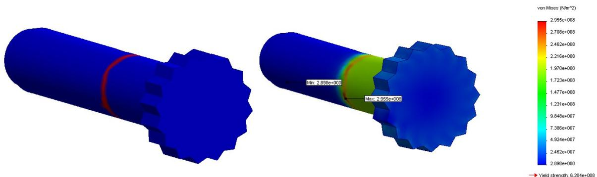
Illustration 40: Shaft safety factor (red shows below 3) and Von Mises stress distribution
