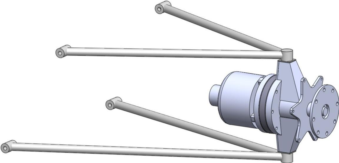
*Illustration 43: Final assembly incorporated into suspension*
