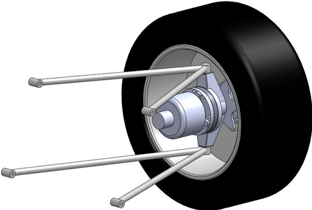
*Illustration 44: Final assembly shown with suspension and wheel*
