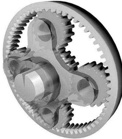
*Illustration 21: Planetary gear-set (Diesel Power. 2009)*
