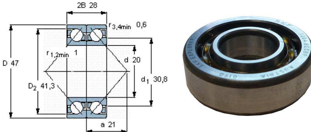
*Illustration 23: SKF Angular contact ball bearing for paired mounting, 7204BECBM*
