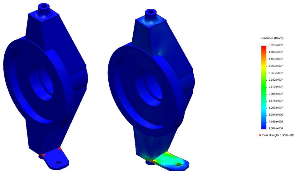
*Illustration 32: Steering mount safety factor (red shows below 6) and Von Mises stress distribution*
