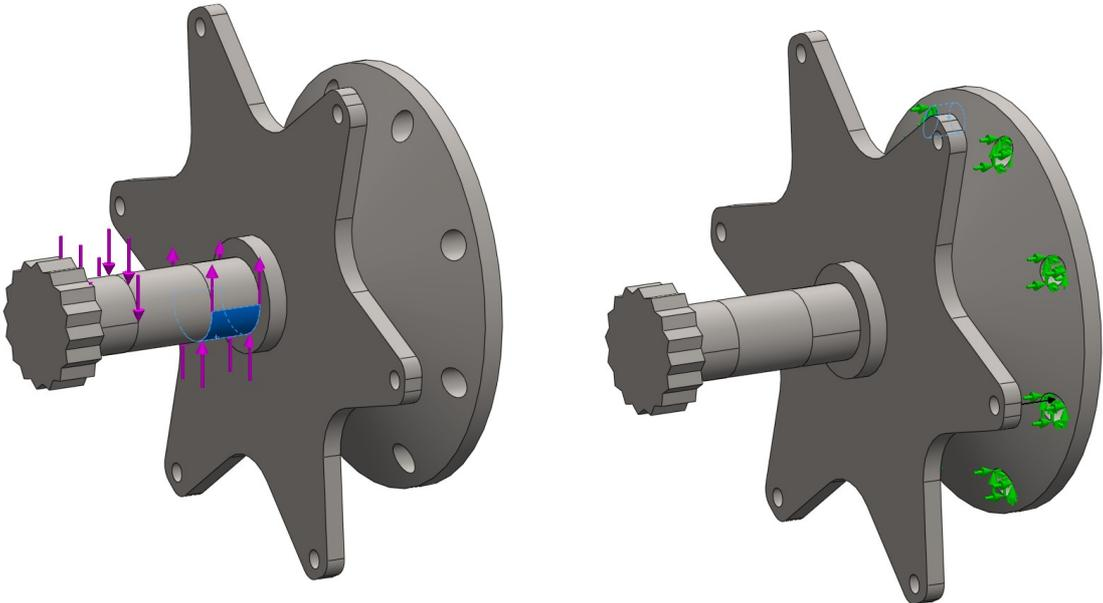
Illustration 37: Forces and restraints on drive-shaft during bending
