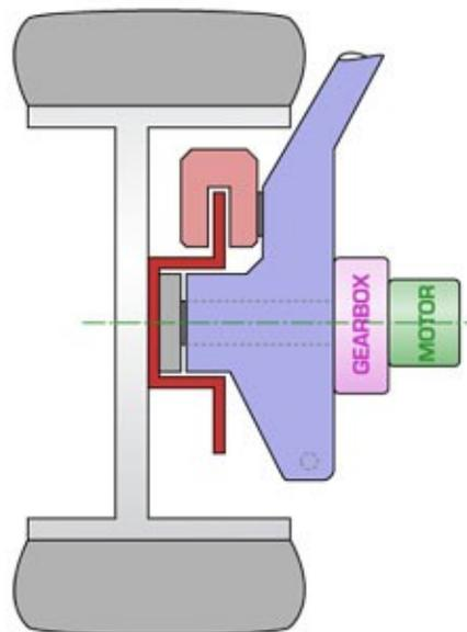
*Illustration 11: Example of a wheel mounted motor (Hooper I 2010)*
