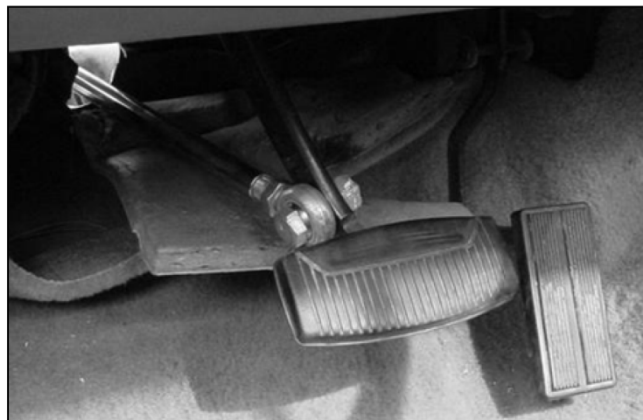
Figure 3: Linear Brake Actuator through Firewall (Golem 2006)
