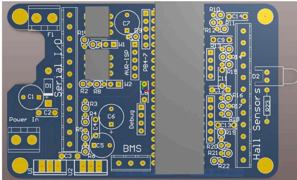
Figure 39 PCB 3D Model (Top Layer)
