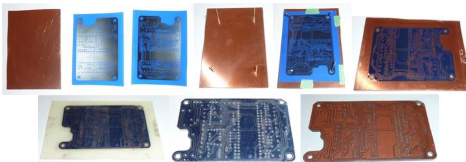
Figure 42 PCB Double Sided Manufacture
