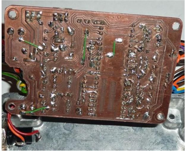
Figure 33 Home Made PCB Prone to Short/Open Circuit, Under/Over Etching
