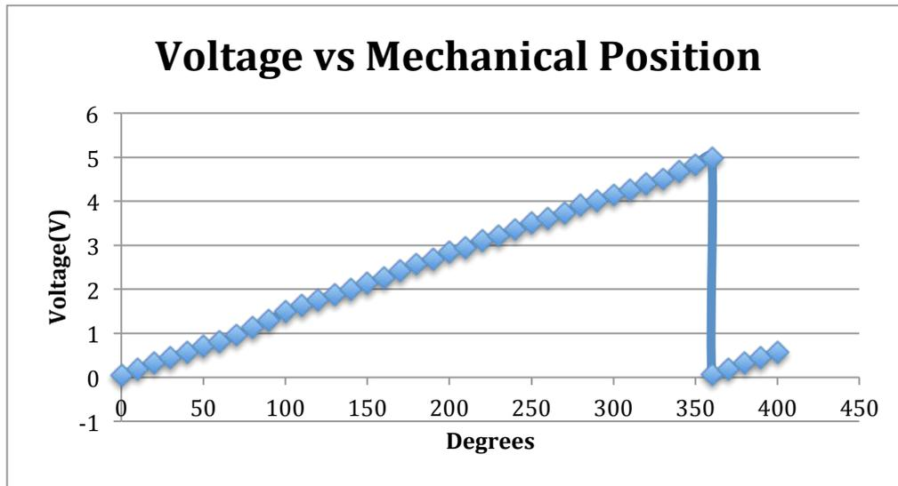
Figure 23 Shaft Encoder Angular Position vs Voltage
