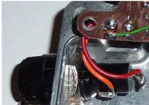
**Figure 9 Externally Accessible M205 Fuse Holder**
