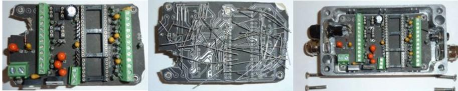
Figure 41 PCB Cardboard Prototyping
