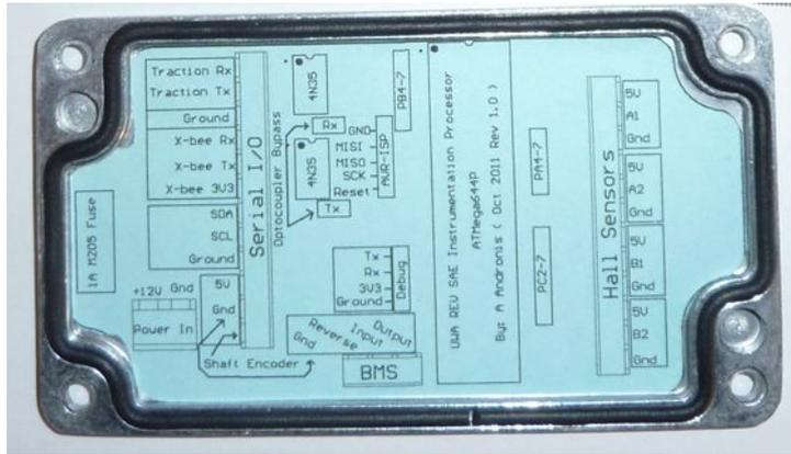
**Figure 13 Diecast Box Hermetic Rubber Seal**
