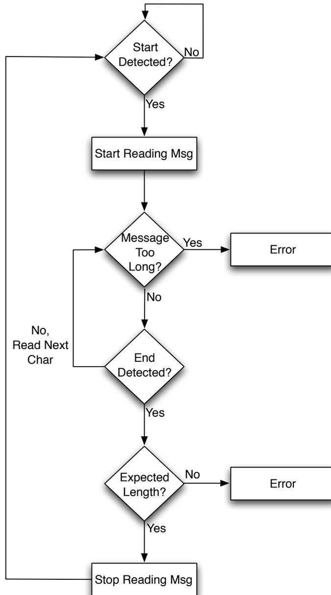
**Figure 32 Receive Sensor Data Flow Chard**
