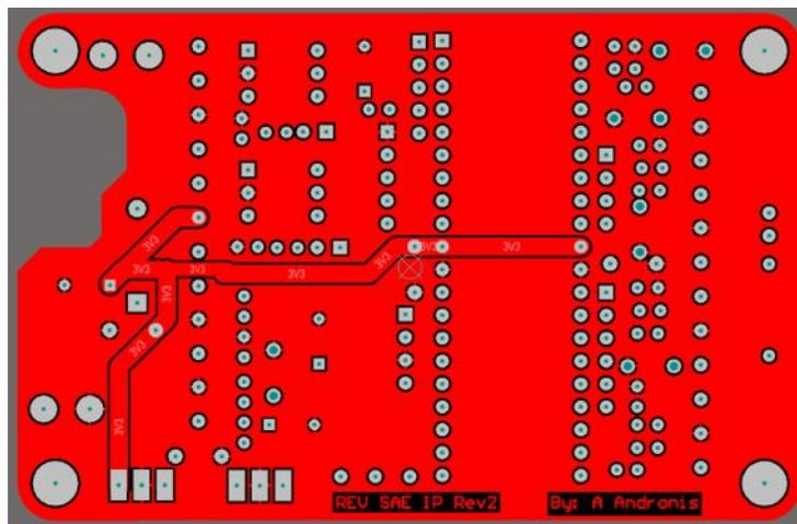
**Figure 10 PCB Top Layer (Ground Plane)**
