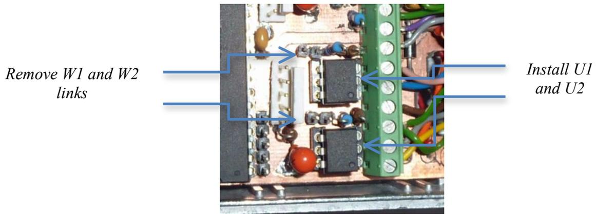
Figure 26 Opto Couplers Installed
