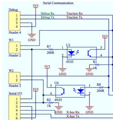
Figure 24 Traction Serial Link Opto Isolators
