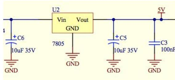
Figure 7 Linear Regulator Power Supply Filtering
