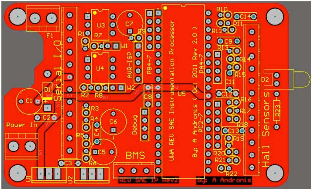
Figure 37 PCB Design (Top Overlay and Top Layer)
