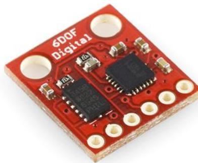
Figure 21 IMU 6DOF Digital Combo [12]
