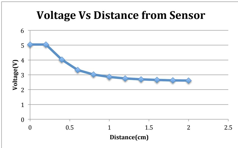
Figure 16 Hall Sensor Linearity Test – Case 1
