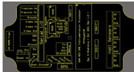
Figure 8 External Wiring Diagram (Attached to lid)
