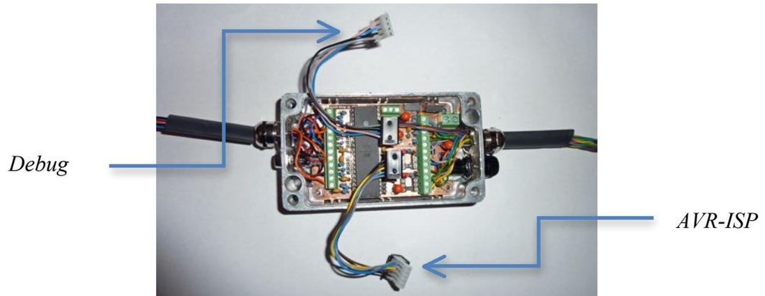
Figure 36 Internal Wiring (Program and Debug Adaptors)
