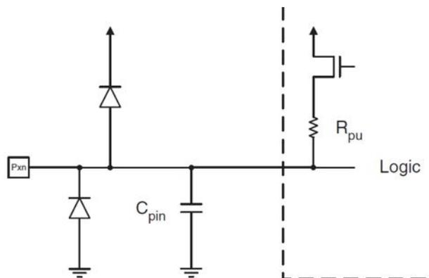
Figure 4 AVR Micro Controller I/O Diode Protection [8]
