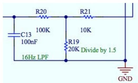
Figure 6 16Hz Low Pass Filter
