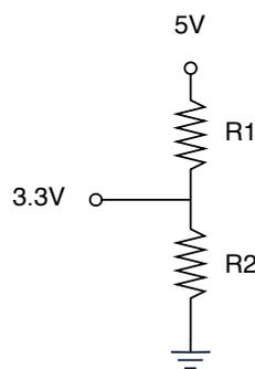
**Figure 5 5V to 3.3V Attenuator**
