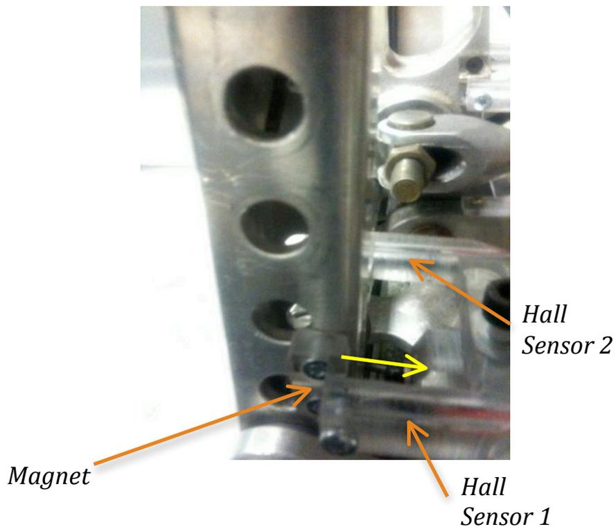
**Figure 19 Magnet and Dual Hall Sensor Mounting**
