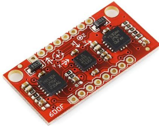
**Figure 20 Analog Gyro/Accelerometer IMU**
