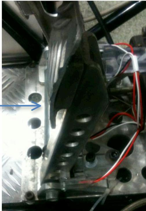
**Figure 18 Hall Sensor Pedal Mounting**
