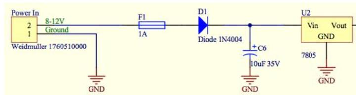
Figure 3 Input Power Protection Circuit
