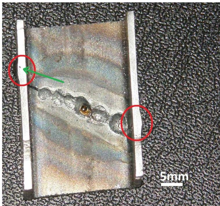
**Figure 47** Weld sample, butt weld of square tube. Small defect indicated with green arrow
