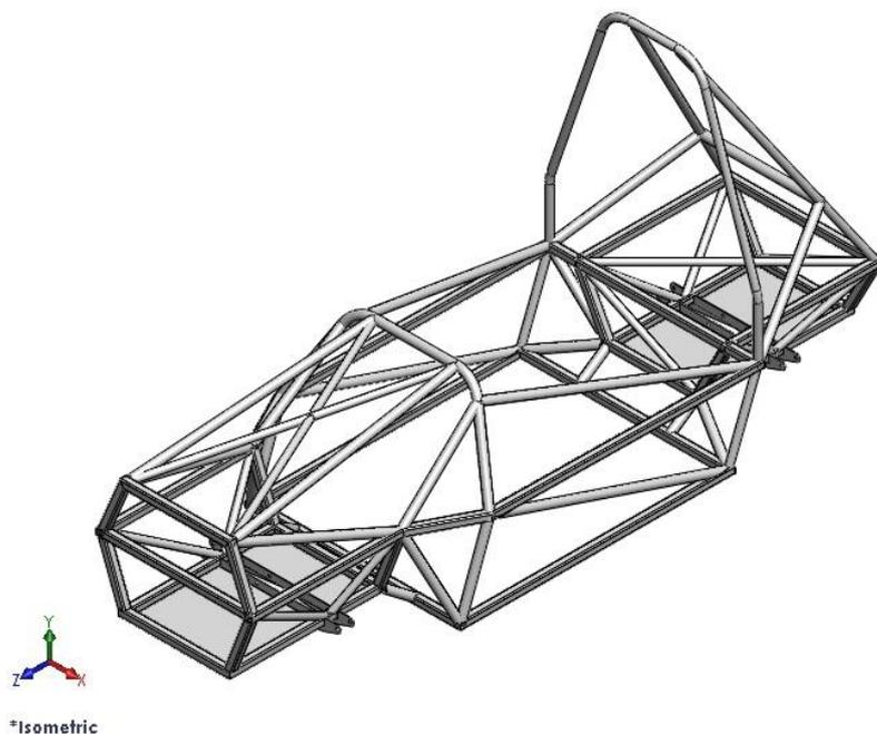
**Figure 42 Completed Space-frame**
