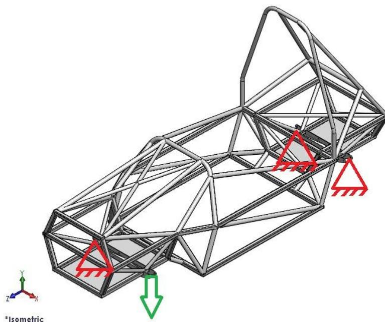
**Figure 45 Torsion test procedure for competed chassis**
