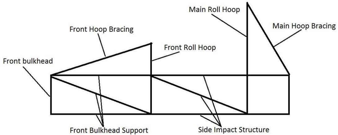
**Figure 2. Pictorial representation of the members required by the FSAE rules.**
