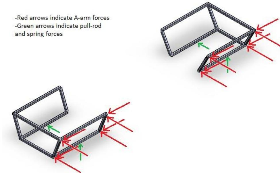
**Figure 7 Basic ends of the chassis that hold the suspension arms in place.**
