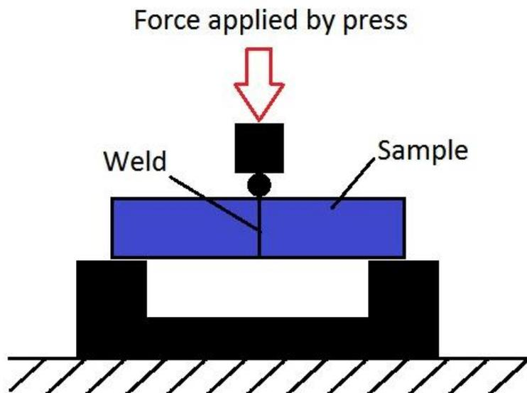
Figure 50 Schematic Diagram of 3 point bend test
