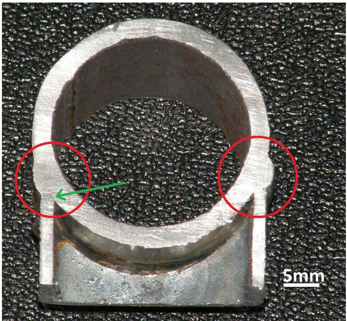
**Figure 48** Weld sample square tube welded to roll hoop tubing. Incomplete fusion indicated with green arrow
