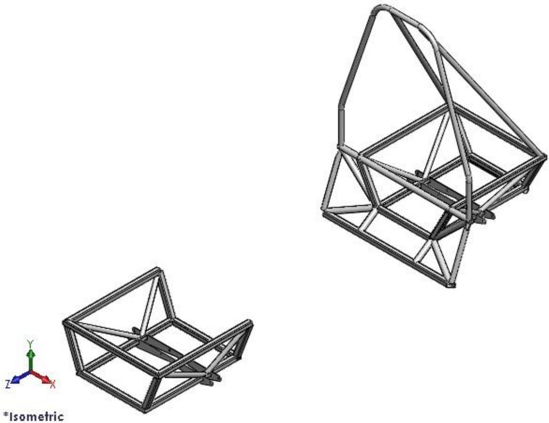
**Figure 30 Front and Rear sections with main roll hoop and roll hoop supports added**
