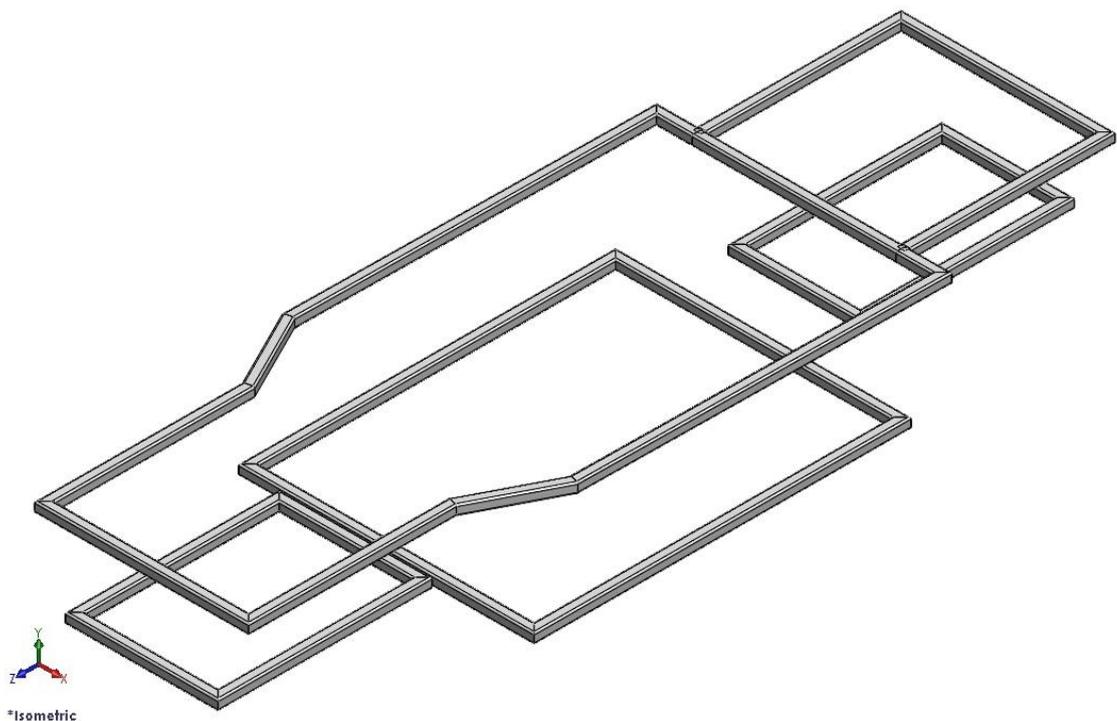
**Figure 38 Horizontal Planar sections are welded first**
