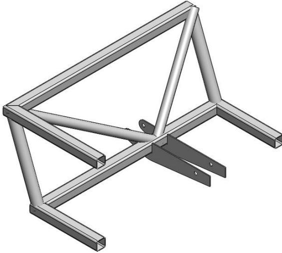
**Figure 26** 3mm Laser cut plate steel sections to mount spring and rocker
