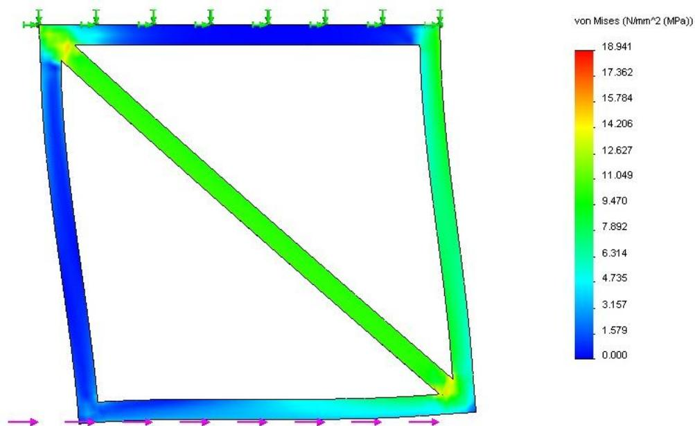
Figure 13 Von-Mises Stress contour for SolidWorks model of a triangulated square frame
