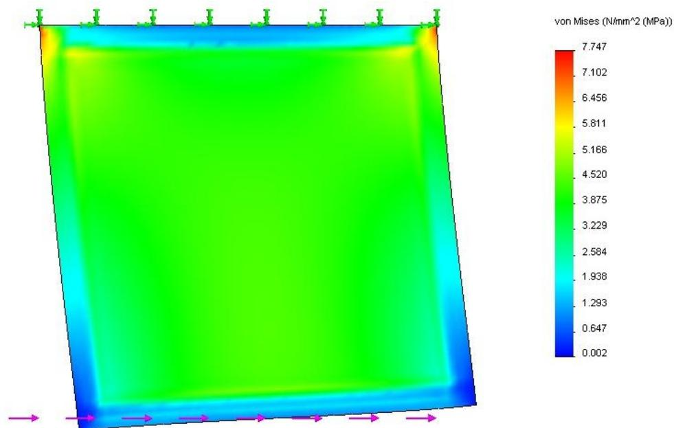
**Figure 15 Von-Mises Stress contour for SolidWorks model of a square frame with stressed skin reinforcement**
