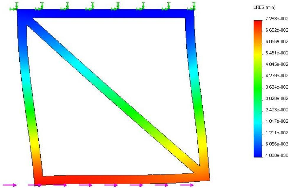
Figure 12 Displacement contour for SolidWorks model of a triangulated square frame
