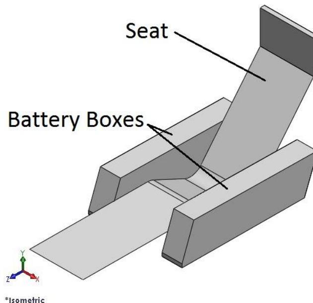
**Figure 17 Stressed battery boxes and seat used to stiffen cockpit section of chassis**
