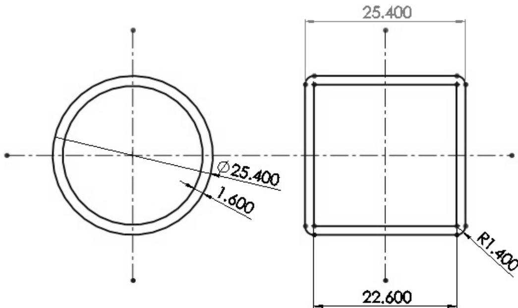
**Figure 8 Dimensions of the square and round tubing used**
