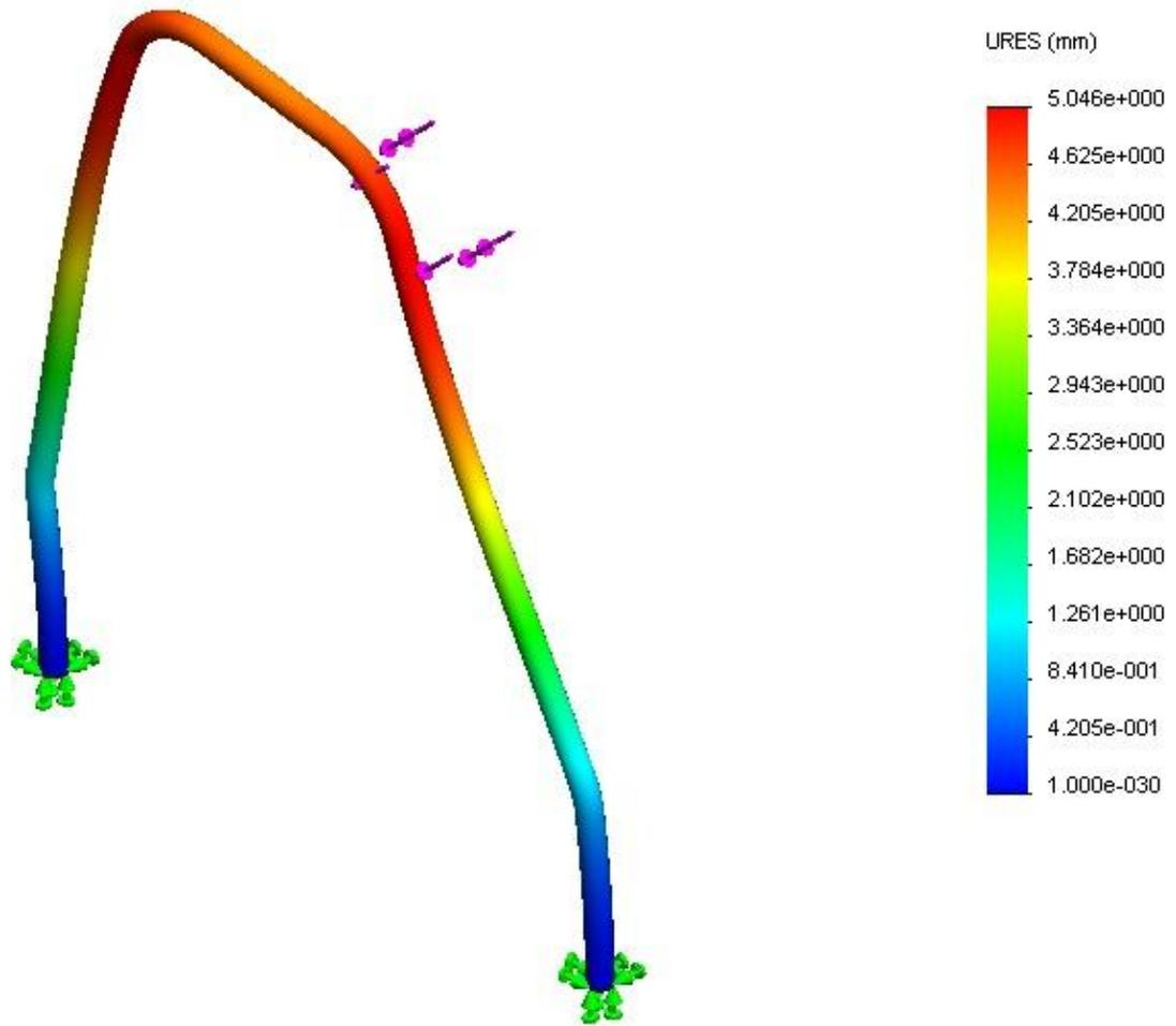
**Figure 31 SolidWorks simulation of roll hoop in roll over situation**
