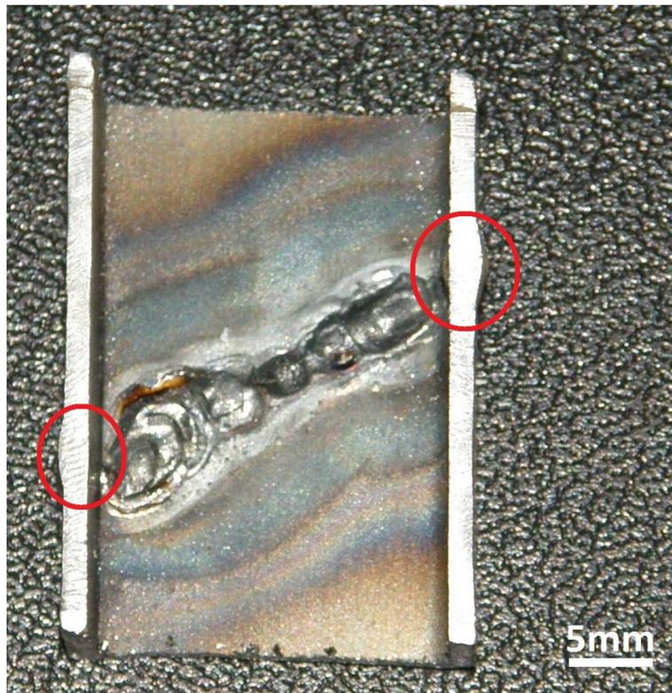
**Figure 46** Weld sample, butt weld of square tube
