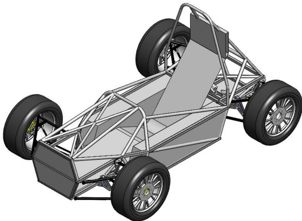
**Figure 36 Complete chassis with suspension**
