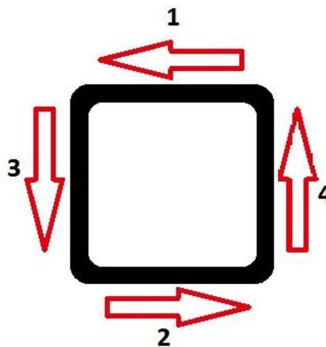
**Figure 37 Order and direction welds should be made around a square tube joint**
