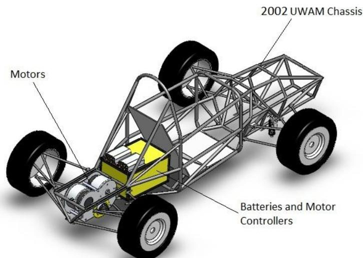
**Figure 1 2001 UWAM Chassis converted to electric power using a conventional inboard engine layout**
