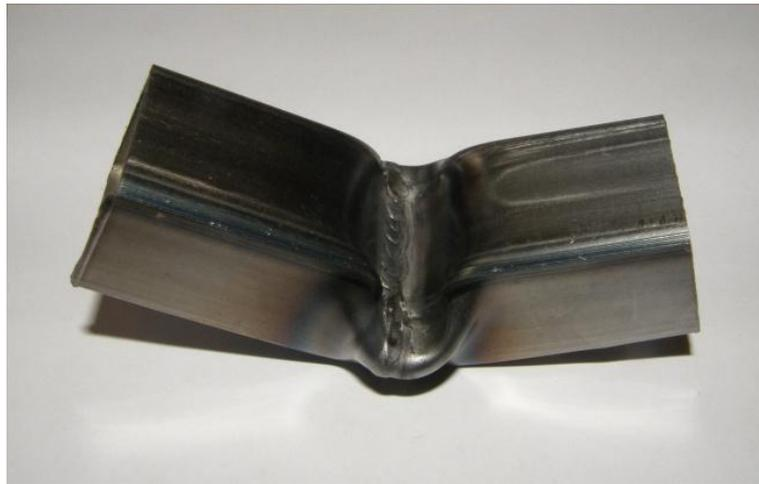
**Figure 51 Three Point Bend weld sample**
