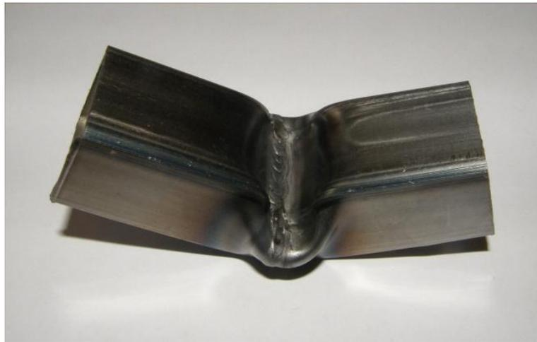
**Figure 51 Three Point Bend weld sample**
