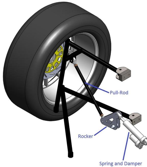
**Figure 23 Front-Right suspension assembly as designed by Marcin Kiszko (Kiszko, 2011)**
