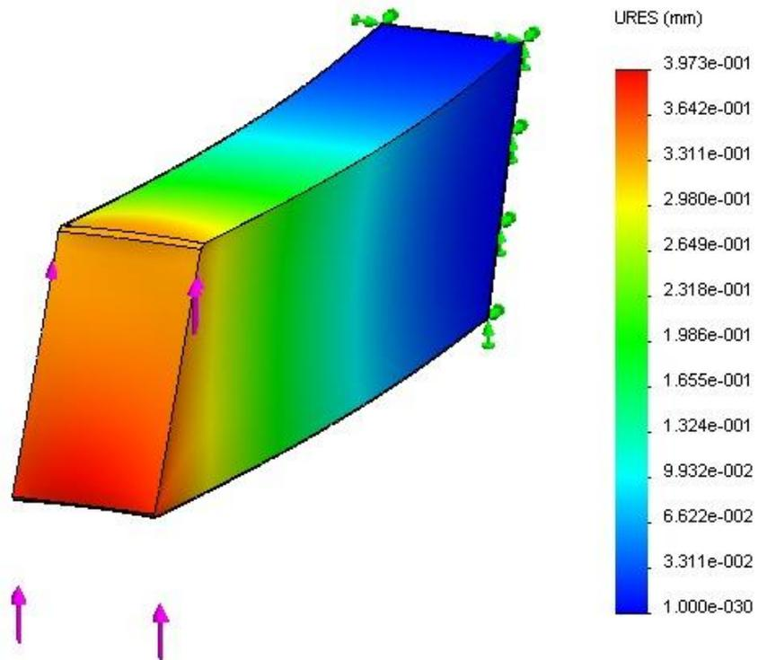
**Figure 19 SolidWorks model of a single battery box in bending**
