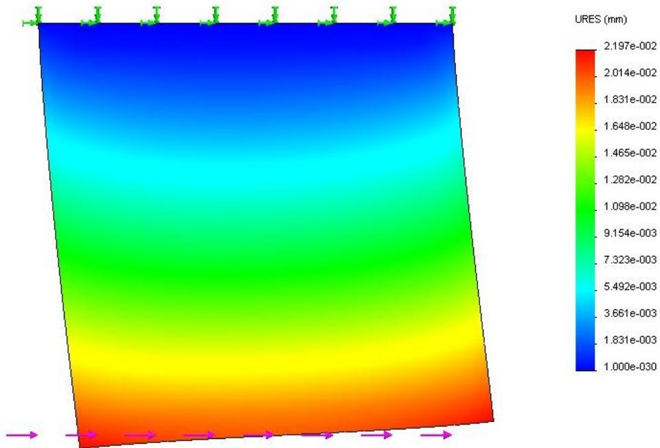
**Figure 14 Displacement contour for SolidWorks model of a square frame with stressed skin reinforcement**
