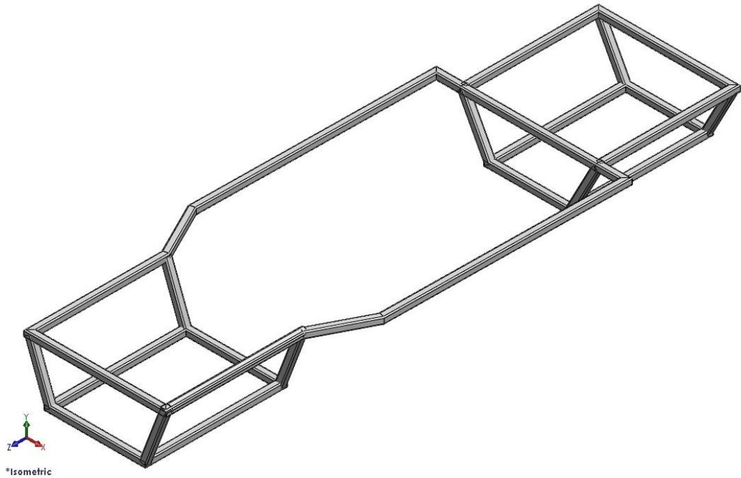
**Figure 39 Front and rear lower sections attached to main horizontal section**
