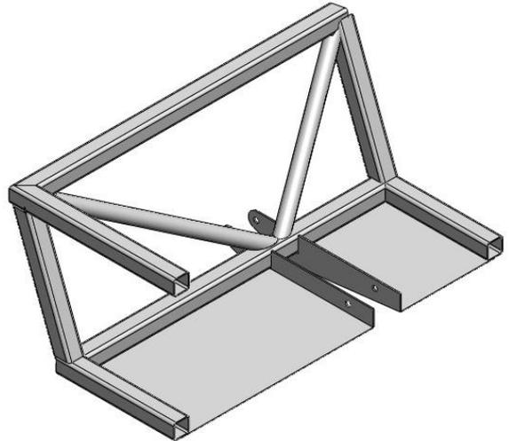
**Figure 27** Stressed skin floor added to triangulate section and support the spring mount against buckling
