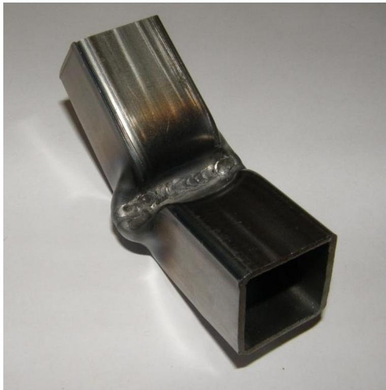
**Figure 52 Three Point Bend weld sample**
