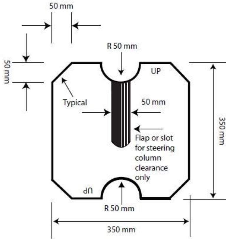
**Figure 5 Foot-well clearance template**
