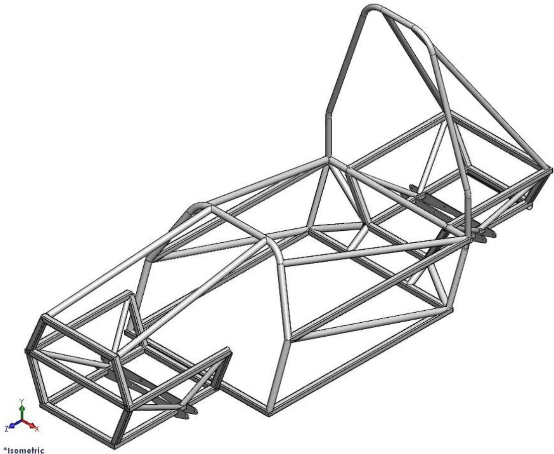
**Figure 33 Front Bulkhead and forward front roll hoop supports**
