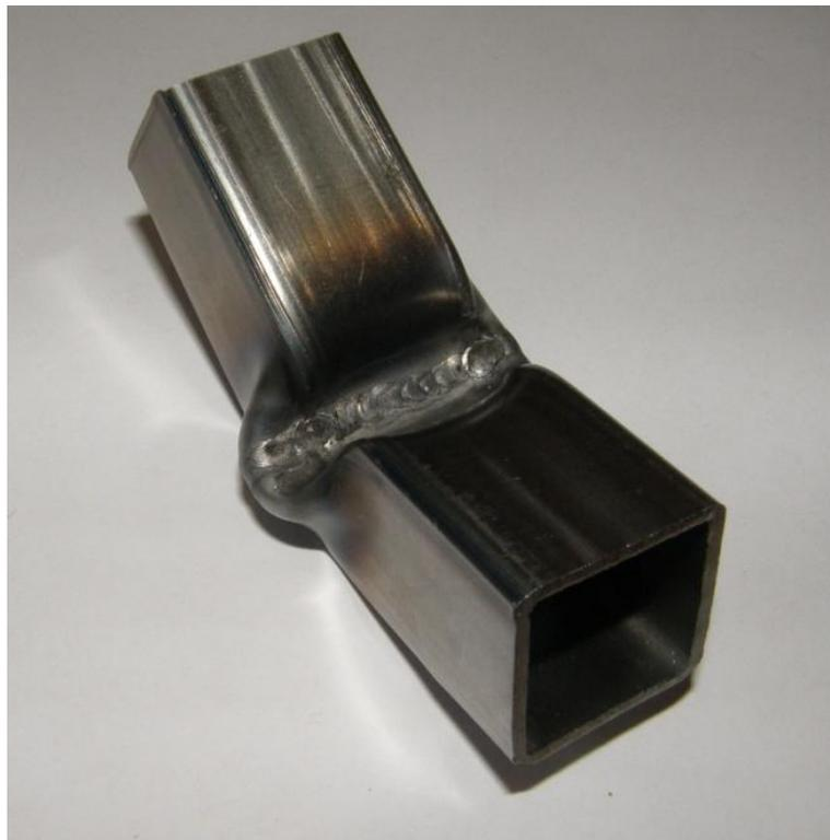
**Figure 52 Three Point Bend weld sample**
