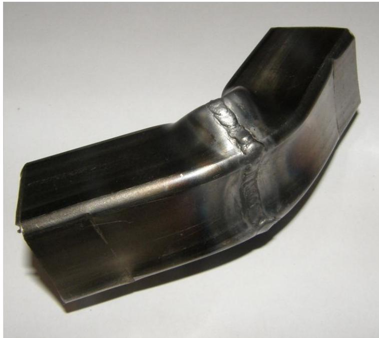
**Figure 53 Three Point Bend weld sample**
