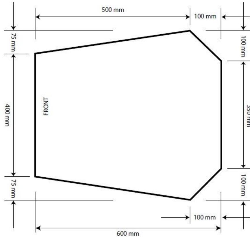
**Figure 4 Cockpit entry template**
