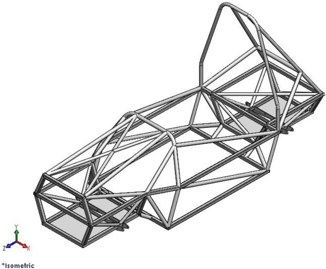
**Figure 34 Completed space-frame**
