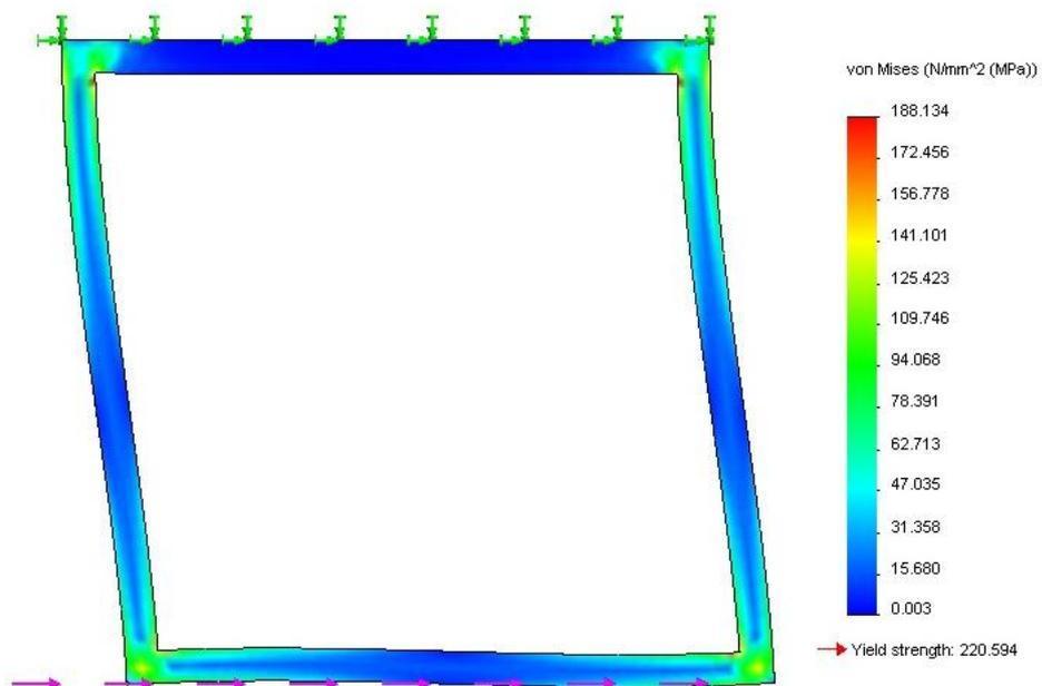
Figure 11 Von-Mises stress contour for SolidWorks model of an un-triangulated square frame
