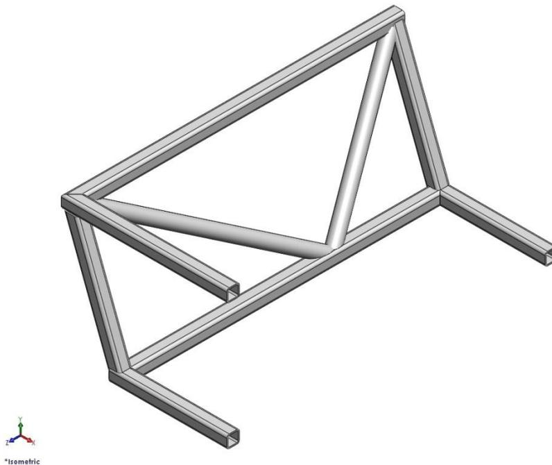
**Figure 25 Front-Right chassis section with Triangulation used to support Y component of suspension force**
