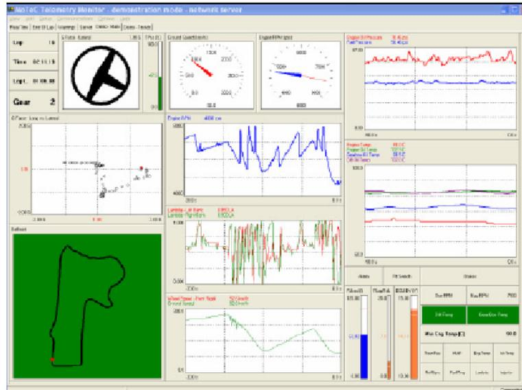
Figure 2.1: MoteC i2 Telemetry Software GUI Overview
