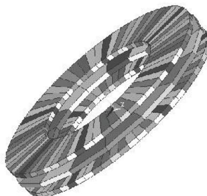
*Figure 5.8: 3D view of three-disc magnet layout
