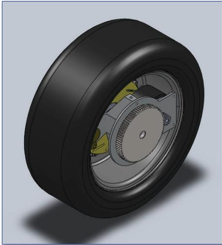
*Figure 9.9: Preliminary hub design in SolidWorks*
