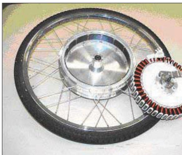
*Figure 5.19: Typical example of direct drive bicycle hub motor (Copied from Brand, Ertugrul & Soong 2003)*
