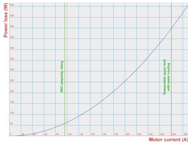
*Figure 7.7: Graph of resistive power loss vs motor current*
