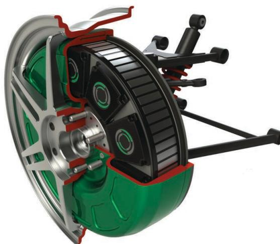
*Figure 5.36: Cutaway view of Protean Electric's electric wheel motor (Copied from Brooke 2010)*
