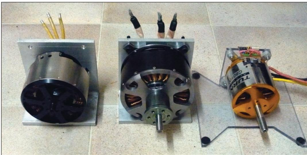
Figure 8.1: From left to right: Plettenberg Predator 37, Turnigy CA120-70, Turnigy CA80100-130
