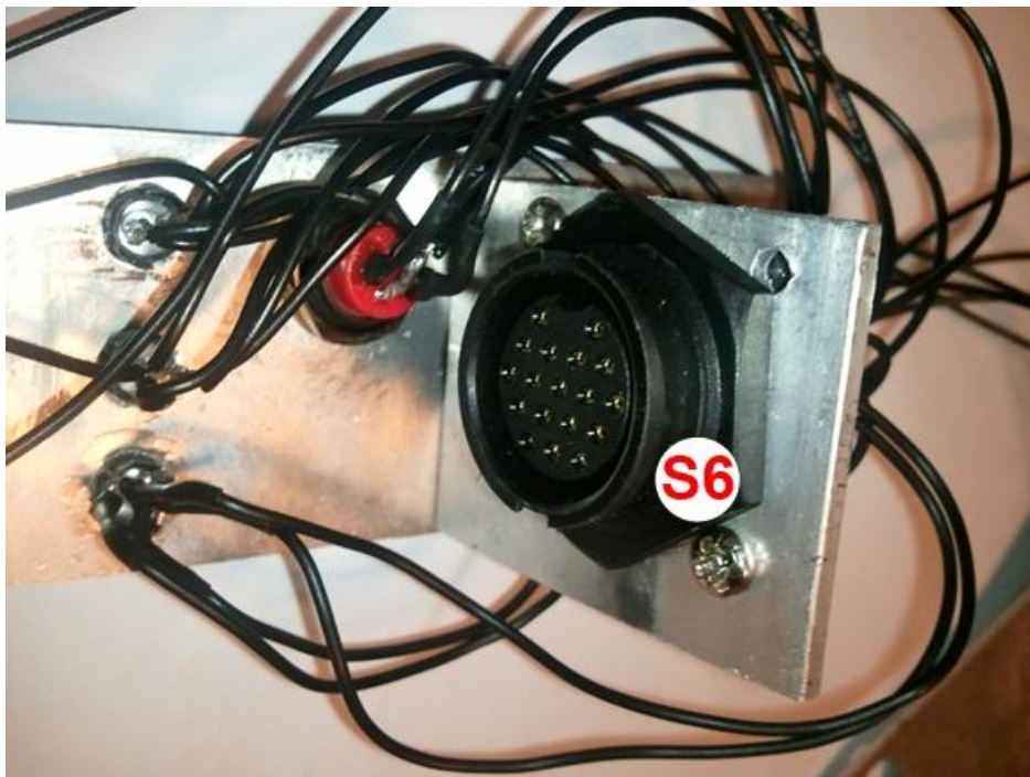
Figure 3.23 Placement of connector S6 mounted behind the dashboard.
