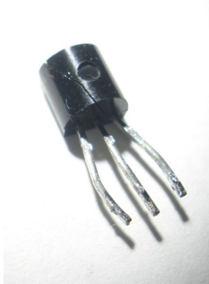
Figure 5.1 Transistor damaged by excessive base current
