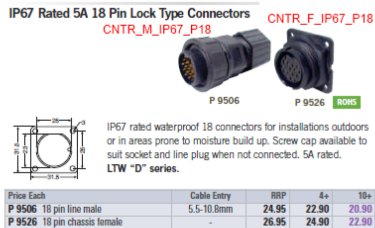
Figure 3.20 CNTR_M_IP67_P18 and CNTR_M_IP67_P18 connector specification [7]
