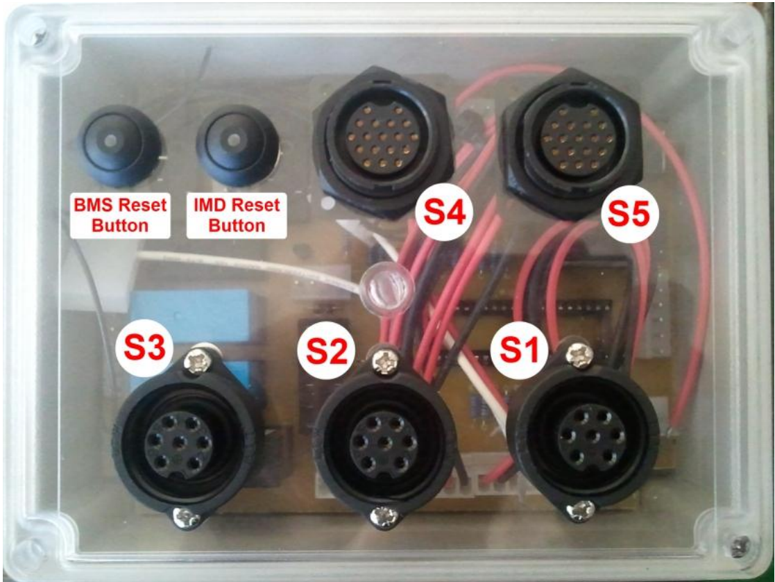
Figure 3.22 Placement of connectors S1, S2, S3, S4, S5 on the SCB lid.
