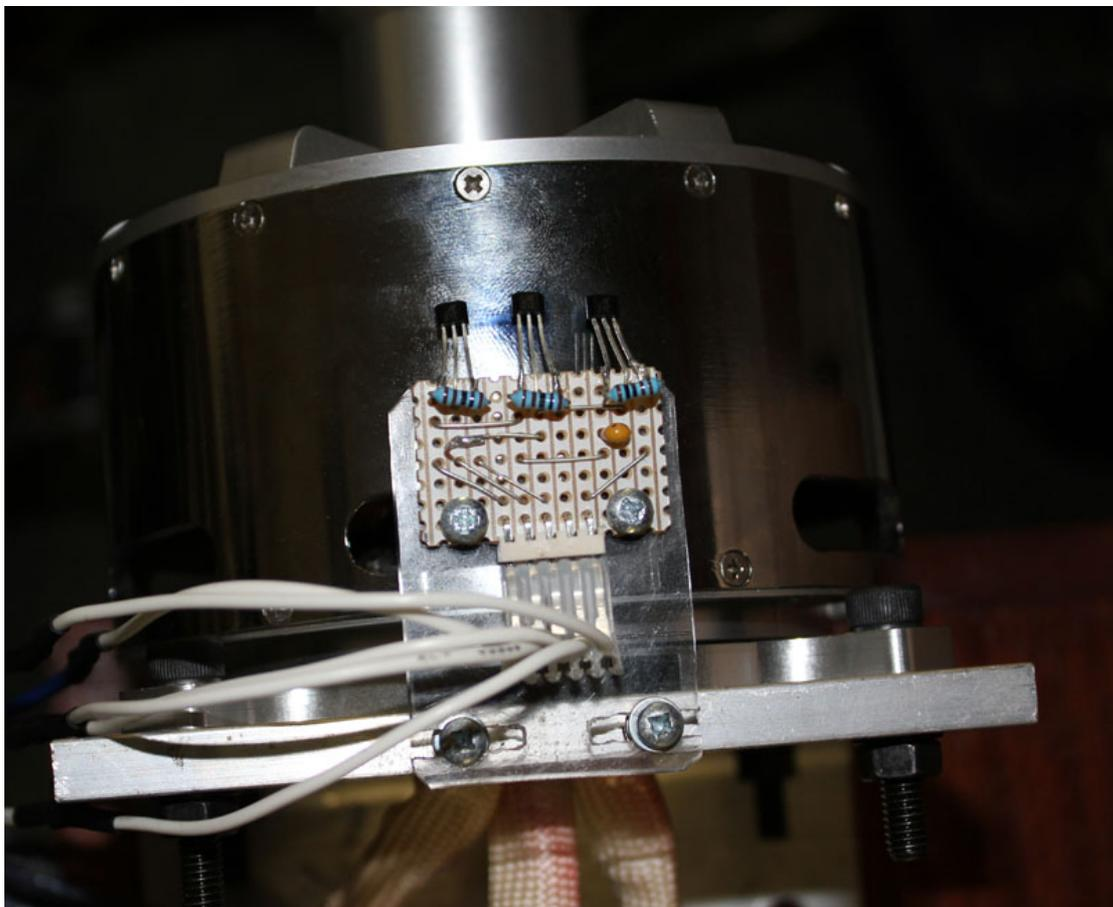
*Figure 24. Hall Effect Encoder mounted on the test platform*
