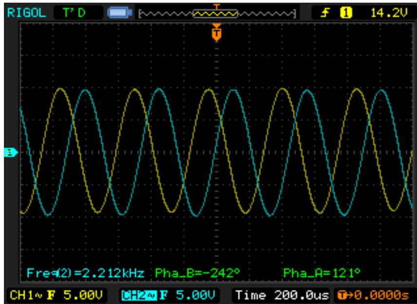
Figure 34. Phase Waveform – Filtered BEMF 2 phases
