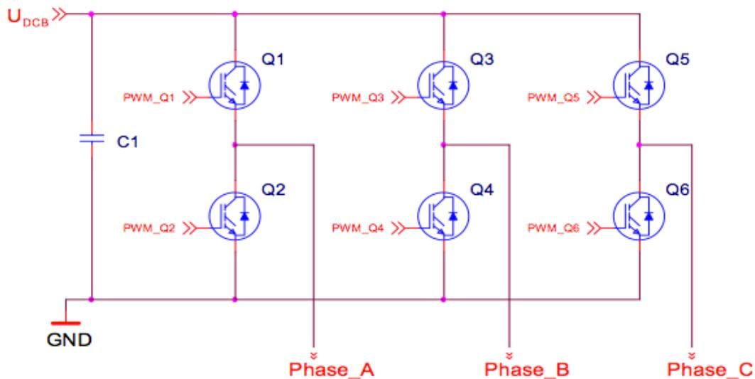
Figure 17. Mosfet Inverter Bridge [6]
