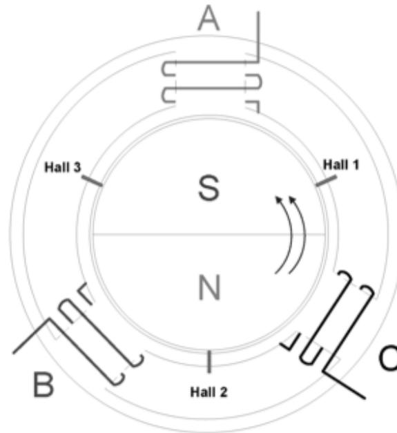
Figure 15. 3-Phase Single Pole Pair Motor – Hall Effect Locations [8]
