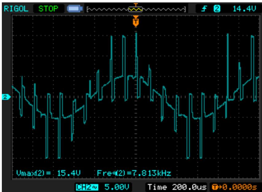
Figure 31. Phase Waveform – Low Throttle Demand
