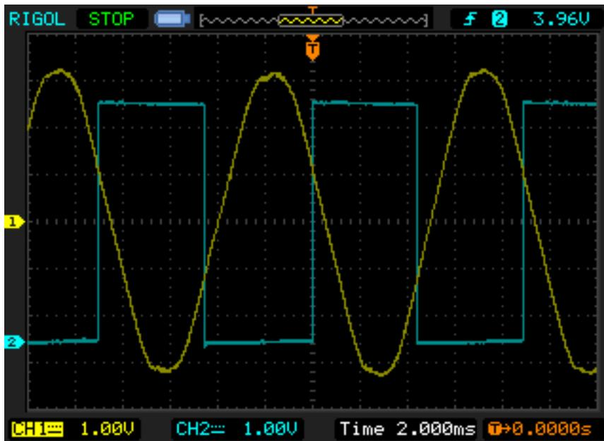
Figure 26. Hall Effect Output vs BEMF – Incorrect Alignment
