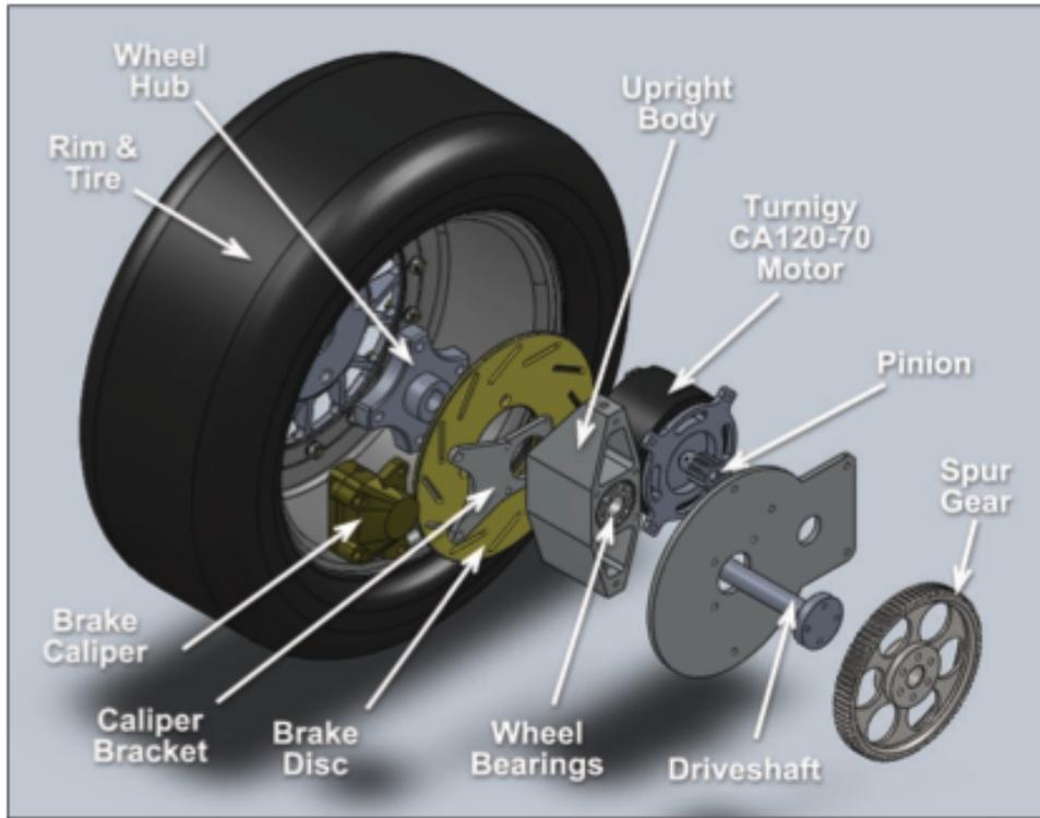
*Figure 1. In-wheel-hub motor and gearing design Source [1]*
