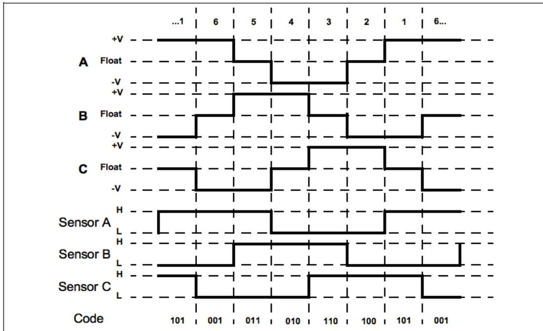
Figure 16. Hall Effect Signal vs Commutation Timing [3]
