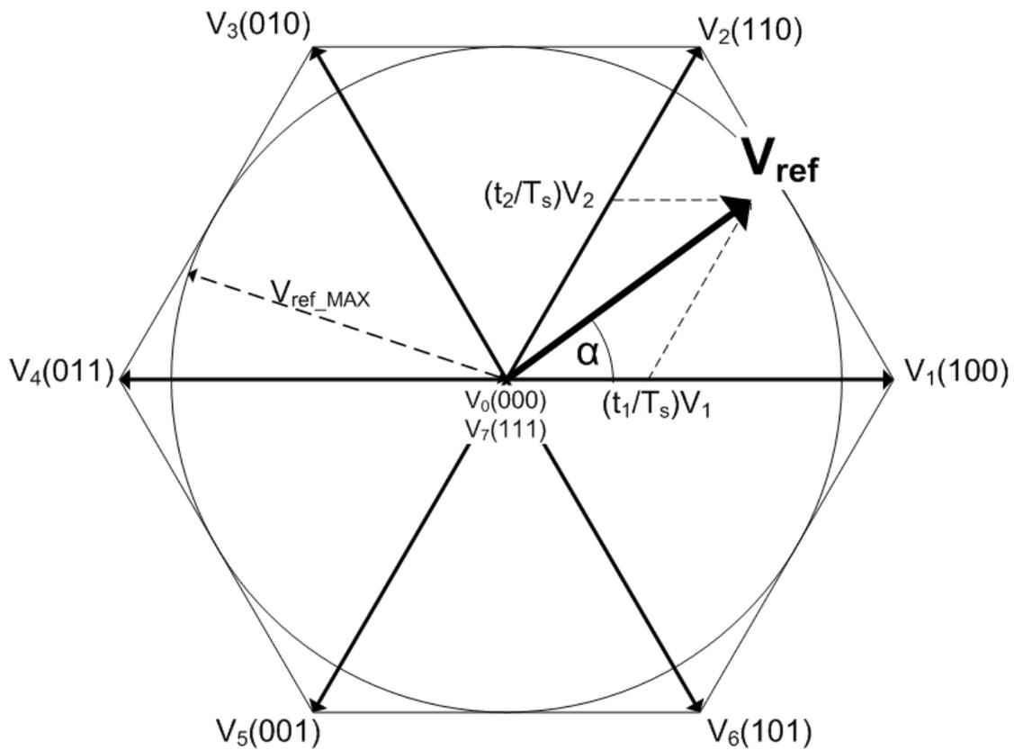
Figure 22. Space Vector Representation of a 3-phase System [12]
