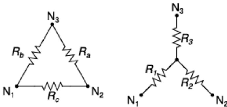
Figure 8. Delta vs Wye connection [10]
