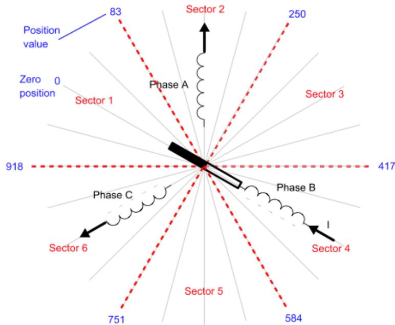
Figure 14. Quadrature Encoder Commutation Sectors [6]
