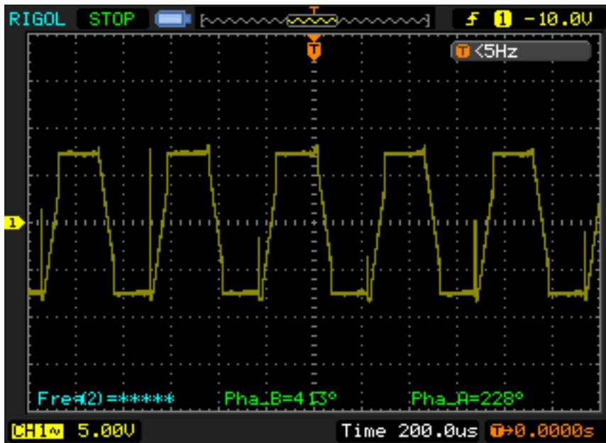
Figure 35. Inverter Output – Ground Referenced
