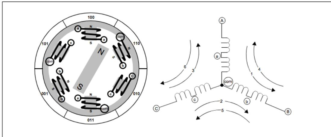
Figure 10. 3-phase BLDC Motor in Wye Configuration [3]
