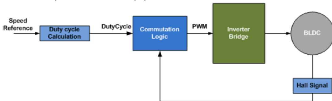
Figure 19. Open Loop Control Block Diagram [6]
