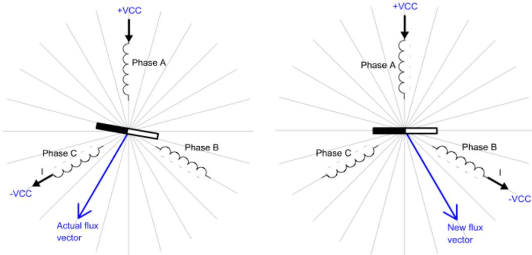
Figure 12. Flux Vector Rotation during Commutation [7]
