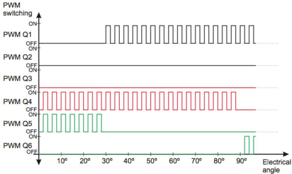
Figure 18. PWM Control Waveforms [6]
