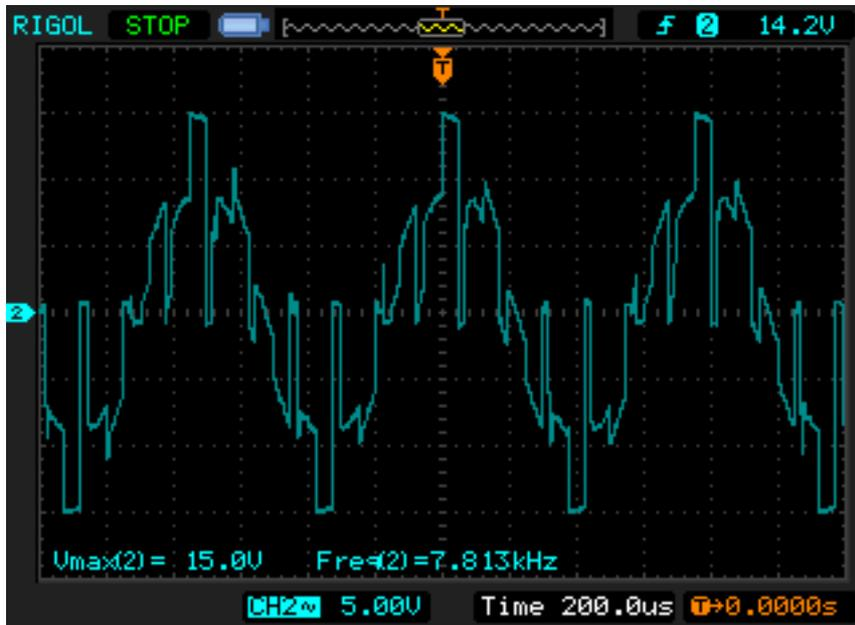
Figure 32. Phase Waveform – Medium Throttle Demand
