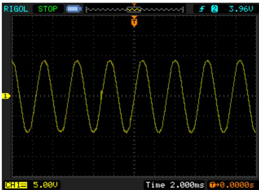
Figure 6. BEMF Waveform of the Turnigy CA120-70 BLDC Motor
