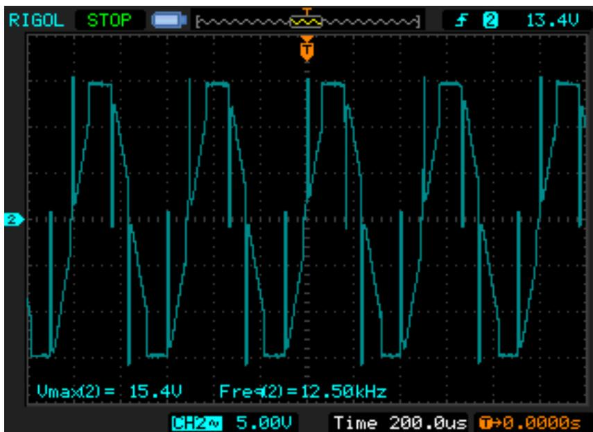
Figure 33. Phase Waveform – Full Throttle Demand
