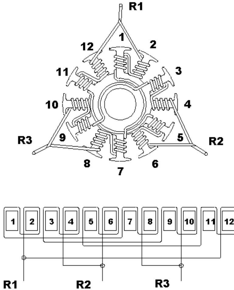
Figure 7. dRLK Winding Pattern – 12 Slot Stator
