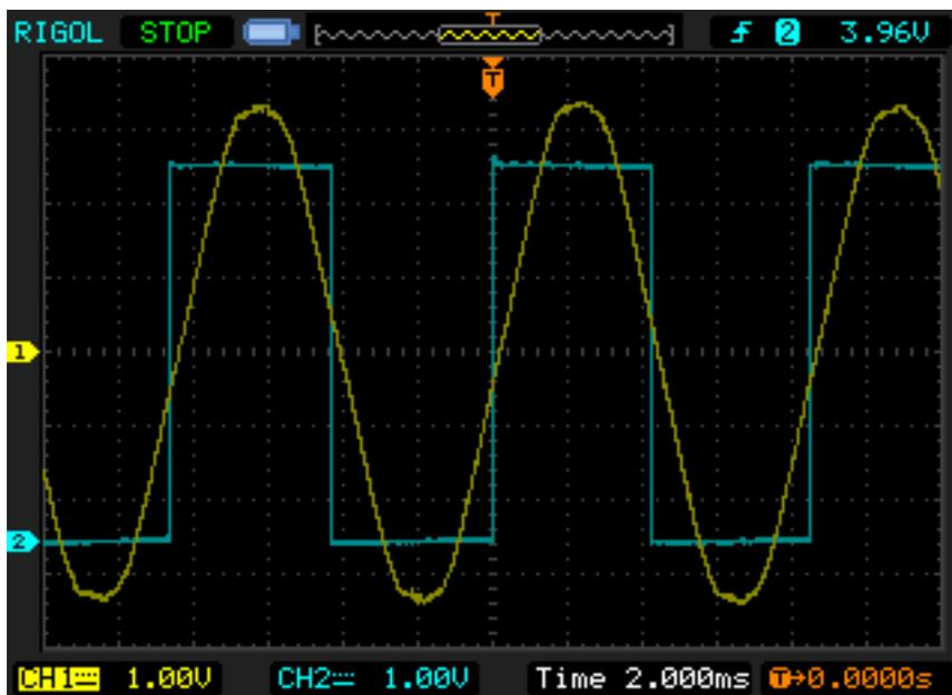
Figure 27. Hall Effect Output vs BEMF – Correct Alignment
