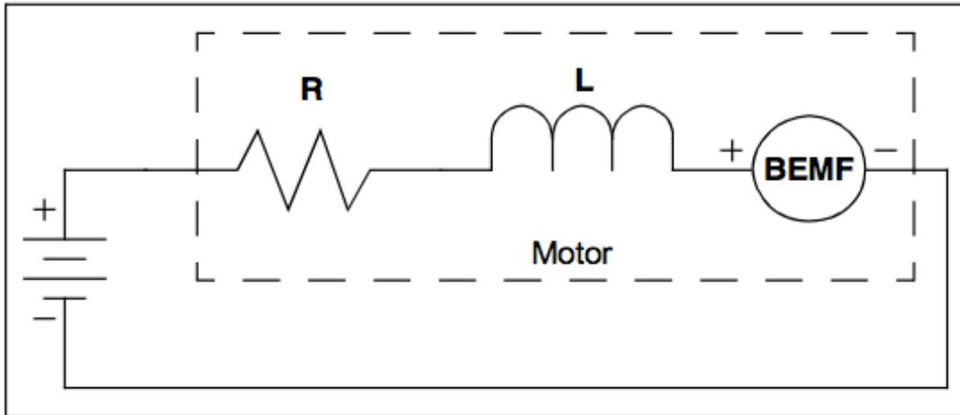
Figure 5. Model Representation of a Single Motor Phase
