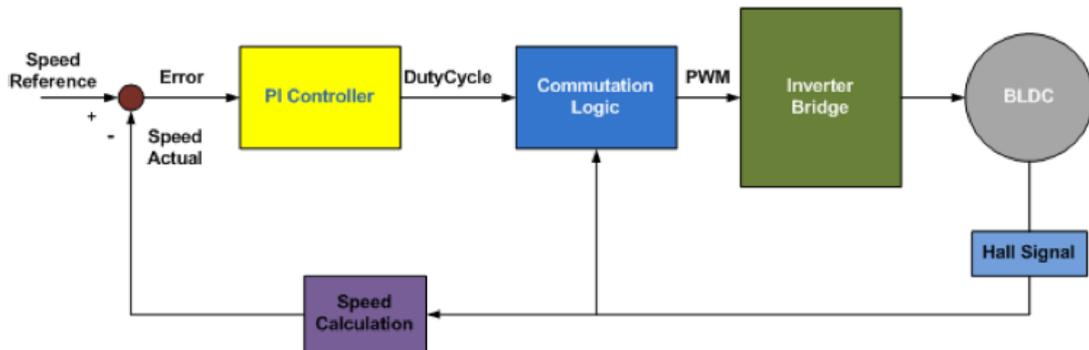
Figure 20. Closed Loop Control Block Diagram [6]
