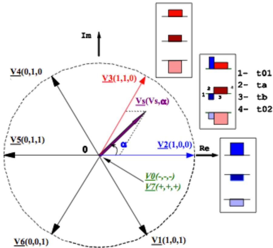
Figure 23. Space Vector Modulation Example [5]
