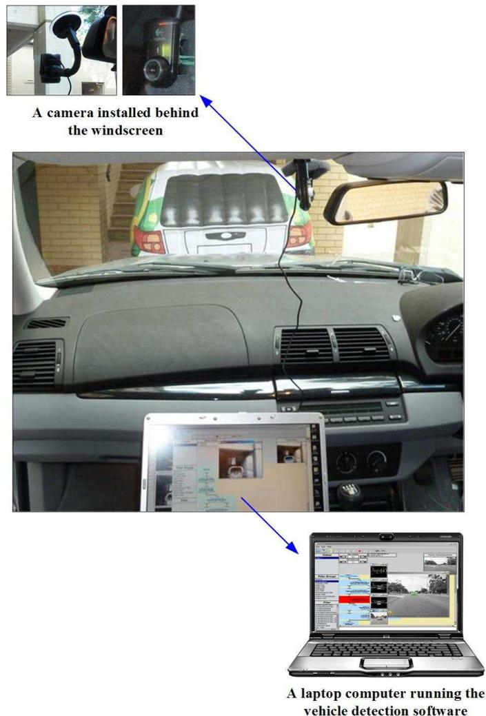
Figure 6.4: Figure shows the setup for testing the vehicle detection system in a BMW X5 vehicle
