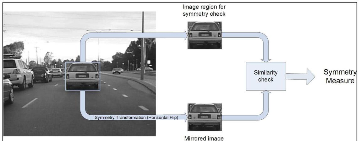
Figure 3.3: An example of vehicle detection using the direct approach. The similarity between the original image and the symmetry transformed image (in this case, the horizontal reflectional symmetry) is checked to determine the degree of symmetry
