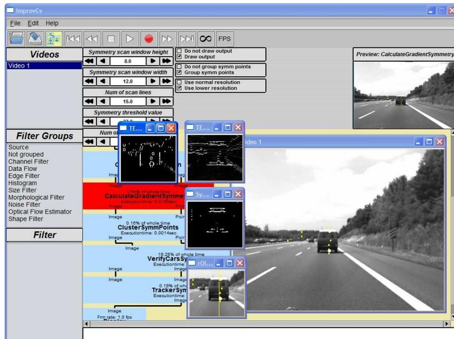
Figure 3.18: Implementation of the symmetry-based vehicle cueing system on the ImprovCV image processing framework
