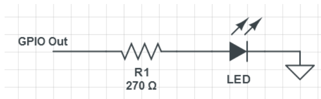
Figure 20: Circuit to connect LED to the Raspberry Pi’s GPIO pin
