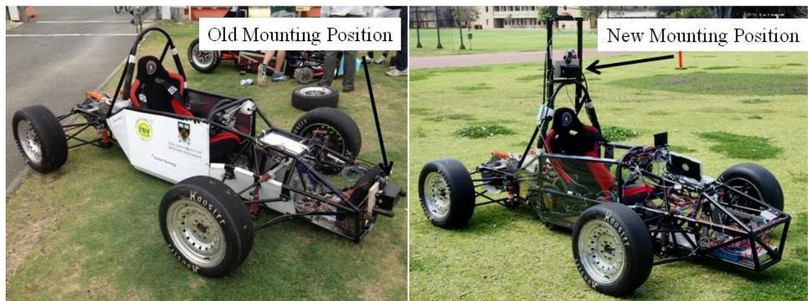
Figure 2: Old and new mounting positions of the IBEO sensor
