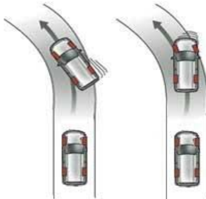
Figure 2-2: Cases of Oversteer (left) and Understeer (right)
