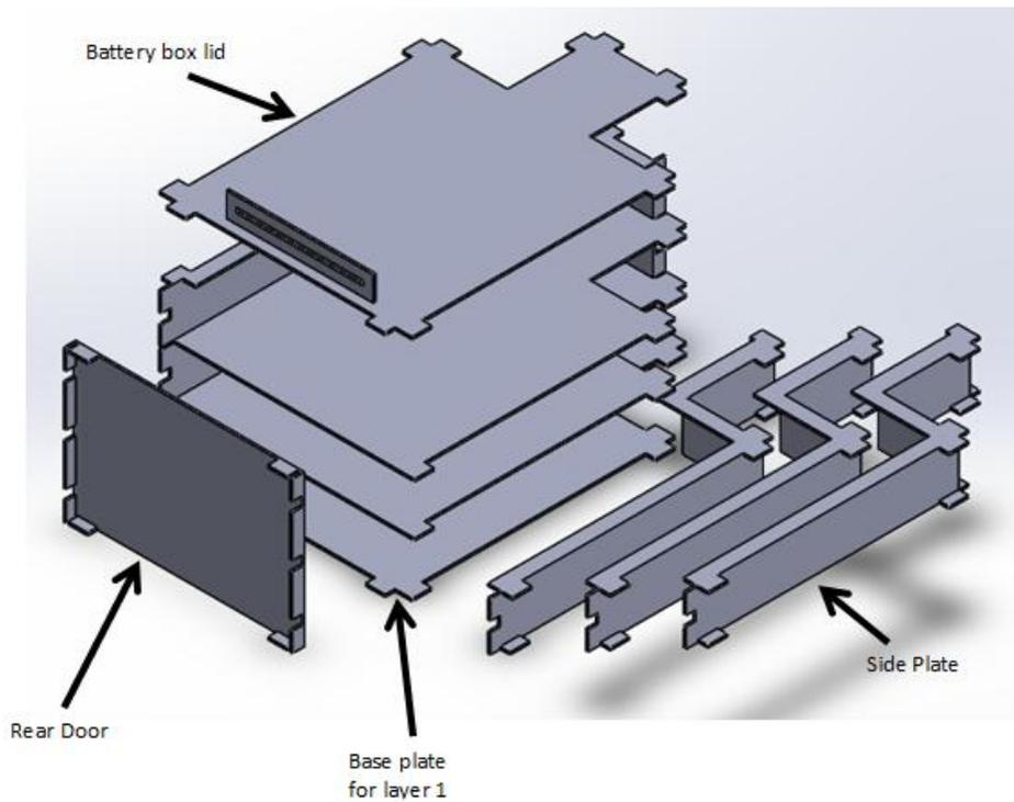
Figure 28 Exploded view of the initial design
