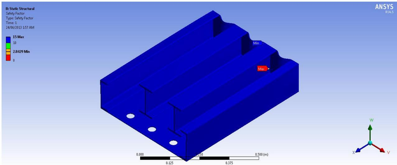
Figure 39 safety factor, front impact, layer 2
