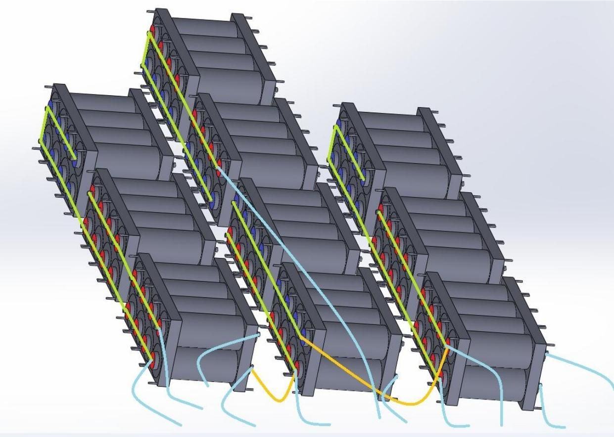
**Figure 24 Initial battery module arrangement**
