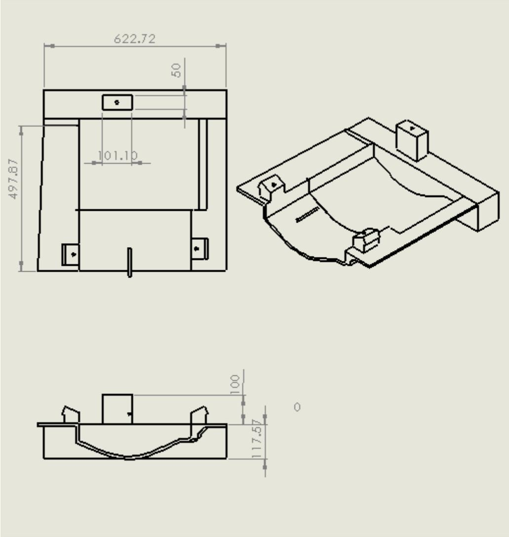
Figure 50 Dimensions for the surface map.
