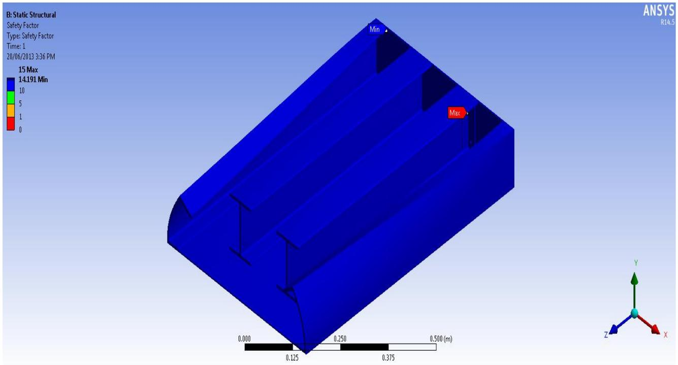
Figure 37 Safety factor, vertical impact, layer1
