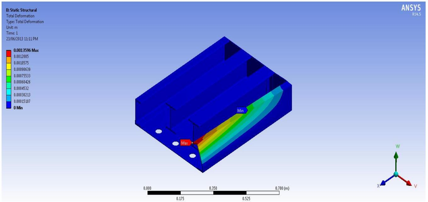
**Figure 40 Total deformation, side impact, layer 2**
