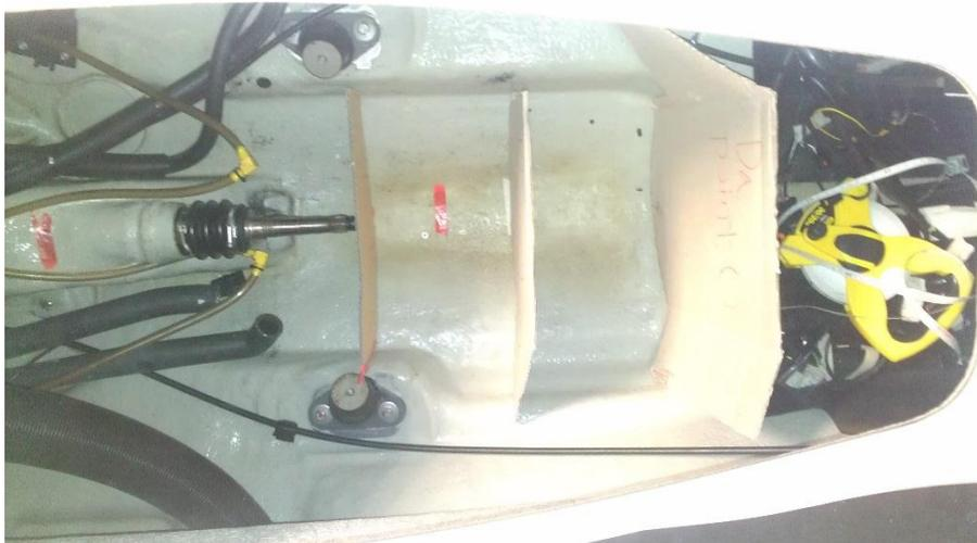
**Figure 6 Card board profile alignment**
