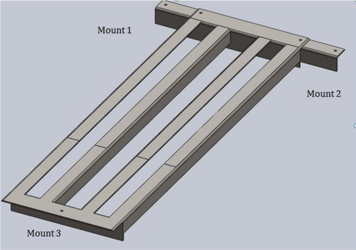
Figure 51 Support Frame design
