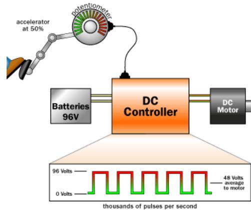
Figure 2 DC motor system
