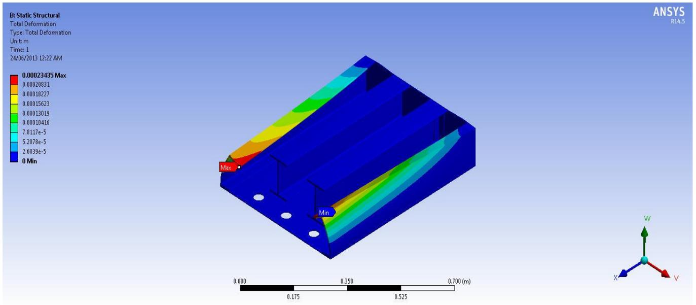
Figure 42 Total deformation, vertical impact, and layer 2
