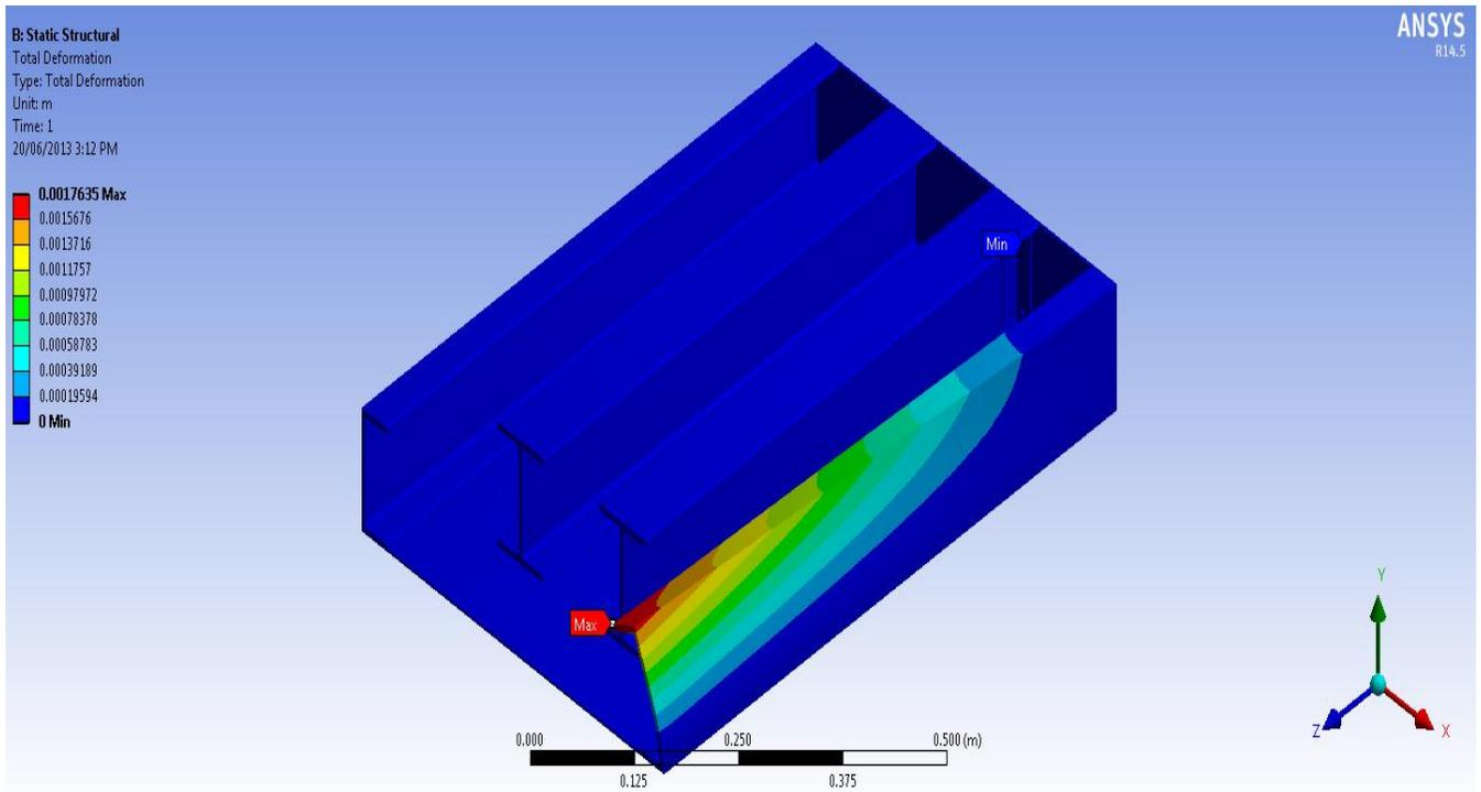
Figure 34 Total deformation side Impact Layer 1
