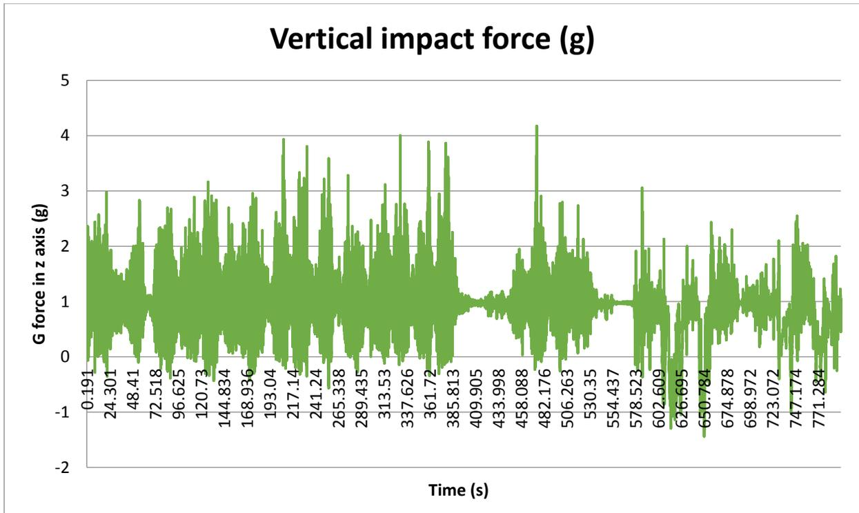
Figure 16 G-force recorded in the z axis
