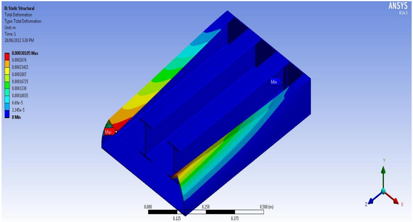
Figure 36 Total deformation, vertical impact, layer 1
