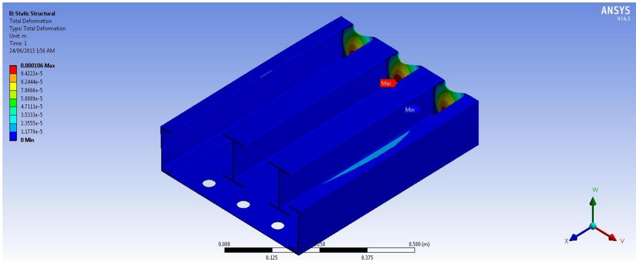
Figure 38 Total deformation, front impact, layer 2
