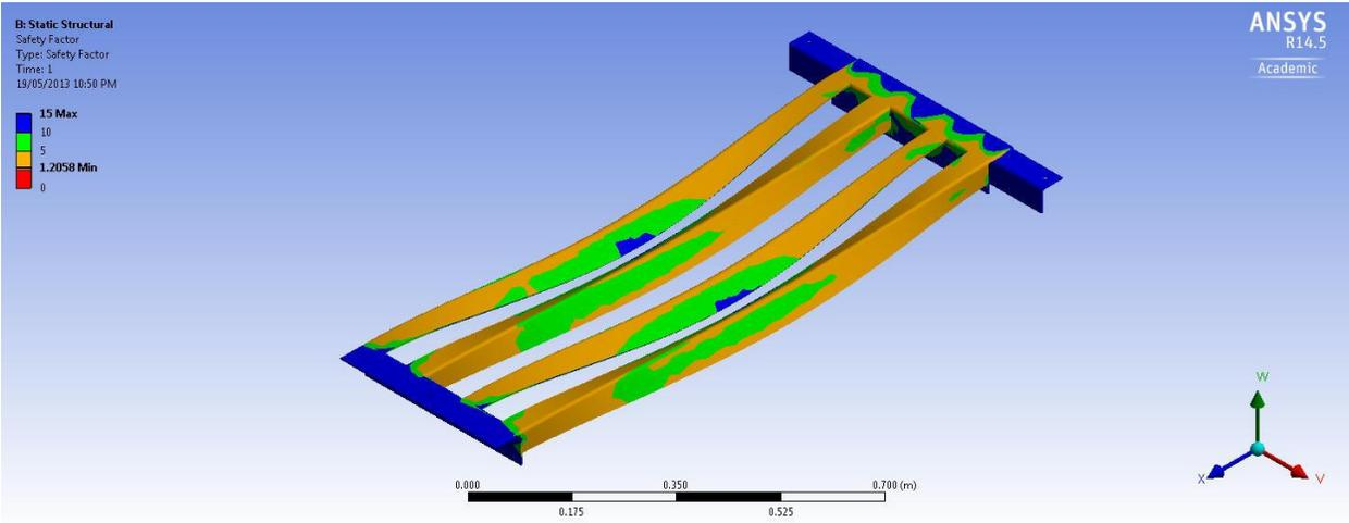
Figure 52 Support mount Vertical Impact of 10g
