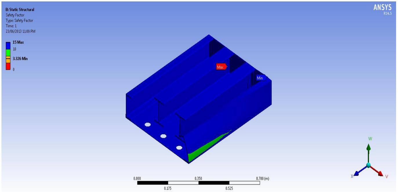
Figure 41 Safety factor, side impact, layer 2
