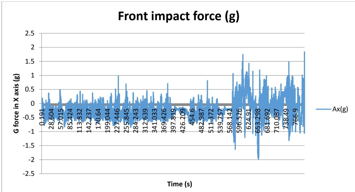
Figure 17 G-force recorded in the x axis
