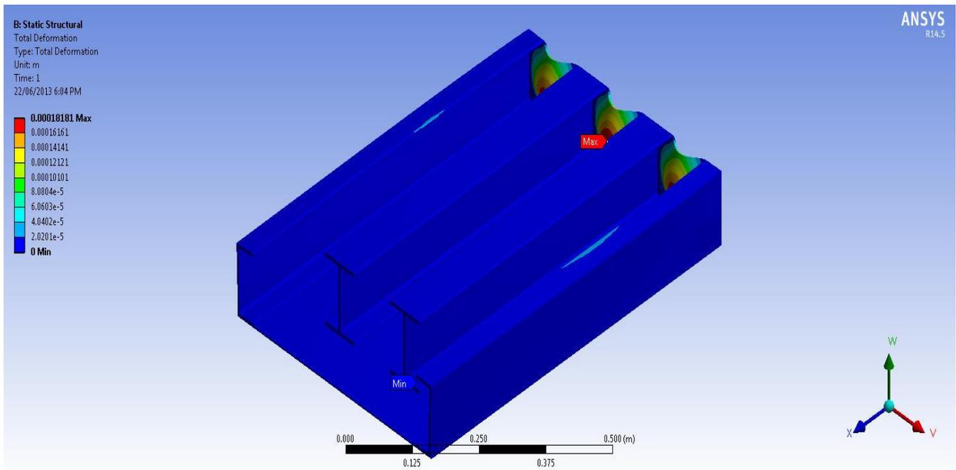
Figure 32 Total deformation, front impact, layer 1
