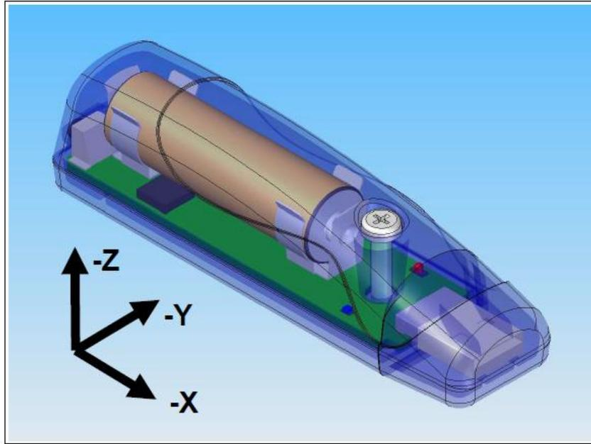
Figure 15 Coordinate system for the accelerometer
