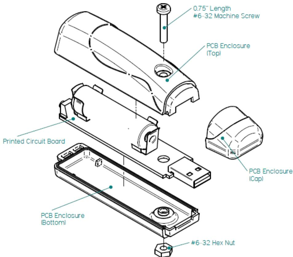
Figure 14 Accelerometer assembly
