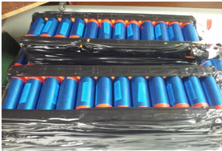
Figure 3.3.6: Battery cells lined with tape.
