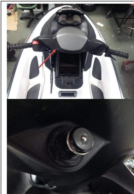
bridge Figure 4.2.4.1: Deadman's switch
