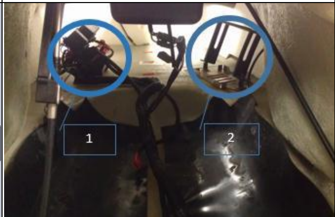
Figure 3.3.5: Fuel tank mounting points - (Jayamanna 2013)
