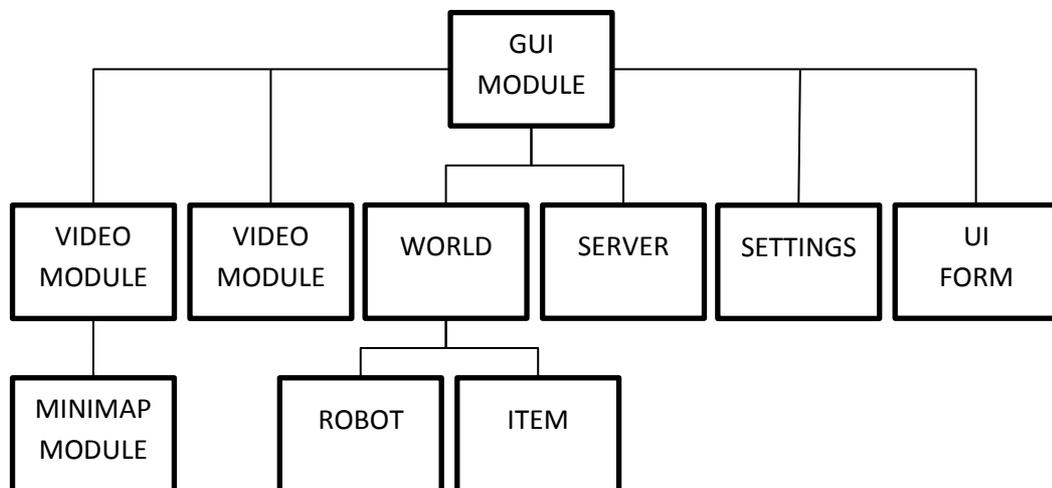
**Figure 3.1** The final software block diagram for the master user interface.
