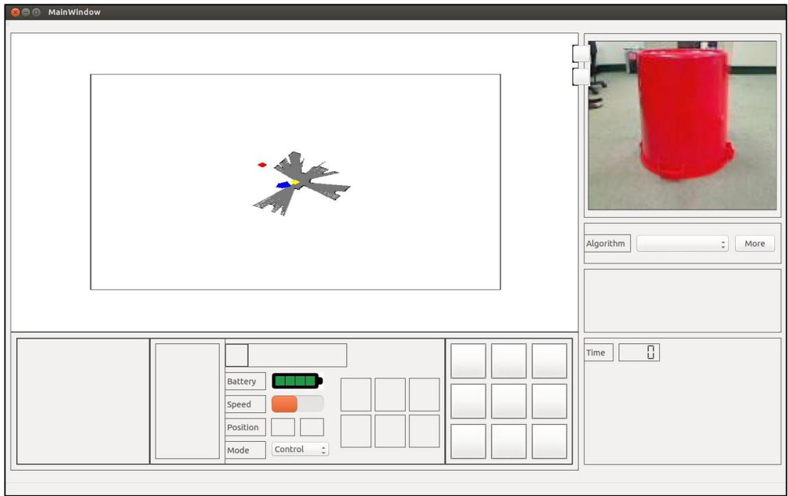
**Figure A3** Graphical interface version 3, functional; map module, video feed, robot selection and goal commands. Basic control panel functions were implemented.
