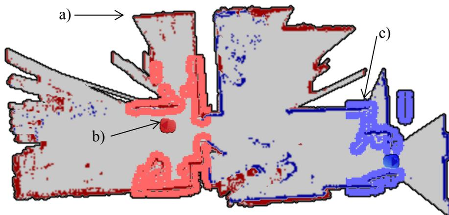
**Figure 3.6** The Map Module demonstrating a) colour coded maps, b) robot position and c) colour coded costmaps.
