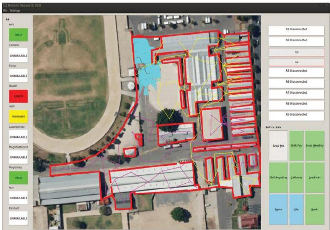
**Figure 1.4** A screenshot from the system developed by the RASR team for MAGIC2010. Shown on the right hand side is the robot status feedback mechanism. The central display shows the robots exploring the environment with overlaid robot position (Lacaze, et al., 2012).
