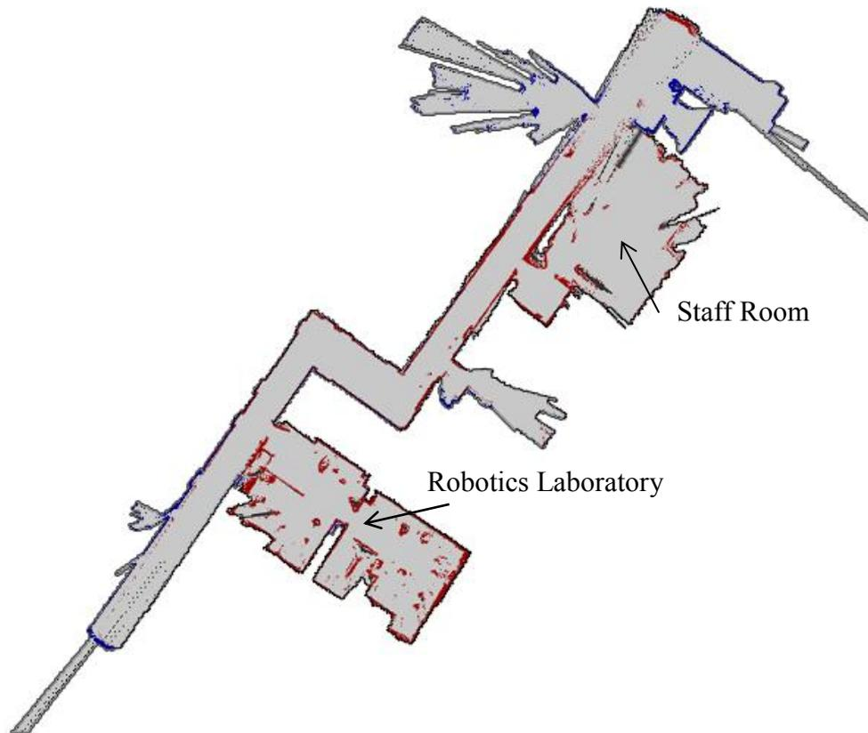
**Figure 4.2** A user generated map of the third floor of the Electrical Engineering building using two robots. The robotics laboratory and staff room are labelled.
