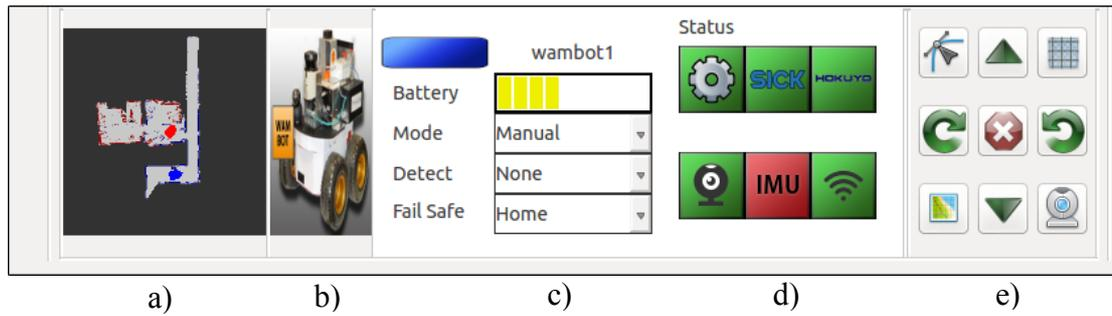
**Figure 3.8** Display panel for a selected robot showing a)minimap, b)robot icon, c) central controls, d) status display and e) command pad.
