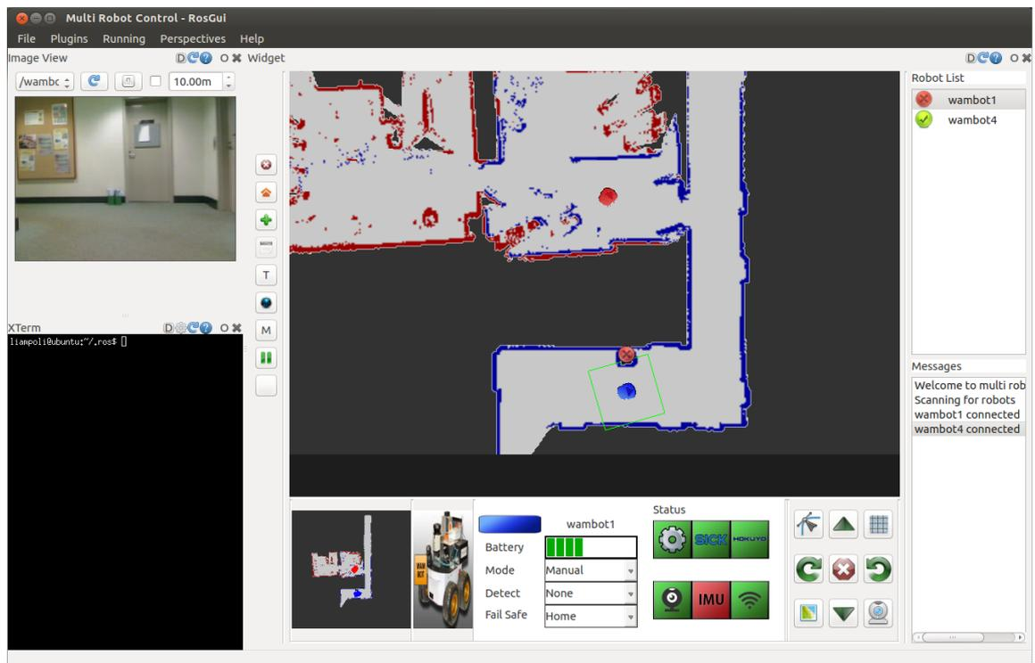
**Figure 3.4** The final graphical user interface displayed on the master computer. In the screen shot the user is controlling two robots, with robot 1, shown in blue currently selected.
