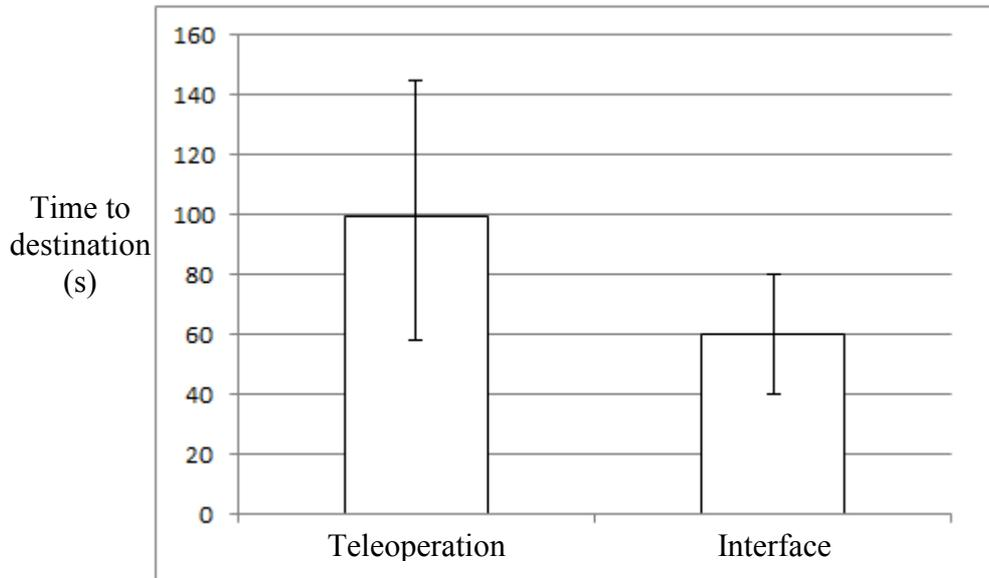
**Figure 4.1** Mean time for users to drive to the destination point, a sample size of eight users. For teleoperation mean = 99.6s, slowest time = 145s, fastest time = 59s and for interface control mean = 60s, slowest time = 80s, fastest time = 40s. Error bars represent the fastest and slowest user times for the case.
