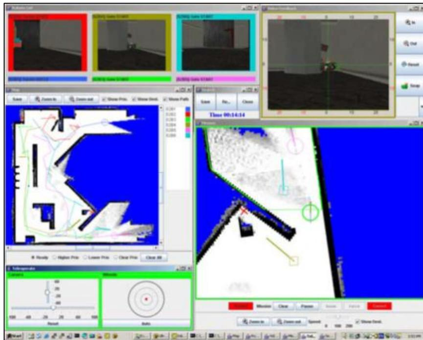
**Figure 1.2** A multi-robot interface developed by the University of Pittsburgh and Carnegie Mellon University. Four camera feeds are shown and two maps. The system was developed and tested using simulated robot data. (Wang, et al., 2008).
