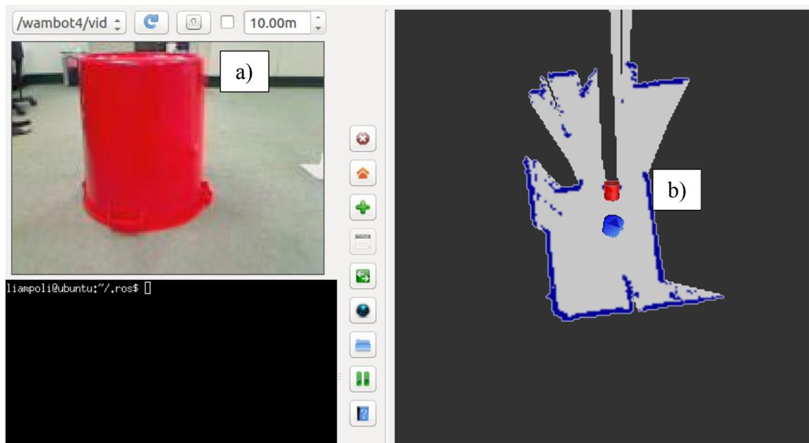
**Figure 3.12** An example of a robot detecting a red barrel a) the current robot video feed b) the red barrel icon being displayed on the map in the position of the detected item.
