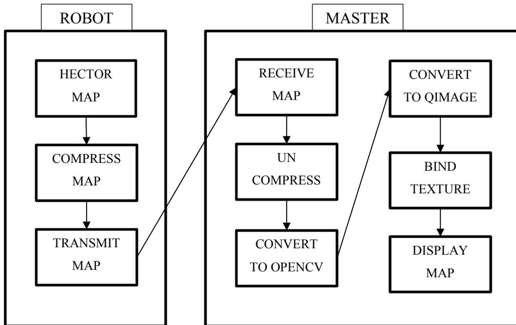
**Figure 3.5** Block diagram illustrating the map display pipeline. Data transmission between the robot and master is facilitated through the Wi-Fi network.
