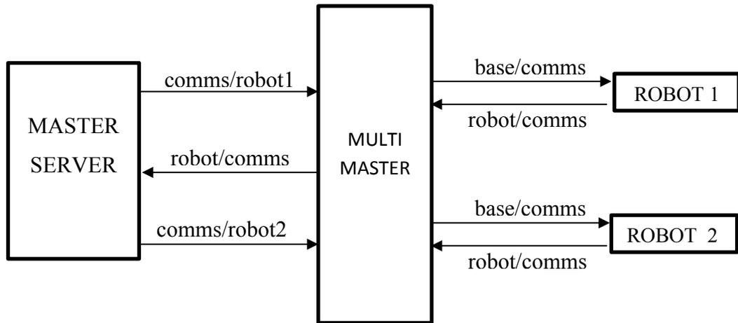
**Figure 3.2** LPCP block diagram, illustrating communication between a single master and multiple robots. The topic names are displayed.
