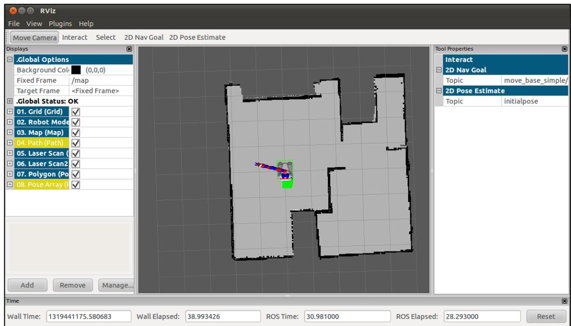
**Figure 1.1** A screenshot from Rviz showing the localised position of a single robot within a map (Fraunhofer IPA, 2011).
