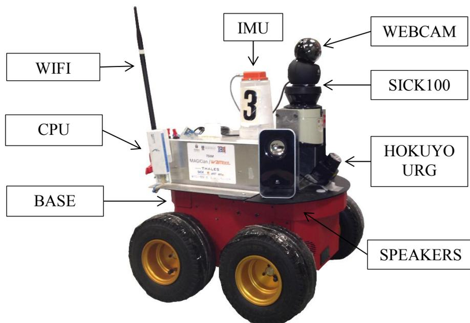
**Figure 2.1** A image illustrating the hardware components of each robot.
