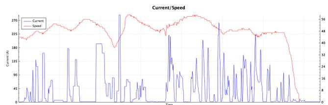
Fig. 11. A current/speed graph created by the GUI on a drive around UWA in the REV Eco. The main purpose of the graph is for drivers to view their driving habits in real time and attempt to reduce peaks in current.
