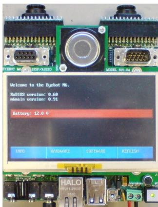
Figure 6. The Eyebot M6, the controller to control instrumentation in the REV Eco up until 2013.
