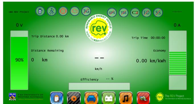
Fig. 19. The Home window of the GUI used in the REV Racer. Note the coloured buttons, due to touchscreen functionality, and the extra battery button.
