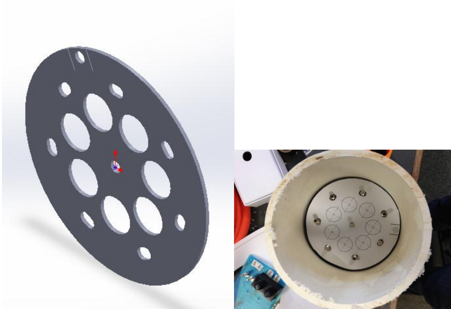
Figure 12: Original Design of the plate to connect the 8 cell configuration together.
