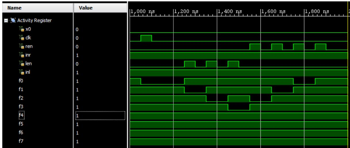
Figure 53 - VHDL Simulation - Activity Register
