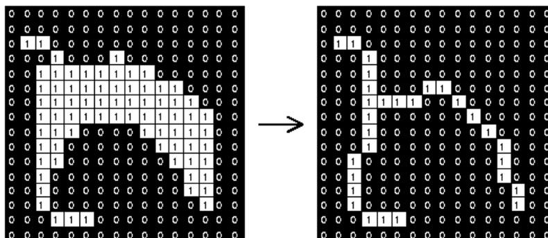
Figure 26 - Skeletonisation using Thinning Example [15]
