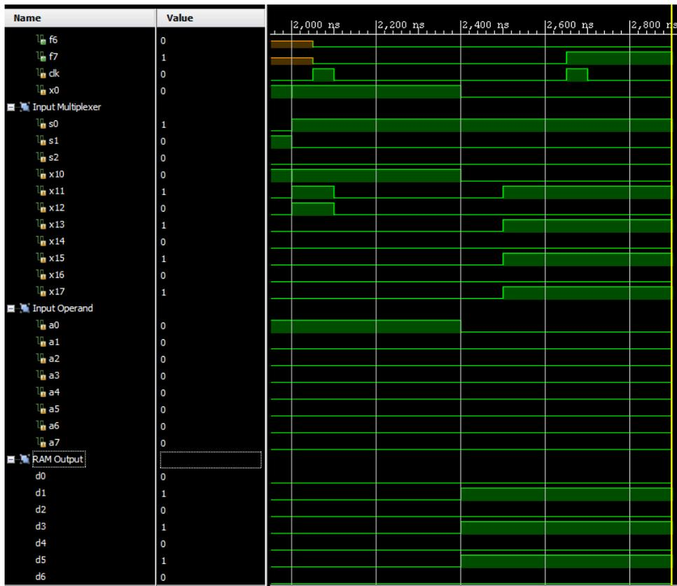
Figure 54 - VHDL Simulation - Load (RAM)
