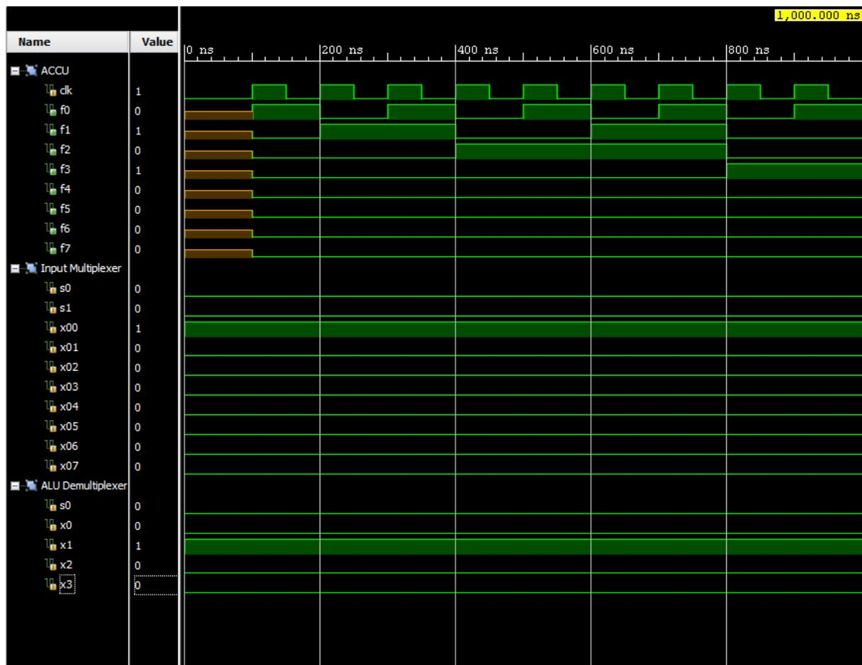
Figure 52 - VHDL Simulation - Addition
