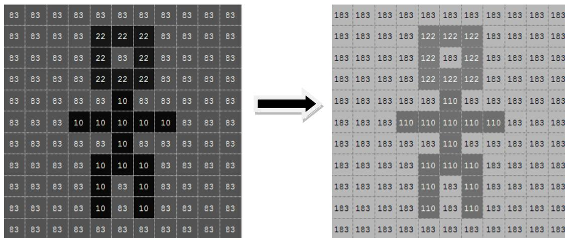
Figure 2 - Brightening Example
