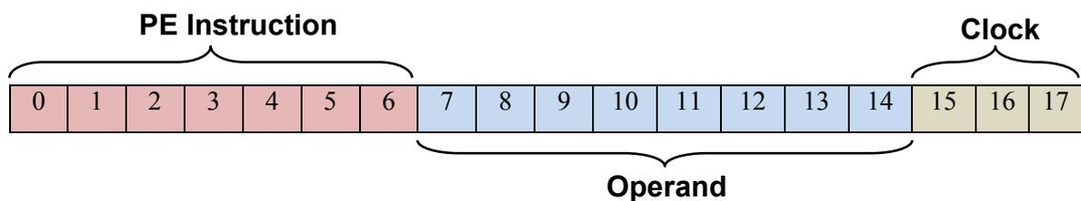
Figure 19 - Sequencer CPU - Instruction Bus Bits
