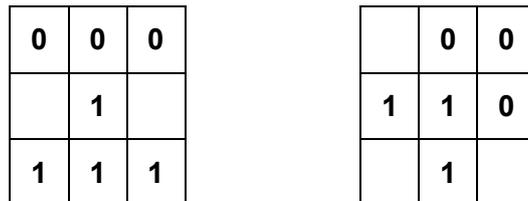
Figure 25 - Structuring elements for Thinning
