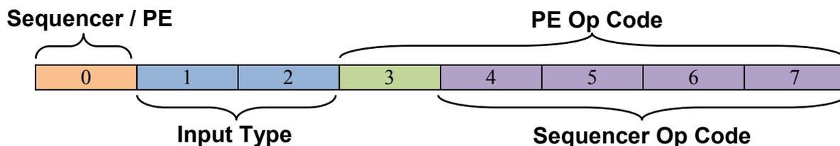
Figure 20 - Sequencer CPU - Instruction Breakdown
