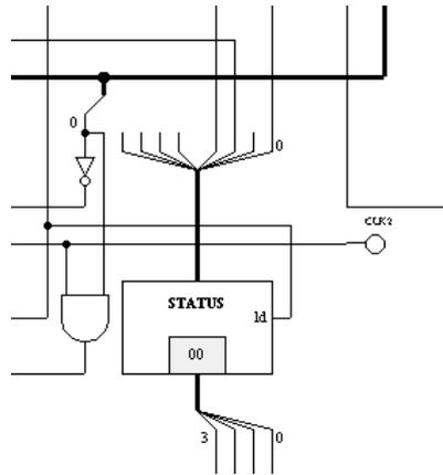
Figure 29 - PE Design - Status Register
