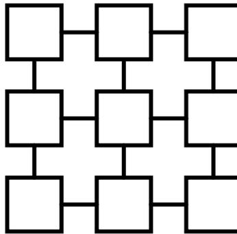
**Figure 7 - 2D Mesh Network**
