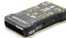
Figure 3: Pixhawk flight controller. Copied from (Pixhawk, 2015)
