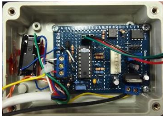
Fig 16. SAE Safety supervisor existing circuit
