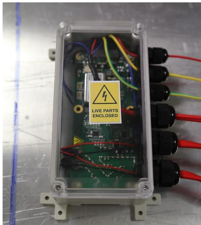
Figure 1 - Bender Insulation monitoring device IR155-3204.
