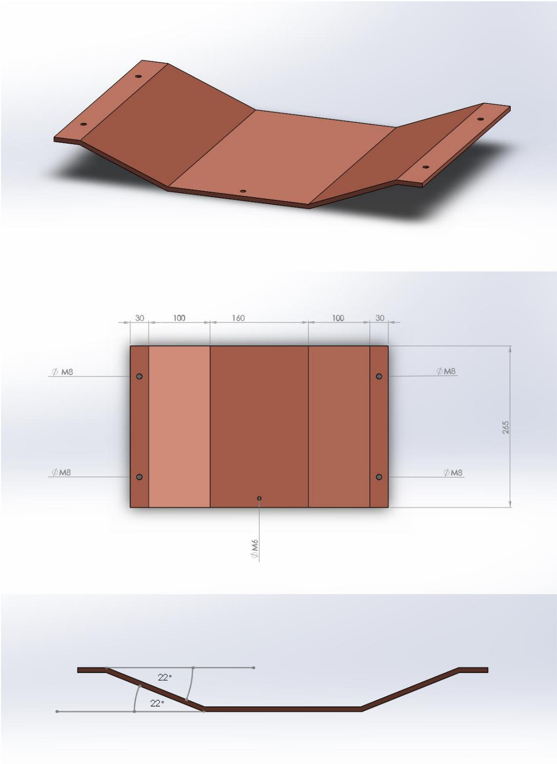
Figure 3 - Model of earth electrode displaying size and shape dimensions are in mm.
