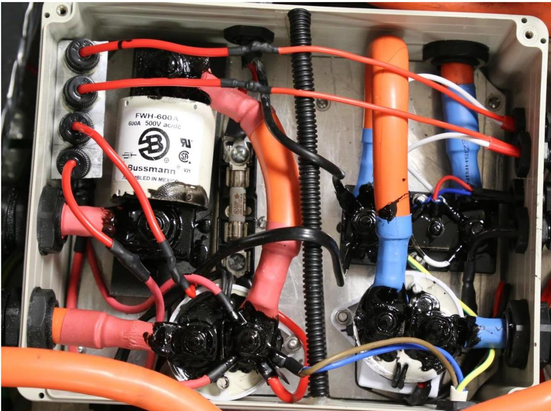
Figure 4 - ELV Switchgear and fuse box showing double insulation by use of heatshrink and putty.
