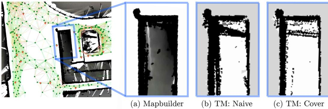
**Figure 7.28. Global occupancy gridmap comparison:** Comparison between outputs from Mapbuilder and Strom and Olson’s approach [56]. Mapbuilder’s output from the start of Phase 2 is shown for context (left). The three insets show enlargements of a barrel at the corner of a 5 meter wide building. (a) shows Mapbuilder’s output, note the aerial map is visible through the inside of the building. (b) is TM’s naive rasterization approach, and (c) is their node covering approach.
