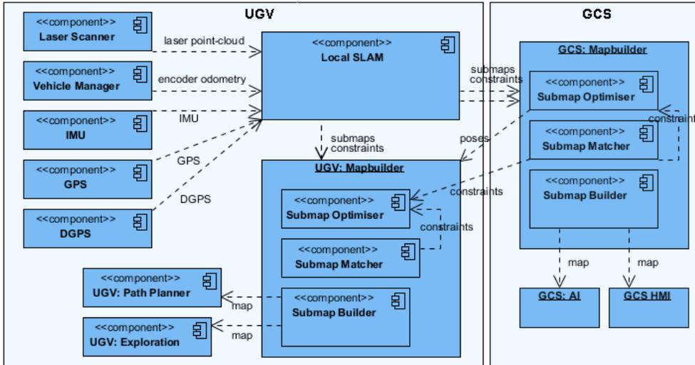
**Figure 4.6. Mapbuilder logical design:** Software components and data flows on a typical UGV participant (left) and GCS participant (right) are shown. Decentralized communications are performed using the DDS middleware.
