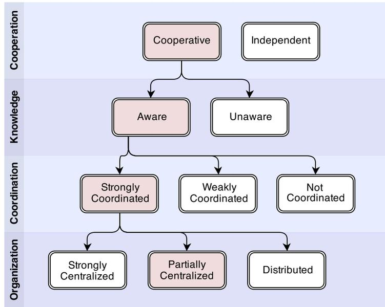
**Figure 1.4. Multi-robot system taxonomy:** Types of cooperation, levels of knowledge sharing, methods of coordination and types of centralization are shown. Boxes highlighted in red indicate the MRS considered in this research. Image from Farinelli et al. [18]
