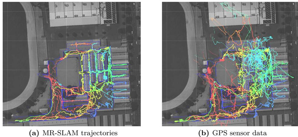
**Figure B.7. Phase 2:** TM’s reprocessed MR-SLAM map from [328] showing GPS data. Trajectories for 12 UGVs are shown in each figure, with the hue mapped from red at the start to blue after 2 hours. A 50 meter grid is overlaid. In (b) GPS position data can be seen drifting widely, with up to 80 meters error around the horse stables due to multipath effects. Maps courtesy Ryan Morton.
