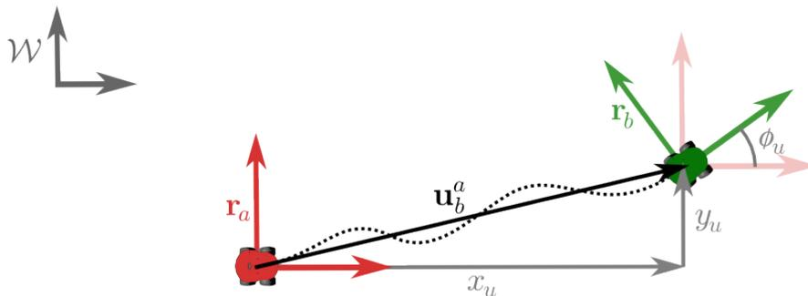
**Figure 2.2. 2-D rigid-body transformations:** A robot drives from pose  $\mathbf{r}_a$  to  $\mathbf{r}_b$ . During this drive it measures the incremental pose change, or odometry,  $\mathbf{u}_b^a = [x_u, y_u, \phi_u]^T$ . Both poses describe local coordinate frames in the world frame  $\mathcal{W}$ , while  $\mathbf{u}_b^a$  describes a rigid-body transformation.
