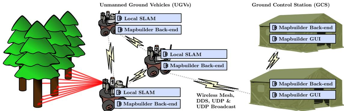
**Figure 4.1. Mapbuilder architecture and software deployment diagram:** Instances of the Local SLAM component execute on each UGV, processing sensor data. Instances of the Mapbuilder back-end execute on all participants (UGV and GCS computers) where it produces distributed copies of the global map. The Mapbuilder GUI software is used by operators at the GCS.
