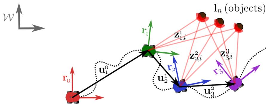
**Figure 2.3. Measurement transformations using  $\mathbb{SE}(2)$ :** A robot drives from pose  $\mathbf{r}_0$  to  $\mathbf{r}_1$ ,  $\mathbf{r}_2$  and  $\mathbf{r}_3$  (local coordinate frames), measuring odometry transform  $\mathbf{u}_1^0$ ,  $\mathbf{u}_2^1$  and  $\mathbf{u}_3^2$ . From each pose,  $\mathbf{r}_t$ , it makes measurements,  $\mathbf{z}_{t,i}^t$ , to the objects in the environment.
