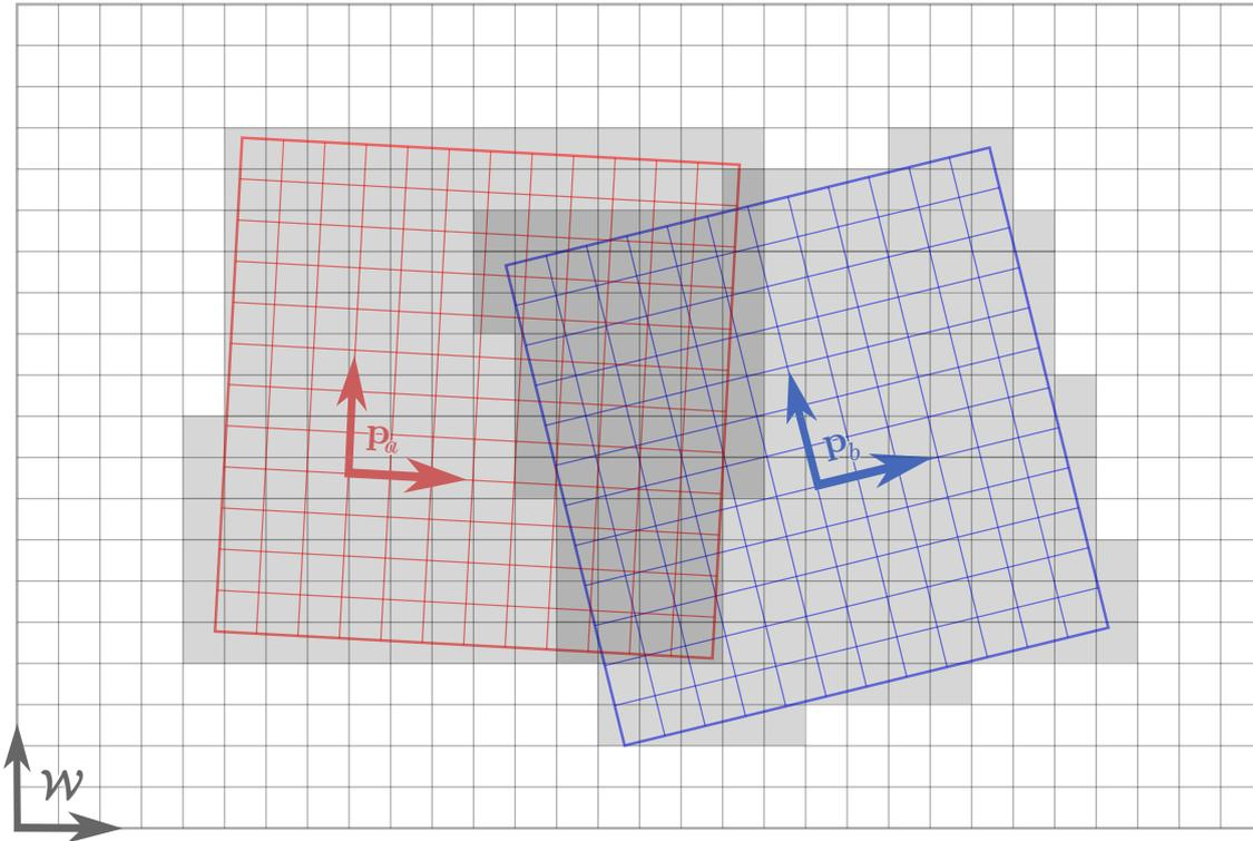
**Figure 5.2. Occupancy Gridmap Fusion:** Two submap gridmaps with origins at  $\mathbf{p}_a^{\mathcal{W}}$  (red grid) and  $\mathbf{p}_b^{\mathcal{W}}$  (blue grid) are being fused into the global output gridmap  $\mathcal{W}$  (gray grid). The inner loop of the algorithm described here iterates over the output gridmap cells that are covered by the submap gridmaps (gray squares). This is a typical rasterization operation in computer graphics. Cell occupancy values are not shown for clarity.
