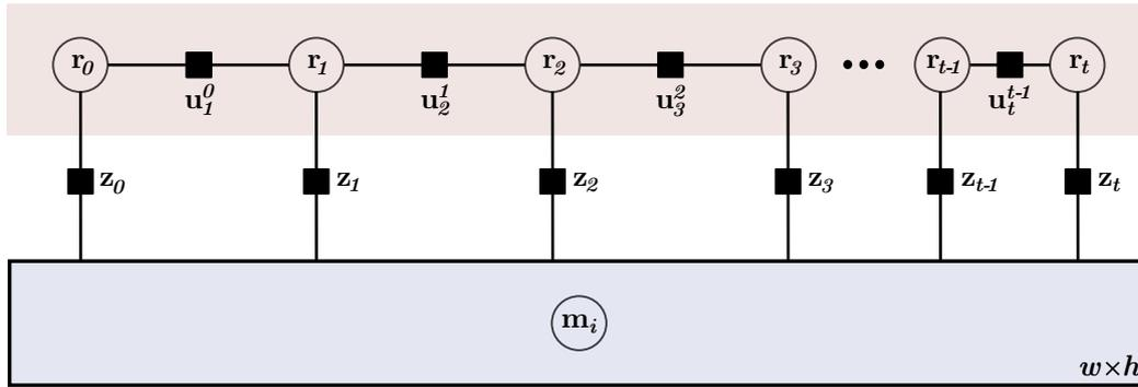
**Figure 2.16. Factor graph for occupancy gridmap SLAM:** Full SLAM factor graph with plate notation [100], the map is represented by an occupancy gridmap with cells,  $m_i$ . Variable nodes are large circles, while factor nodes are squares. Robot poses,  $r_t$ , are variable nodes that are separated by either odometry factors,  $u_t^{t-1}$ , or measurement factors,  $z_t$ .
