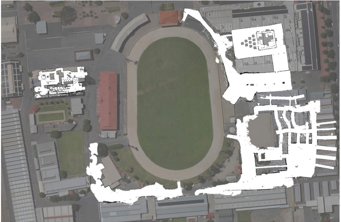
**Figure B.2. Team Michigan challenge day results:** Occupancy gridmaps superimposed on aerial imagery. TM won the challenge by exploring 100 % of the first two phases and 10 % of the third. TM released more accurate post-processed maps after the challenge. Gridmaps courtesy Ed Olson et al. [53, 54]. Aerial imagery courtesy DSTO.
