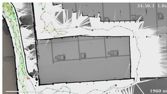
(d) **34m 50s:** Before loop closure between two UGVs at top center. Perceptual aliasing and odometry errors have shortened the walls, however it is unclear which ones.
