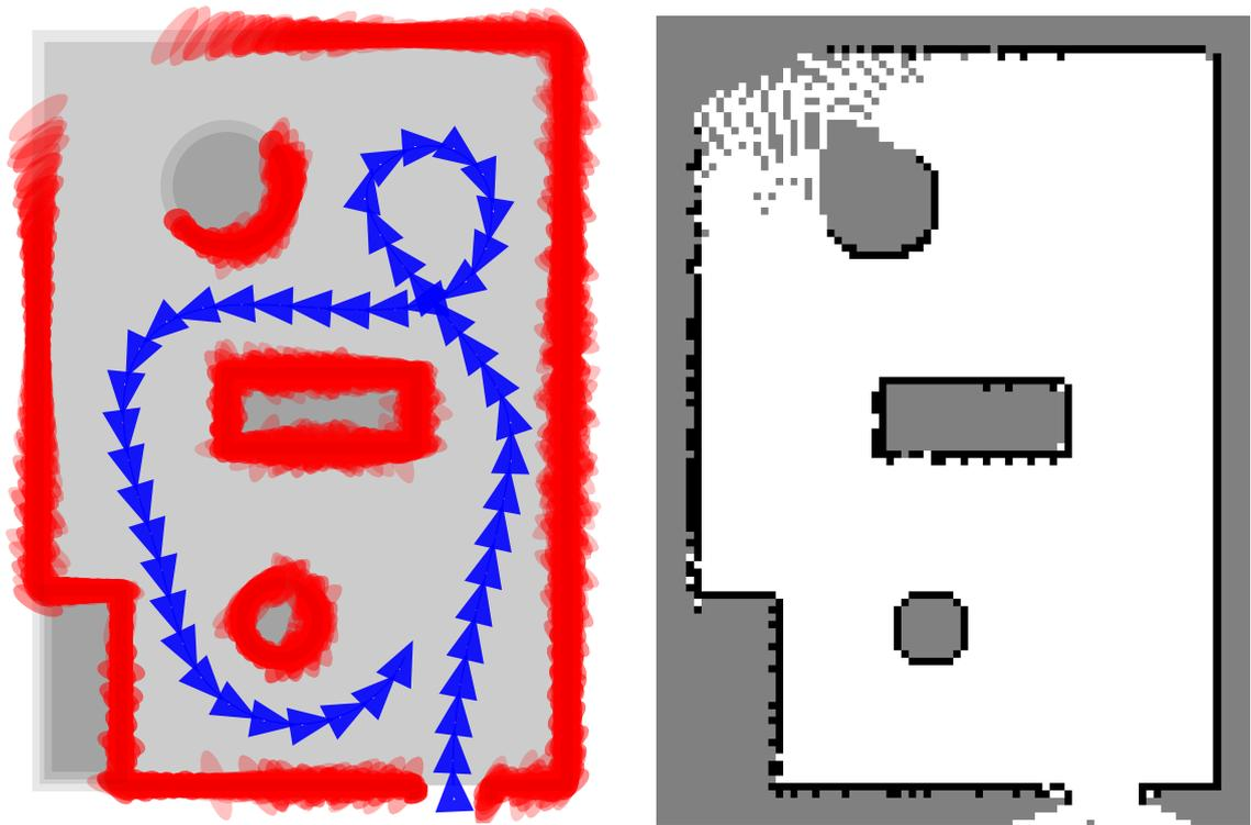
**Figure 2.7. Occupancy gridmap:** All lidar scans from the example problem, projected from exact poses. The door is visible at the bottom right, while an unmapped area remains at the top. **Left:** 2-D top view. **Right:** Occupancy gridmaps. For each grid cell  $m_i$ : **Gray:** Unknown  $p(m_i) = 0.5$ . **Black:** Occupied  $p(m_i) = 1$ . **White:** Free  $p(m_i) = 0$ .
