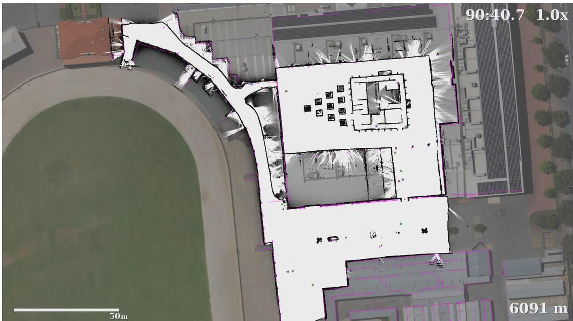
(e) **90m 40s:** Global gridmap with surveyed ground truth overlaid (magenta). The temporary structures inside the pavilion were not surveyed. Note: the dataset ended after 80 minutes. The RMS error calculated from 76 samples was  $\pm 0.62$  meters.
