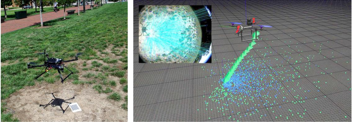
**Figure 2.15. Visual SLAM with a sliding window filter:** Visual SLAM on a quadrotor. **Left:** photo at take-off. **Right:** 3-D visualization with camera poses are shown as green pyramids, marginalized landmarks are blue dots, while currently estimated landmarks are shown in green. **Right Inset:** wide FOV camera view showing epipolar lines [111]. These images are from other research not included in this thesis.
