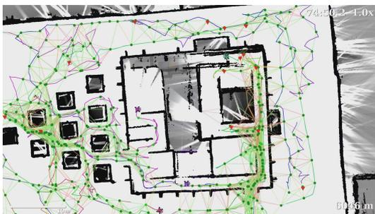
(c) **74m 50s:** The pavilion is 95% explored. The inner maze contained many  $15^\circ$  ramps that tested the UGVs' mobility.
