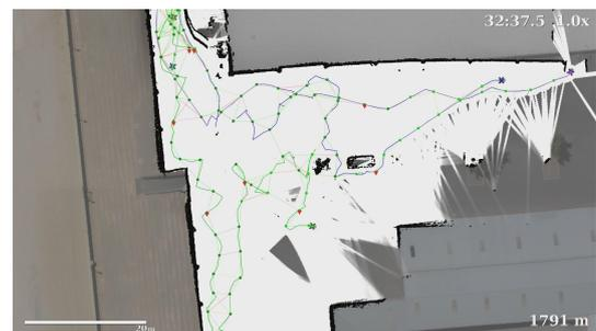
(c) **32m 37s:** The second UGV team explores the car park and finds the southern entrance. Odometry errors accumulate quickly in the sparse environment.
