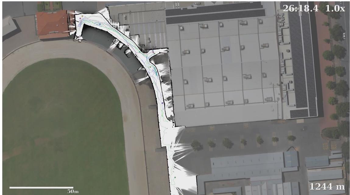
(a) **26m 18s:** The 14 UGVs start in the north-west corner and explore down the west edge of the phase. Large odometry errors occur in this alleyway. One team of UGVs assembles near the west door to the pavilion, a second team moves south into the open car park.
