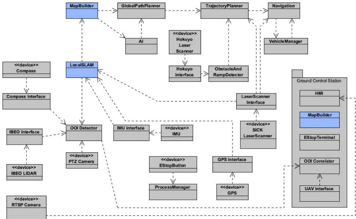
**Figure A.1. WAMbot MRS component diagram:** 16 software components and 9 device interfaces that ran on each UGV are shown. The components that ran on the GCS computer are inset on the right. The MR-SLAM components (Mapbuilder and Local SLAM) are highlighted in blue. UML diagram courtesy Adrian Boeing [64].
