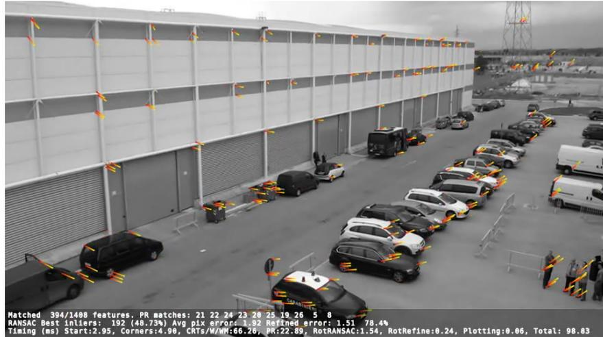
**Figure 2.11. Visual place recognition:** Visual odometry (VO) and visual place recognition (PR) from a flying quadrotor MAV. After completing a 200 meter loop, PR found 10 potential matches to previously seen images. Results from my unpublished research. Video courtesy Cybertech.
