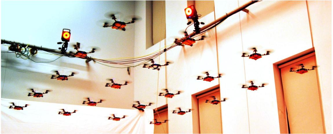
**Figure 1.5. MRS of quadrotors MAVs:** 20 nano quadrotor MAVs flying in a  $5 \times 4$  grid formation. Two of the cameras used for external localization can be seen mounted to the wall. Image courtesy of Alex Kushleyev and KMel Robotics.
