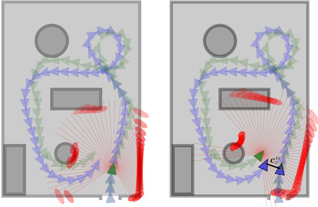
**Figure 2.18. Loop closure constraints:** A loop closure is found in the example problem. Blue triangles are the exact robot pose, green triangles are estimates, red ellipses are lidar measurements. **Left:**  $t = 3$ . **Right:**  $t = 49$ . After completing a loop of the room, a large amount of odometry noise has accumulated. Note the similarity between the two lidar scans (red): the loop closure constraint  $\mathbf{c}_3^{49}$  is the estimated transform required to align them.
