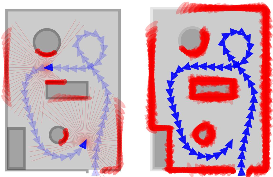
(a) Lidar scans from  $t = 30$  and  $t = 48$ . Laser pulses diverge, increasing the bearing uncertainty to more distant objects.
