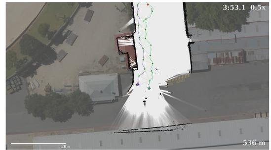
(b) **3m 53s:** Two UGVs reach the end of the wide alley. Significant perceptual aliasing prevents submap matching from correcting the odometry drift.
