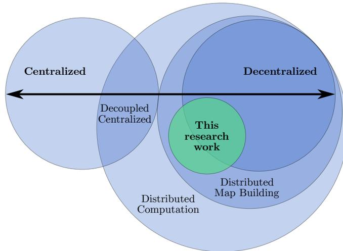
**Figure 3.1. MR-SLAM architectures:** Venn diagram showing different classes of MR-SLAM architectures spanning from centralized to decentralized. Not all architectures that distribute MR-SLAM computation are able to build distributed copies of the global map. For reference, the hybrid-decentralized architecture designed for my research provides fully distributed computation and map building. It is described in [Chapter 4](#), and shown here in green.
