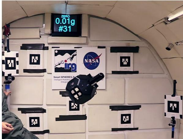
**Figure 2.12. Map-based localization using visual fiducials:** One of NASA’s SPHERES robots, [175], floating in a zero-g aircraft. ALVAR visual tags allow accurate on-board map-based localization [174]. Image courtesy NASA Ames and Google ATAP.
