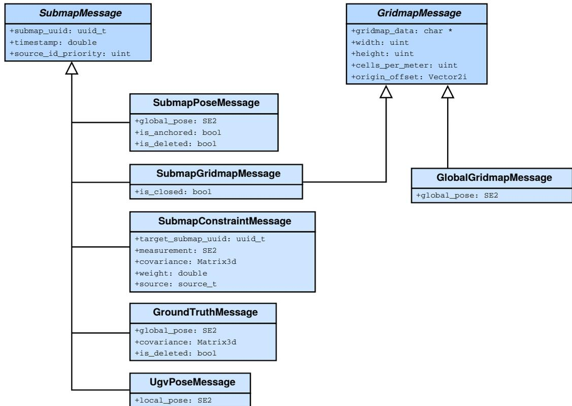
Figure 4.7. Mapbuilder message types: UML class diagram of demarshalled message types.
