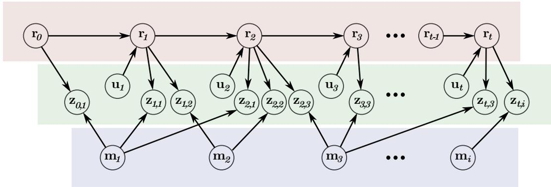
**Figure 2.13. Graphical model for landmark-based SLAM:** The red and blue boxes contain variables estimated in the SLAM state. The green box indicates measurements. Arrows indicate dependencies, or causal relationships. Robot pose estimates,  $\mathbf{r}_t$ , depend on the previous pose,  $\mathbf{r}_{t-1}$ , and odometry,  $\mathbf{u}_t$ . Map landmark estimates,  $\mathbf{m}_i$ , combined with the robot pose, cause the sensor measurement distributions  $\mathbf{z}_{t,i}$ .
