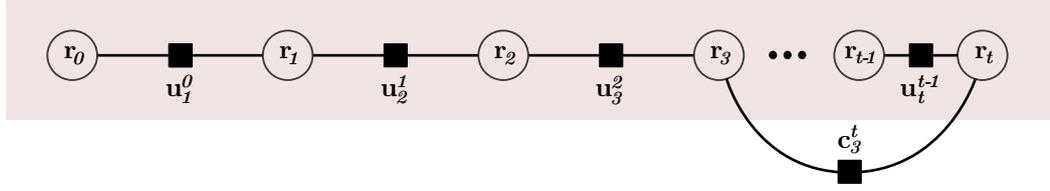
**Figure 2.17. Factor graph with a loop closure:** A pose-graph SLAM estimation problem where the robot poses,  $\mathbf{r}_t$ , are the variable nodes, separated by either odometry factors,  $\mathbf{u}_t$ , or loop closure factors,  $\mathbf{c}_k^j$ . A typical pose graph has many more loop closures.
