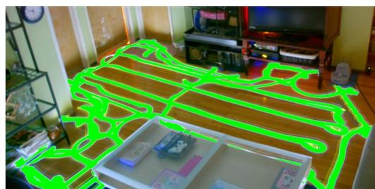
(b) The Neato XV-11 navigates using SLAM, which allows it to vacuum more efficiently.
