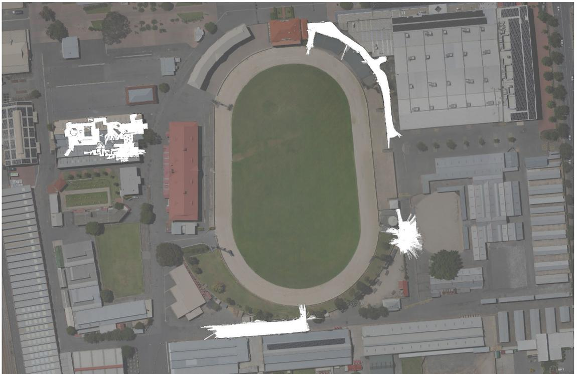
**Figure 7.2. WAMbot challenge day results:** Occupancy gridmaps superimposed on aerial imagery. Due to a combination of hardware and software issues, described in [64], our UGVs only explored 15%, 8% and 5% of the three phases. WAMbot performed considerably better in the Old Ram Shed Challenge (ORSC) on the left, exploring 83%. Aerial imagery courtesy DSTO.
