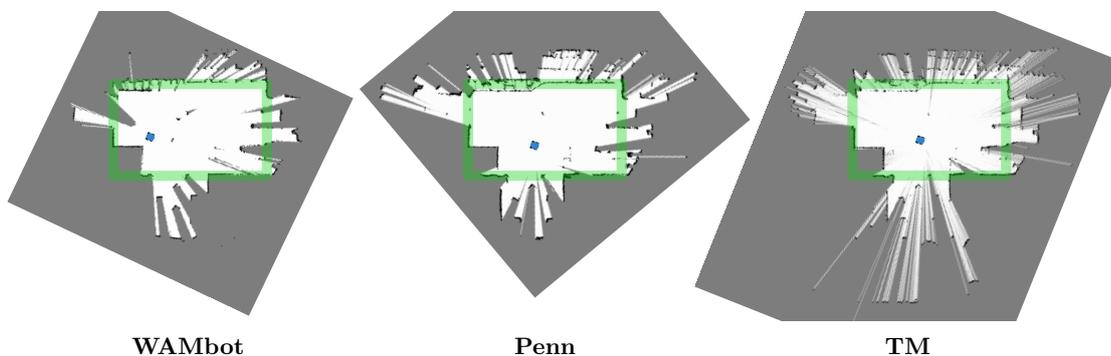
**Figure 7.27. Sample submaps:** Captured from the three different UGVs around the same location in the Old Ram Shed Challenge (ORSC). For reference, the  $20 \times 12$  meter boundary of first room is highlighted in green.
