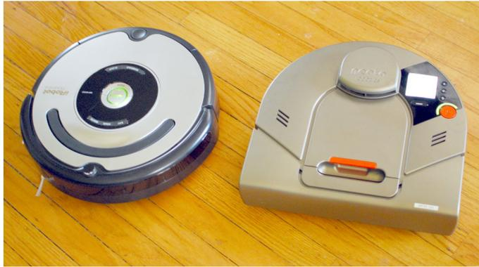
**Figure 1.2. Two mobile robot vacuum cleaners:** The iRobot Roomba 560 (left) and the Neato XV-11 (right). Image courtesy of Evan Ackerman, IEEE Spectrum.
