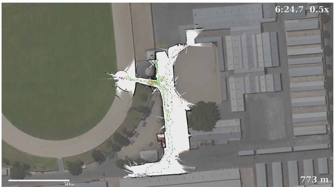
(c) **6m 24s:** Mapbuilder aligns the submaps at the end of the alley as additional submap matches are made. The UGVs explore the phase on five separate frontiers.
