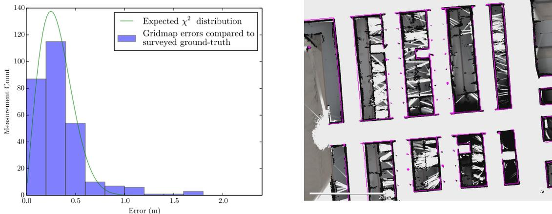
(a) Histogram of map errors between Mapbuilder’s global gridmaps and the surveyed ground-truth. Errors measurements were spatially distributed using a grid. The  $\chi^2(2)$  distribution is shown for  $\sigma=0.25$  m.
