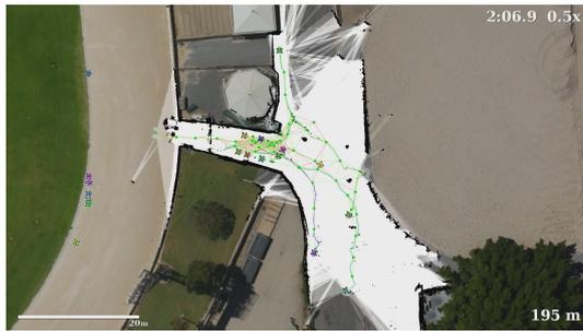
(a) **2m 6s:** Initial global localization: 12 of 23 UGVs are connected in the pose graph. Odometry errors are already visible in the 20 m wide alley to the south.
