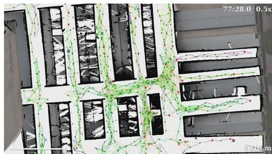
(d) **77m 28s:** The density of nodes in the pose graph indicates the stables have been mapped thoroughly. The UGVs explore the corridors to the east.
