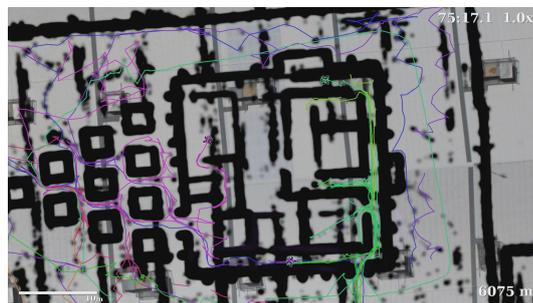
(d) **75m 17s:** Alternate "x-ray" view showing roof beams and clutter that is successfully filtered in the regular gridmaps.
