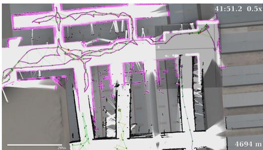
(c) **41m 51s:** One UGV (magenta) has explored the north horse stables. Several meters of drift is corrected to enable five loop closures, the first and largest is 330 m.
