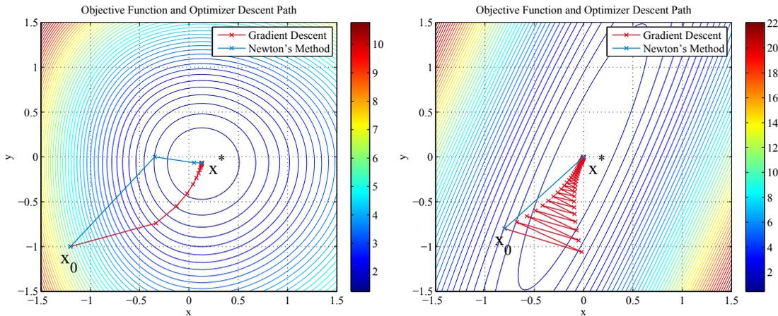
**Figure 2.20. Convergence properties:** Convergence for different optimization algorithms varies depending on the shape of the cost function. Here gradient descent and Newton’s method are compared for a 2-D cost function  $\|\mathbf{x}\|_{\Sigma}^2$ . Both circular (left) and ellipsoidal covariances (right) are common in pose graphs. Gradient descent converges slowly, and while Newton’s method converges quicker, it may get stuck at saddle points [234]. Figure courtesy Niko Sünderhauf [244].
