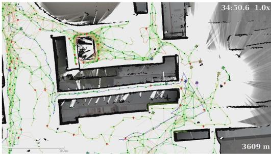
(a) **34m 50s:** 10 UGVs converge in the Red Square (right) before closing a 210 m loop. The map distortions indicate that about 1 m of drift is corrected by the closure.
