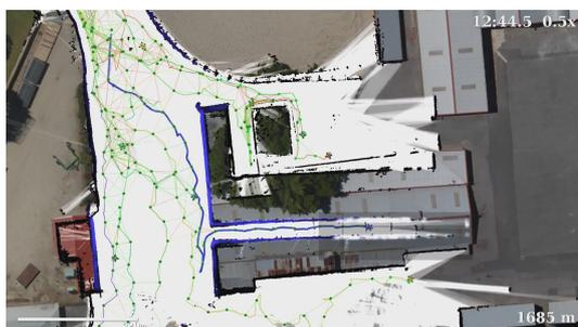
(d) **12m 44s:** Three teams explore frontiers towards the east. UGV number 16 (blue) accumulates odometry errors in a narrow corridor and its path is adjusted.
