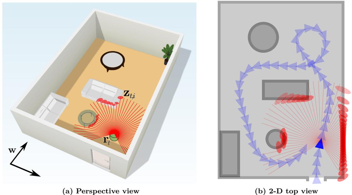
**Figure 2.1. Example problem:** A robotic vacuum cleaner drives around a room containing two couches and two tables. In (a) measurements  $\mathbf{z}_{t,i}$  from a lidar scanner are shown extending from the robot in red. Each lidar return measures the mean range to the objects overlapped by the corresponding red ellipse. In (b) the robot's exact path is shown in blue. The lidar measurements  $\mathbf{z}_{4,i}$ , from  $t = 4$ , are shown in red.
