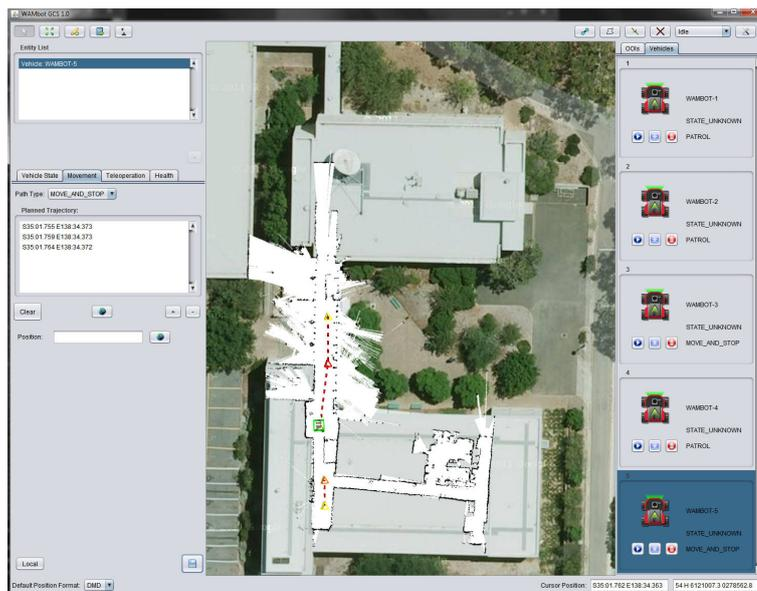
**Figure A.3. WAMbot HMI:** Screen shot taken during testing at Flinders University in Adelaide. The Mapbuilder occupancy gridmap is overlaid on an aerial image. Taken during debugging, an invalid constraint has caused the bottom part of the gridmap to be slightly misaligned.
