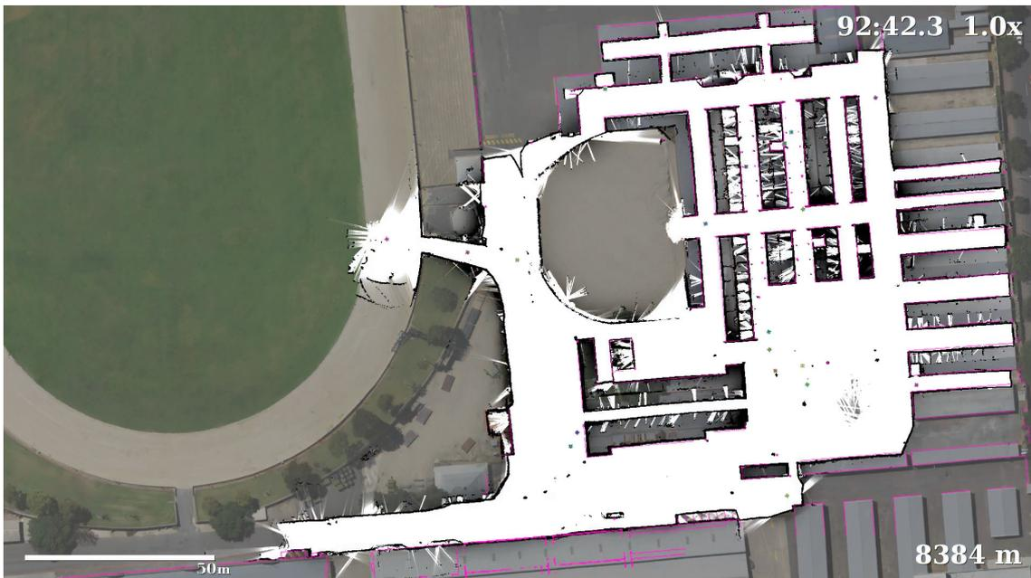
(e) **92m 42s:** Global gridmap with surveyed ground truth overlaid (magenta). Small colored marks in the white (free) areas are UGVs, while many black marks are round barrels used to support infrastructure. The RMS error calculated from 100 samples was  $\pm 0.35$  meters.
