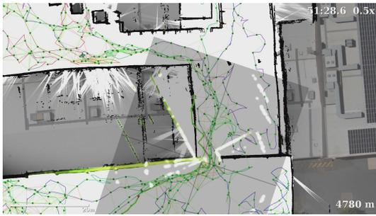
(a) **51m 28s:** Odometry errors while entering the southern doorway. One of many instances where the submap gridmaps were corrupted (white ghosting).
