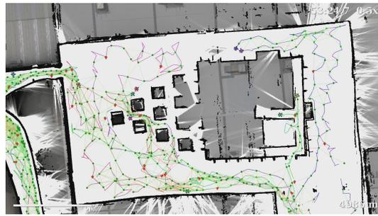
(b) **53m 24s:** The second largest loop closure on the northern edge of the pavilion. Additional ground truths were required to resolve the perceptual aliasing.
