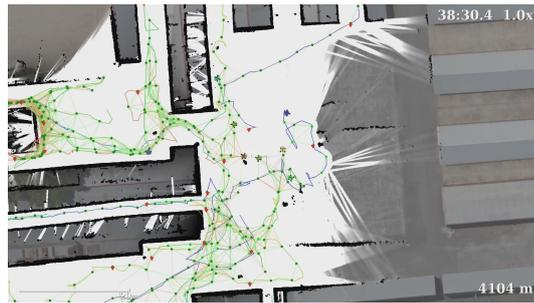
(b) **38m 30s:** After the loop closure the UGV's explore north into the stables. Red Square is larger than the lidar sensors range and uncorrected odometry errors result.
