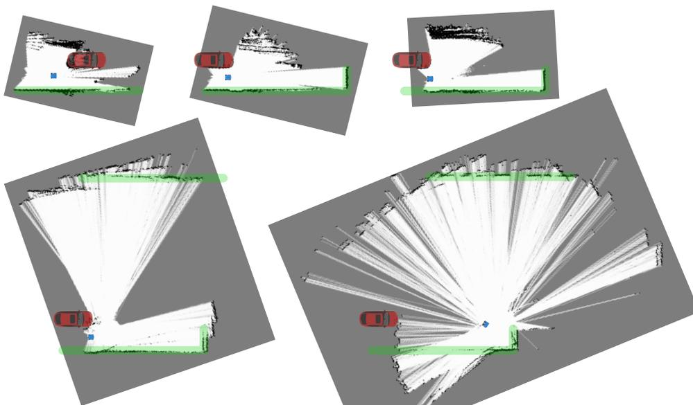
**Figure B.6. Phase 2 South Boulevard:** Corrupted submaps from a 20 meter wide alley where wheel slippage consistently occurred in a drain. Both TM and Penn’s SLAM front-ends produced unusable submaps. **Blue:** UGV. **Red:** Graphic where car was parked. **Green:** Nearby walls.
