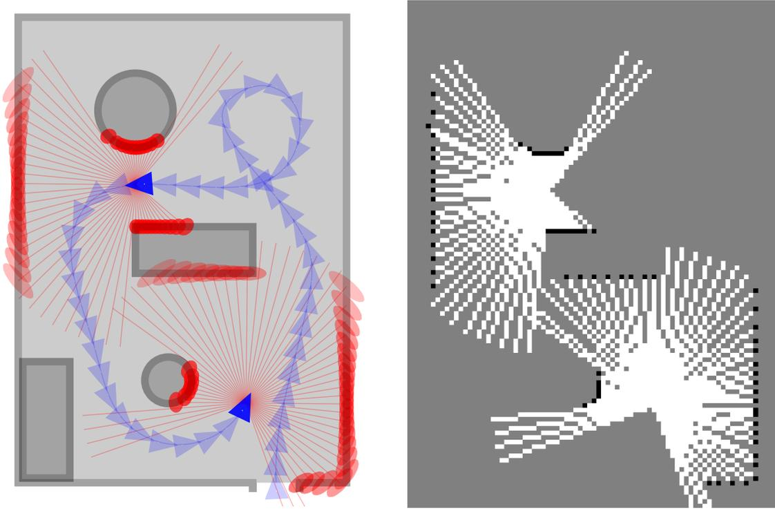
**Figure 2.6. Occupancy gridmap:** Two lidar scans from the example problem, at  $t = 30$  and  $t = 48$ , projected from exact robot poses (no odometry noise). **Left:** 2-D top view. **Right:** Occupancy gridmaps with two lidar scans fused. For each grid cell  $m_i$ : **Gray:** Unknown  $p(m_i) = 0.5$ . **Black:** Occupied  $p(m_i) = 1$ . **White:** Free  $p(m_i) = 0$ .
