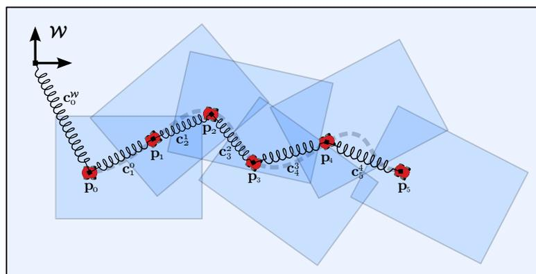
**Figure 4.3. Submap constraints:** Constraints are analogous to mechanical springs that connect pairs of submaps. During optimization they slide and rotate each submap's pose,  $\mathbf{p}_a^W$ , until all forces and torques balance. This pose graph has a single ground-truth constraint,  $\mathbf{c}_0^W$ , which locates the first submap in the world frame. The five subsequent submaps have their positions determined by the relative constraints  $\mathbf{c}_i^a$ .
