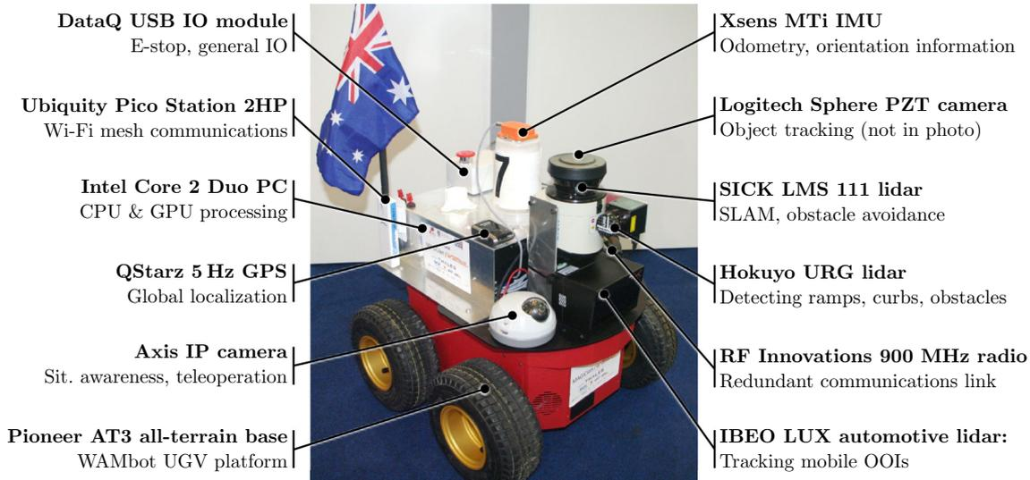
**Figure A.4. WAMbot UGVs:** The WAMbot hardware design integrated many COTS components.
