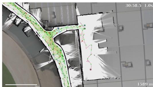
(b) **30m 58s:** The first team enters the pavilion. With limited submap overlap ground-truth constraints are required to align the inside and outside walls.
