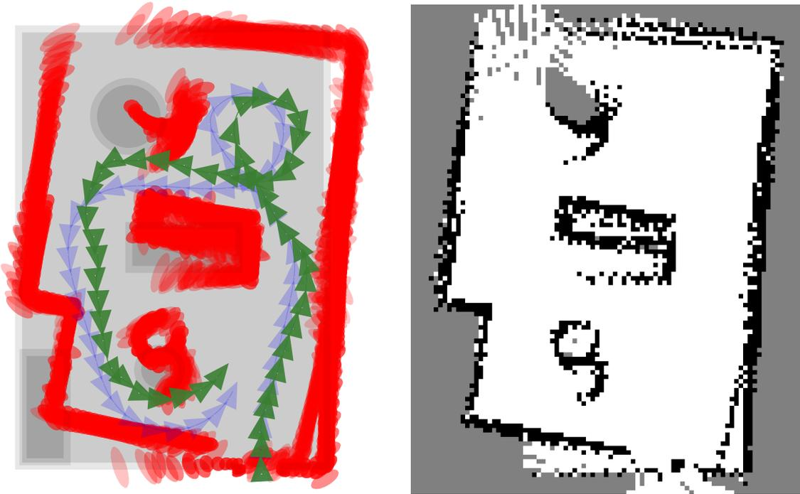
**Figure 2.8. Occupancy gridmap:** All lidar scans from the example problem projected from odometry estimates accumulated with noise. **Left:** 2-D top view showing lidar measurements superimposed. Blue: the robot's true path. Green: the robot's noisy path based on odometry. **Right:** In the corresponding gridmap the structure of the environment can be discerned, however large misalignments are visible.
