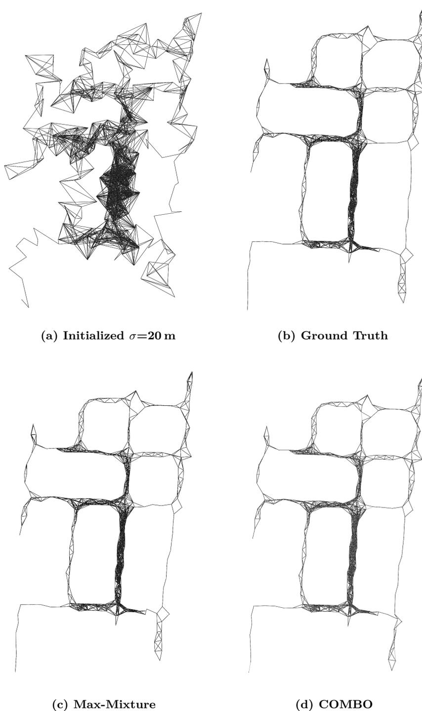
**Figure 7.23. Results: Pose graphs for Manhattan Small dataset.** A three block (315 meters) wide subset of the Manhattan dataset with 7,400 meters of odometry. The pose graph constraints are shown in black. (a) The  $\text{SE}(2)$  pose graph is initialized by perturbing with Gaussian noise ( $\sigma=20$  m). (b) Ground truth used in RMSE calculations. The pose graphs (c) and (d) both converge to almost identical solutions.
