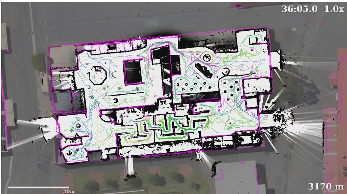
(e) **36m 5s (end)**: Global gridmap with surveyed ground truth overlaid (magenta). Note: many temporary barriers were not surveyed, including the straw hay bale “maze”. The RMS error calculated from 88 samples was  $\pm 0.27$  meters.
