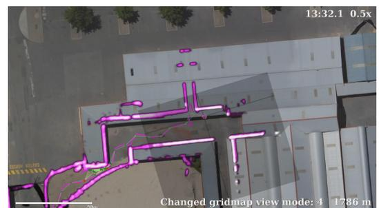
(e) **13m 32s:** UGV number 18 (magenta) explores through the horse stables. The “x-ray” view is used to align its gridmap to the building eaves in the aerial imagery.
