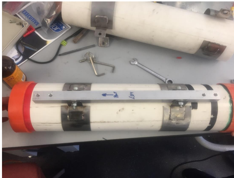
Figure 11: Final small battery tube mounting system
