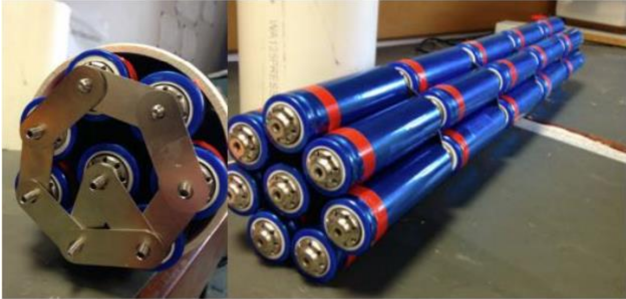
Figure 3: Battery cells before installation in PVC pipe
