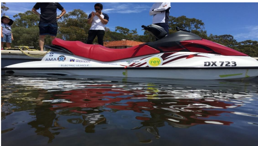
Figure 14 Back heavy LKG as seen in water.
