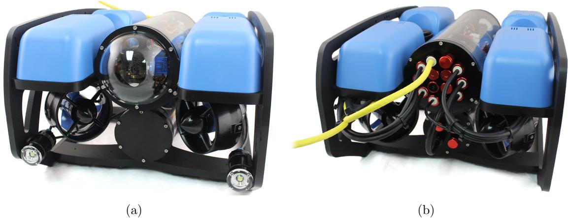
Figure 4.1: Blue Robotics' BlueROV2. (a) front view, (b) back view. Figure source: [59]
