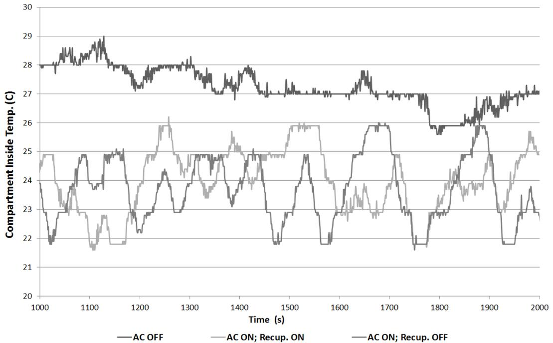
Figure 4-11 EV passenger compartment temperature fluctuations over 16 minutes of a test drive
