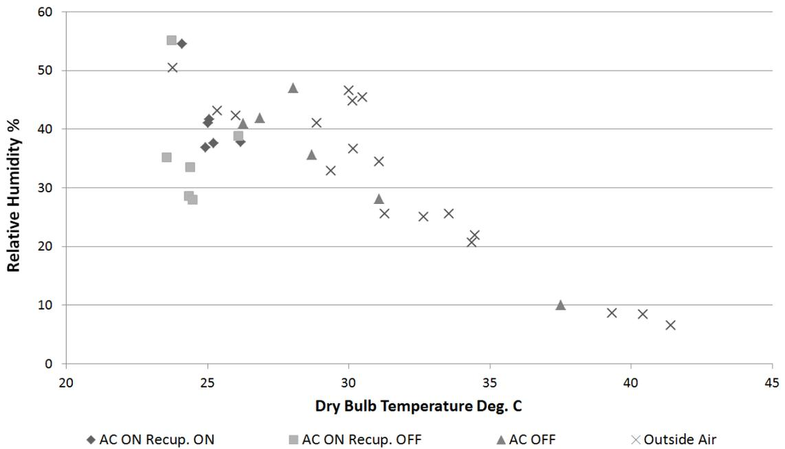
Figure 4-12 Outside air and passenger compartment mean temperatures and humidity over the six test days under different driving configurations
