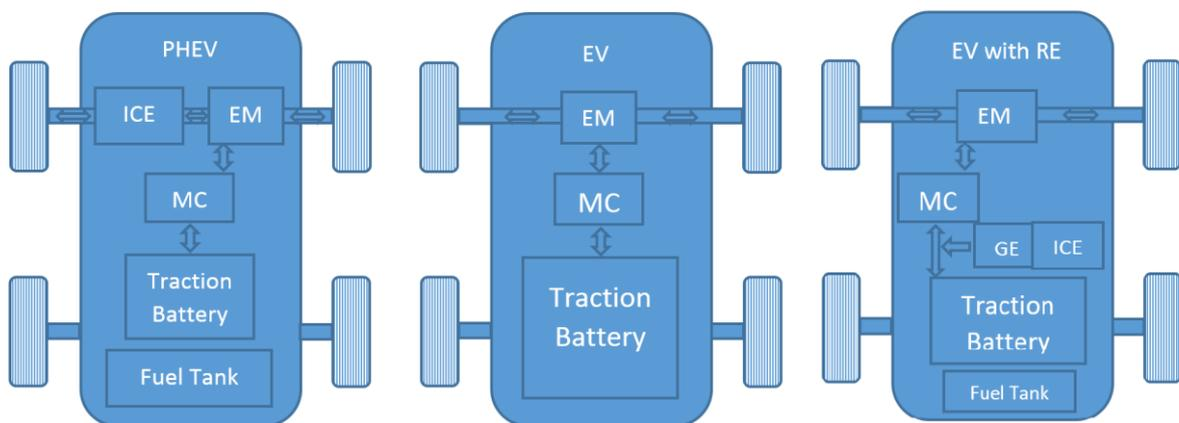
Figure 2-1: A block diagram describing the power trains of a plug-in hybrid vehicle (PHEV), full electric vehicle (EV) and EV with range extender (EV with RE)
