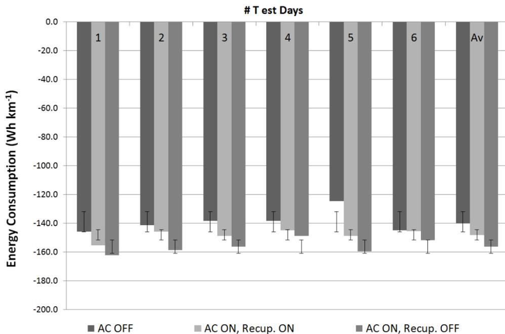
Figure 4-8 The Ford Focus EV average energy consumption over the six testing days and the overall average (in  $\text{Wh km}^{-1}$ ) with standard deviation error bars
