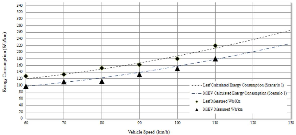
Figure 7-2 Measured and extrapolated energy consumption over a speed range of 60 to 130 km/h.
