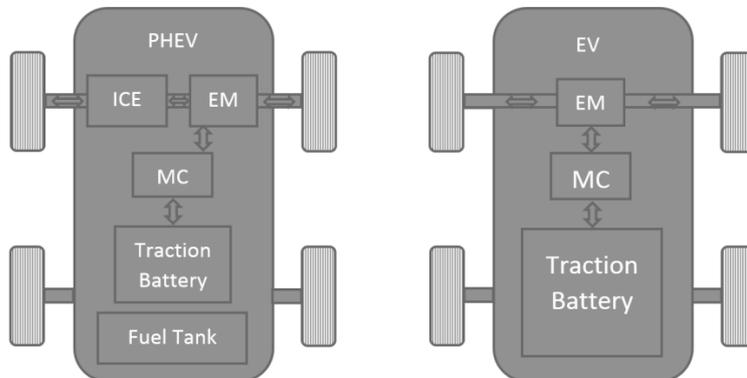
Figure 5-1: A basic block diagram of a power train of a PHEV and EV
