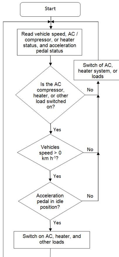
Figure 4-6 A flow chart of the control strategy for the modified AC control system
