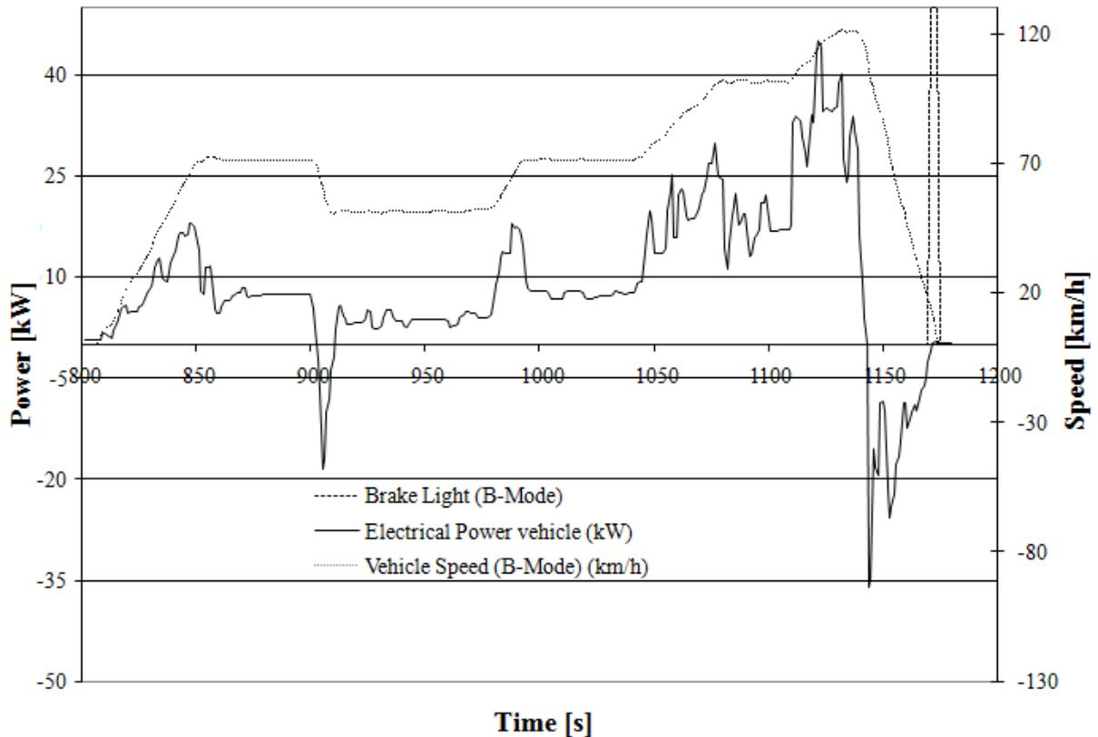
Figure 3-9: The NEDC Highway section speed profile, traction, regeneration power and the short period of the friction brake (brake light) in use below  $16 \text{ km h}^{-1}$  near the end of the highway section.
