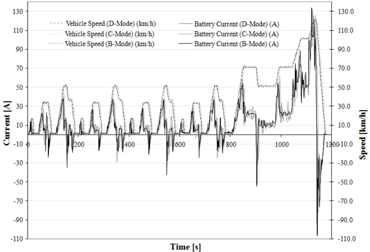
Figure 3-8: i-MiEV speed and current profile during three NEDC drive cycles for modes C, B, and D.
