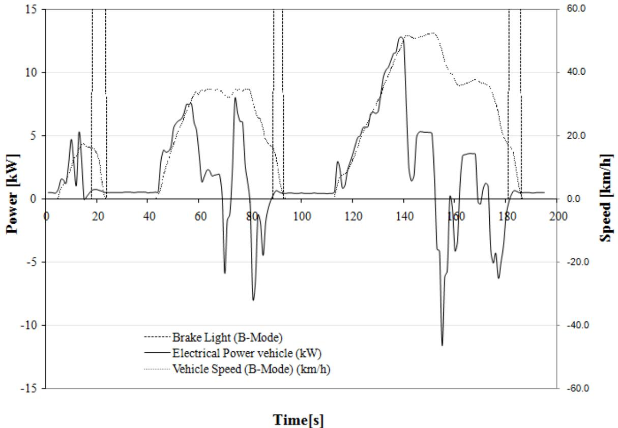
Figure 3-5: NEDC city driving cycle indicating the end of regenerating electrical power at the point when the RBS is disabled below its threshold of  $16 \text{ km h}^{-1}$  and the friction brake becomes active (brake light)
