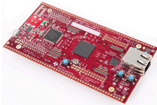
Figure 4 The new controller, Texas Instrument Hercules Launchpad (LAUNCHXL2-570LC43). Available [online]:
