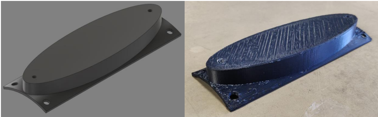
Figure 11 Left: 3D model of first motor mount design. Right: 3D printed model of first motor mount design
