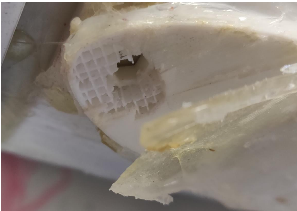
Figure 10: Close-up of damaged SPAR motor mount
