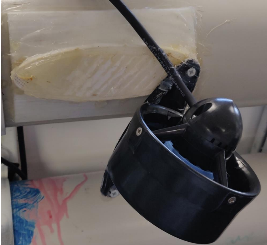
Figure 9: Damaged SPAR motor mount
