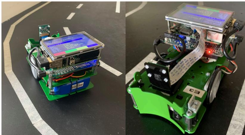
Figure 3: SoccerBot mobile driving robot
