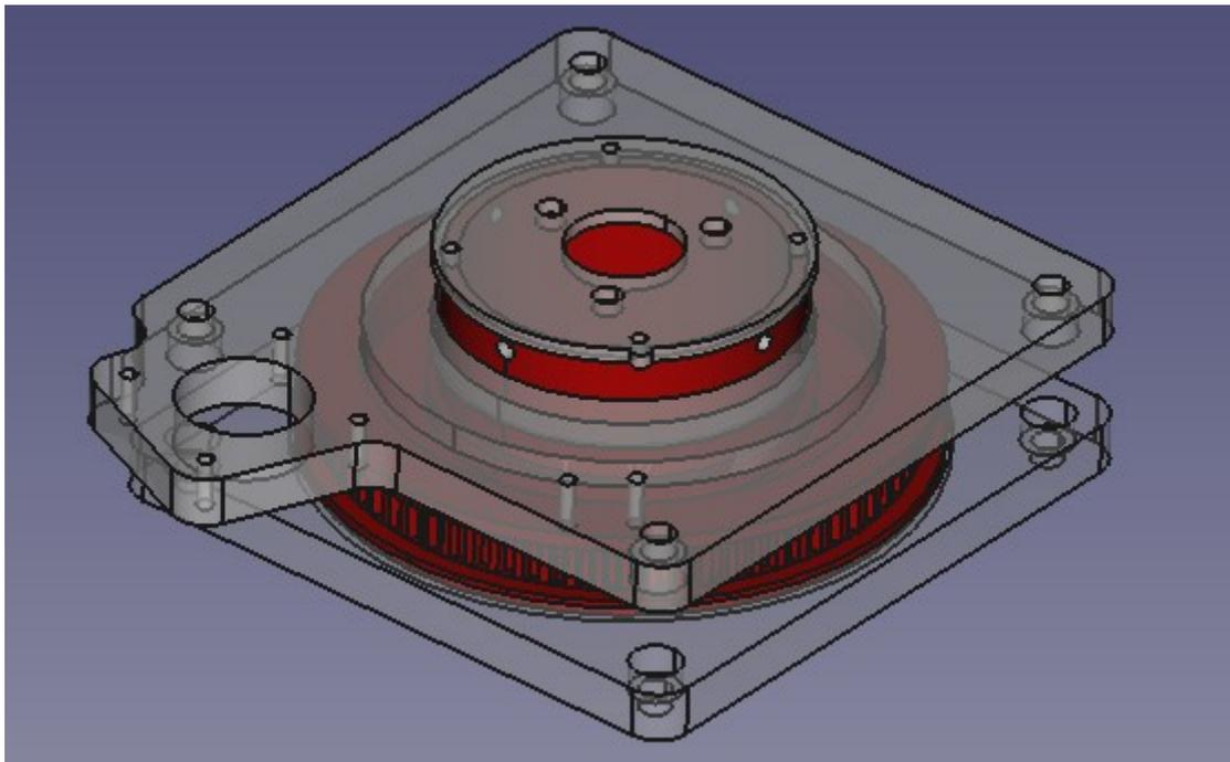
*Illustration 10: Above deck belt-driven steering gear design*
