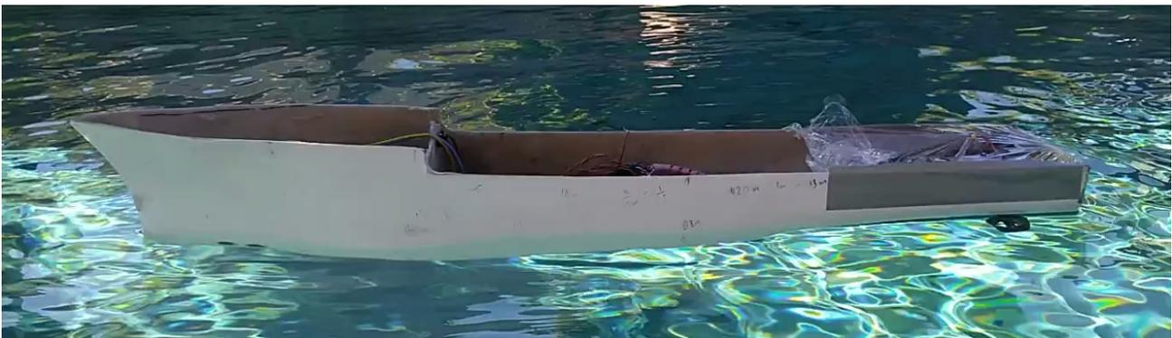
*Illustration 16: In-water test of the control equations on the OSV model*
