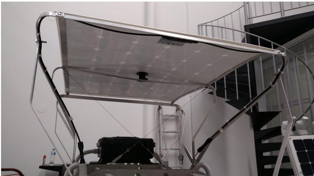
*Illustration 13: Awning structure, showing the cross cable shrouds and turnbuckles*
