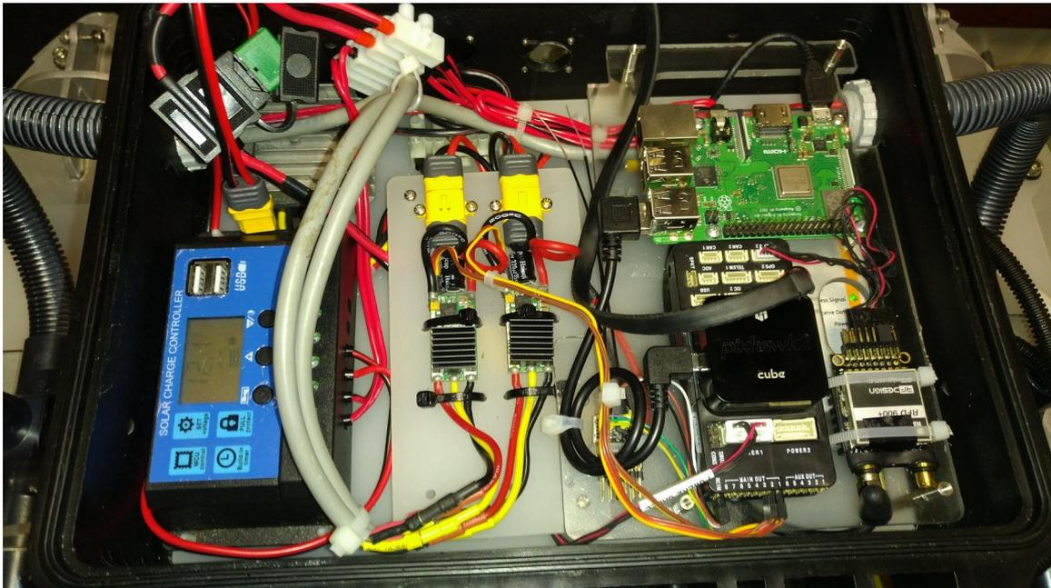
*Illustration 12: Internals of the control box, with electronics mounted on acrylic plates*
