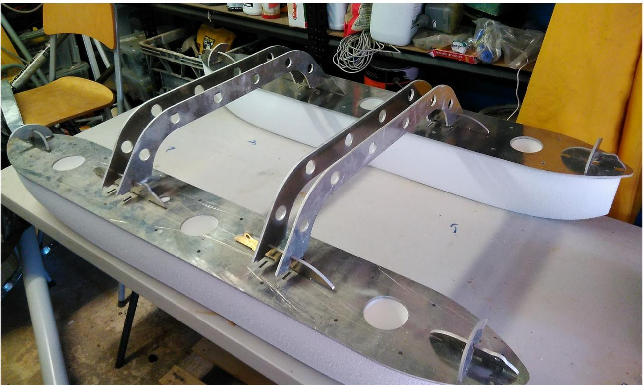
*Illustration 7: Structural bridge - raw CNC cut plates pre-assembly*
