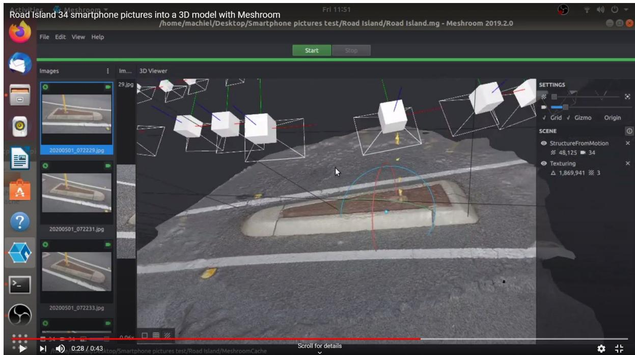
Figure 3.13, A very detailed Road Island after about 20 minutes of rendering in Meshroom with 30+ smartphone pictures, (Machiel van der Stelt, 2020).
