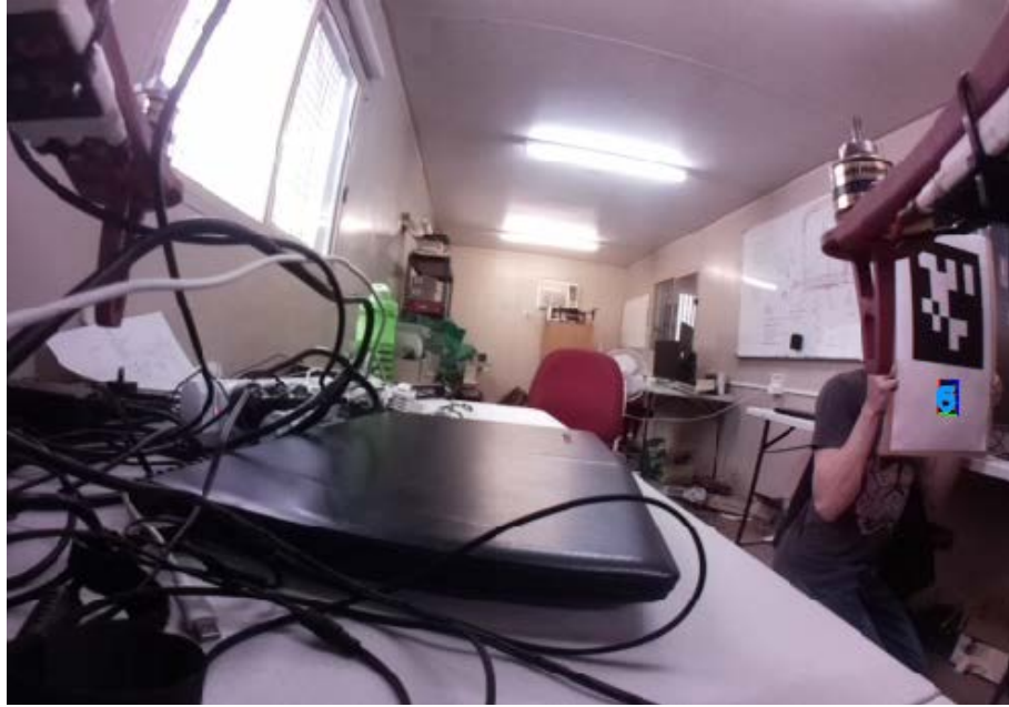
FIGURE 7: APRILTAG BEING DETECTED NEAR EDGE OF FOV OF FISHEYE LENSED CAMERA
