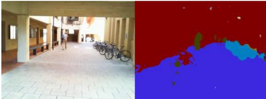
Fig. 4.12 SegNet output showing segmented pedestrian (olive), bicycles (light blue), pathway (blue) and building (red).
