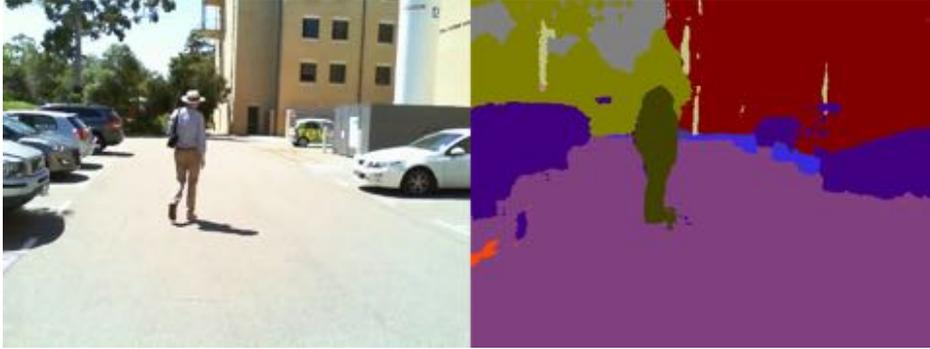
Fig. 5.8 Segmentation results from a parking area on campus grounds.
