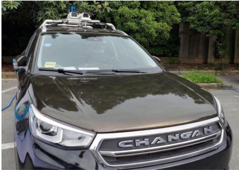
Fig. 1.2 An autonomous car with its sensors visibly mounted on its roof.
