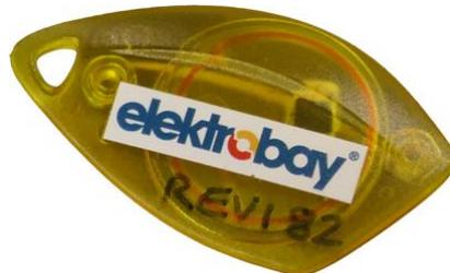
Fig. 9.10 An RFID token used for our AC charging station network. Pictured here is the tag for the User ID REV182.
