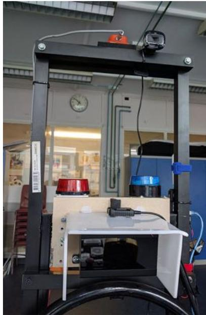
Fig. 5.1 The camera is mounted above the LiDAR system from [291], beside the IMU.
