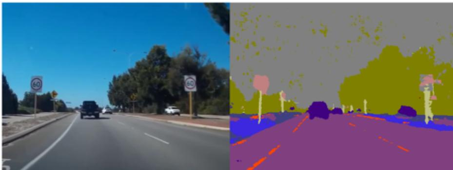
Fig. 2.4 SegNet's input (left) and output (right) for a typical Western Australian road scene.
