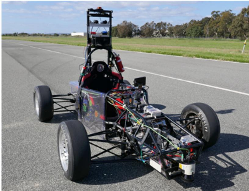
Fig. 7.1 Autonomous SAE Vehicle.
