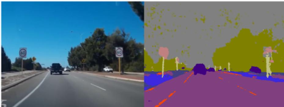
Fig. 5.7 SegNet's input (left) and output (right) for a dual carriageway in the Perth metro area.
