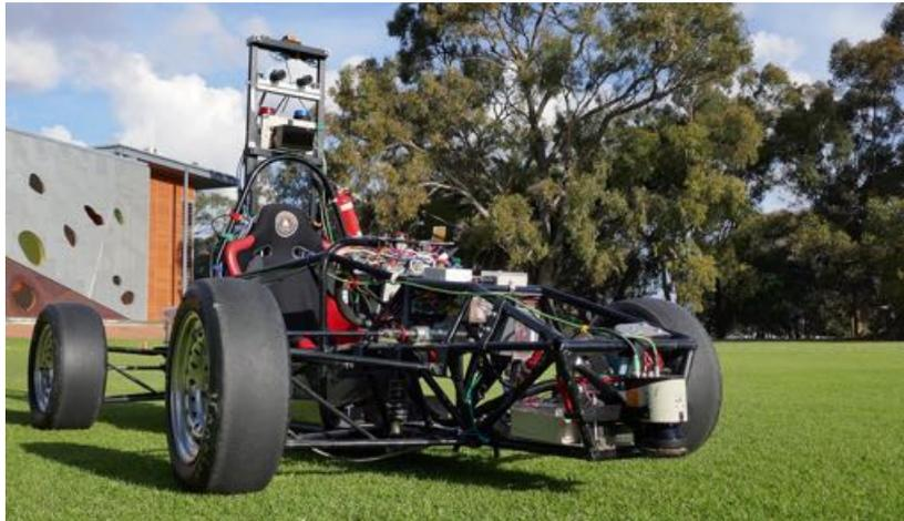
Fig. 1.4 The REV Project's autonomous Formula SAE Electric test vehicle.
