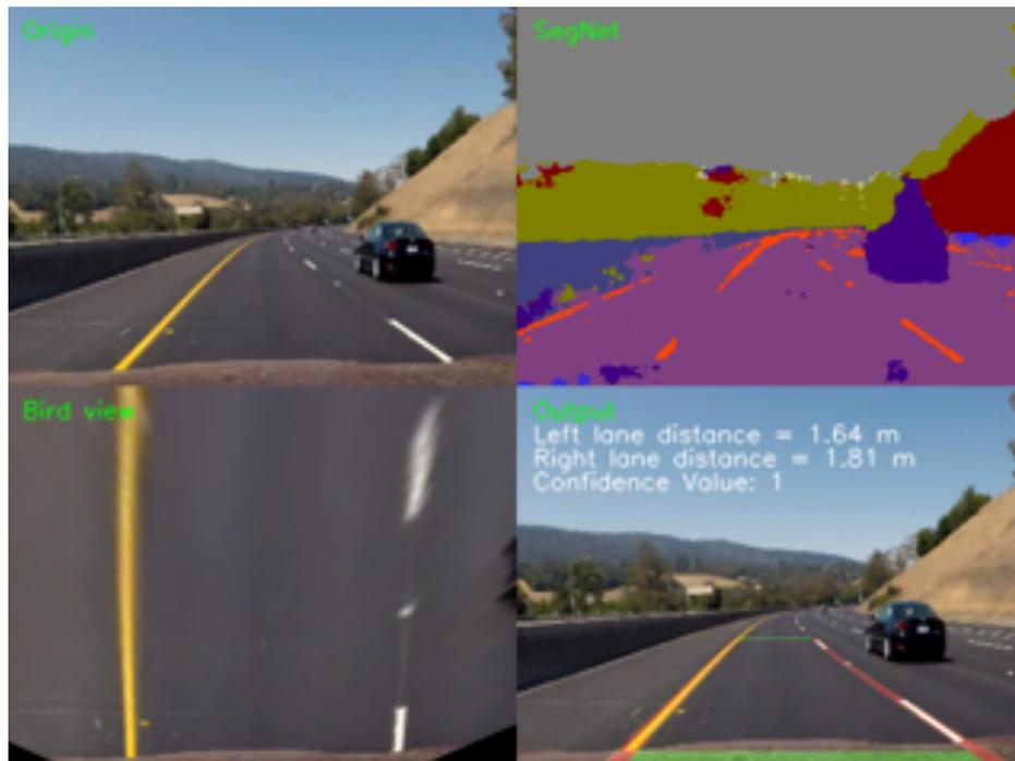
Fig. 6.7 Original and Jetson TX1 output showing segmentation, bird's eye view, vehicle distance to left and right lane marks.
