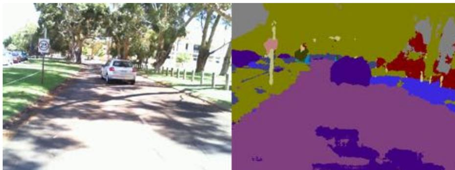
Fig. 5.13 Segmentation results on a road with pronounced shadows.
