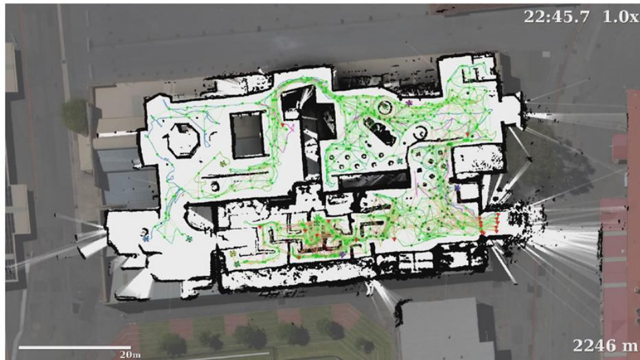
Fig. 4.7 SLAM output showing loop closure between both teams, with the first team about to exit via the southwestern corner.
