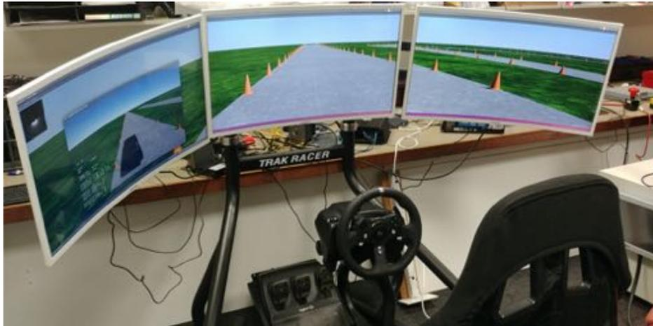
Fig. 8.5 Autonomous driving simulator setup.
