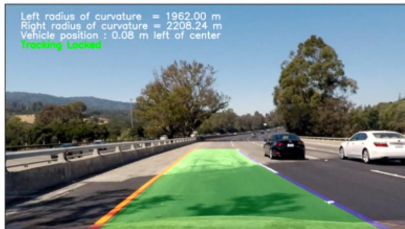
Fig. 2.6 The Self-Driving Car Nanodegree's Term 1, Project 4 output. Reprinted with permission from [140].
