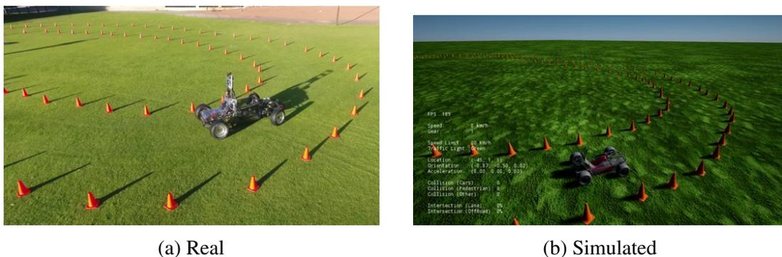
Fig. 8.1 Track setup used for comparing real (a) and simulated (b) LiDAR and visual cone processing outputs.
