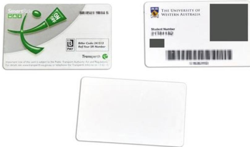
Fig. 9.4 RFID cards supported by the DC station. Pictured are a Transperth Smart-Rider card, a UWA Student ID and a general issue MIFARE RFID card, commonly used by station users.
