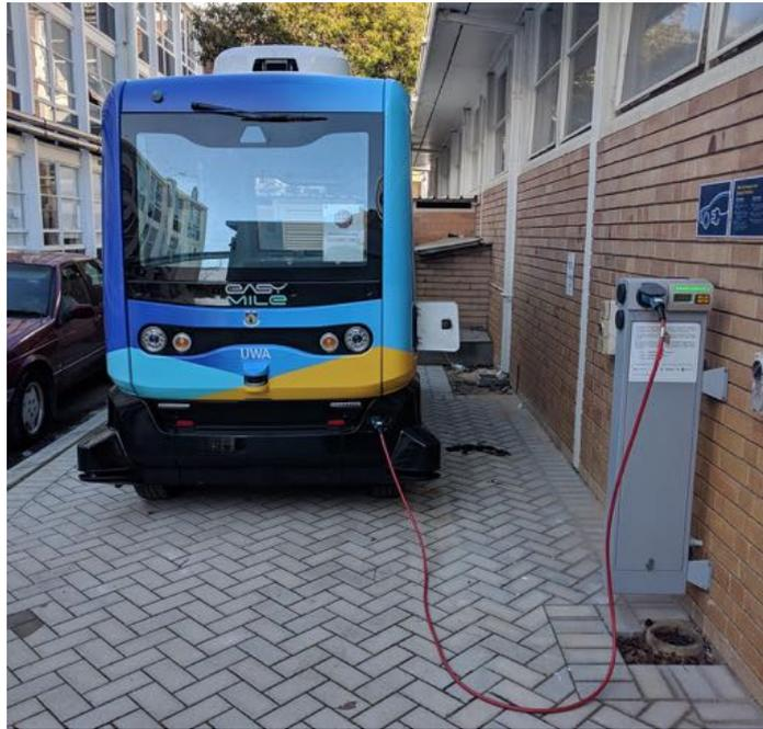
Fig. 1.1 An EasyMile EZ10 driverless shuttle at a UWA charging station.
