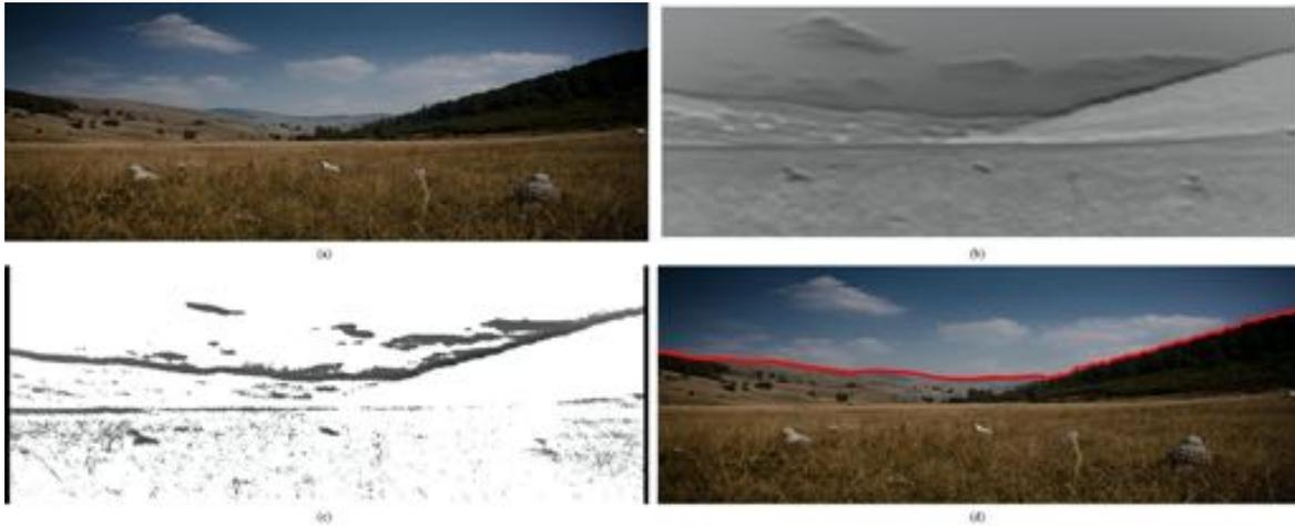
Fig. 2.1 An edge-less horizon detection algorithm generates a dense classifier score image (DCSI) (b) from a query image (a) using trained classifiers, where a threshold is then applied (c) before it plots the horizon line (d). Reprinted with permission from [58]
