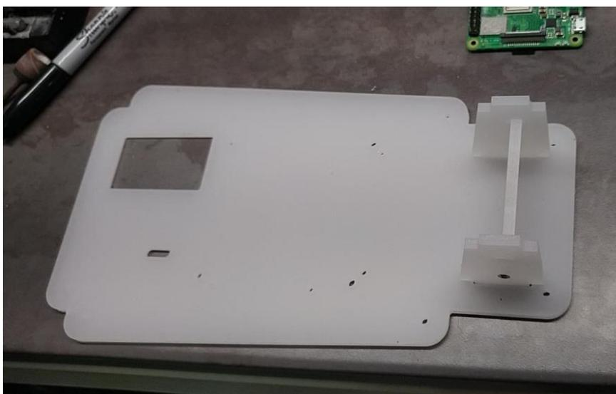
Figure 10: CNC Produced Mounting Plate
