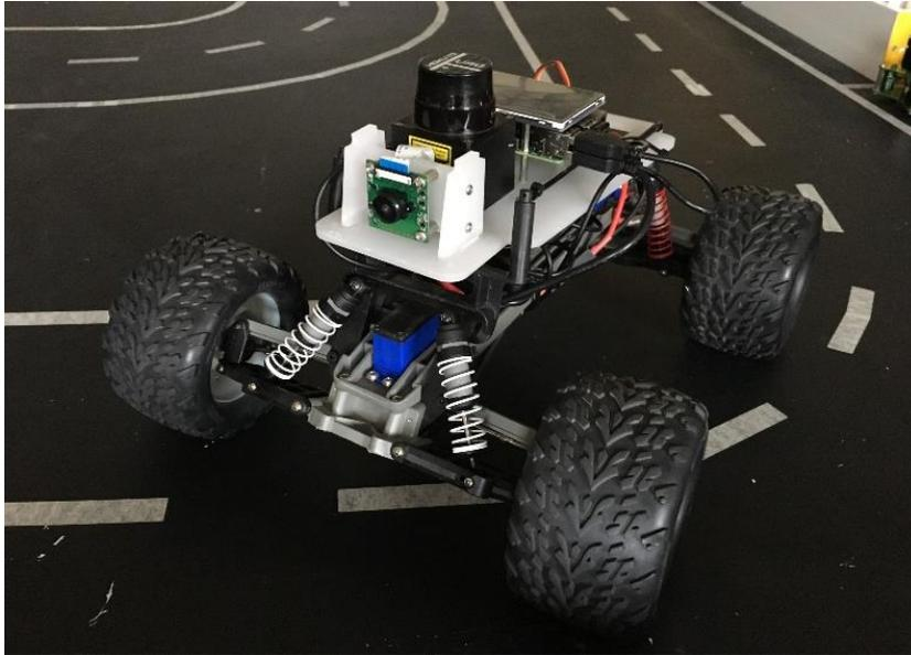
Figure 11: ModelCar-2 Autonomous Driving Robot
