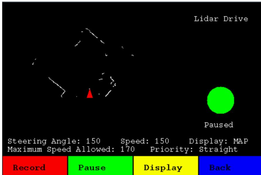
Figure 16: LIDAR Drive Point Map Display Mode
