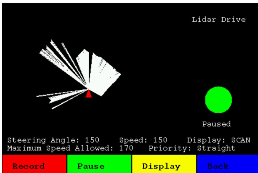
Figure 15: LIDAR Drive Scan Display Mode
