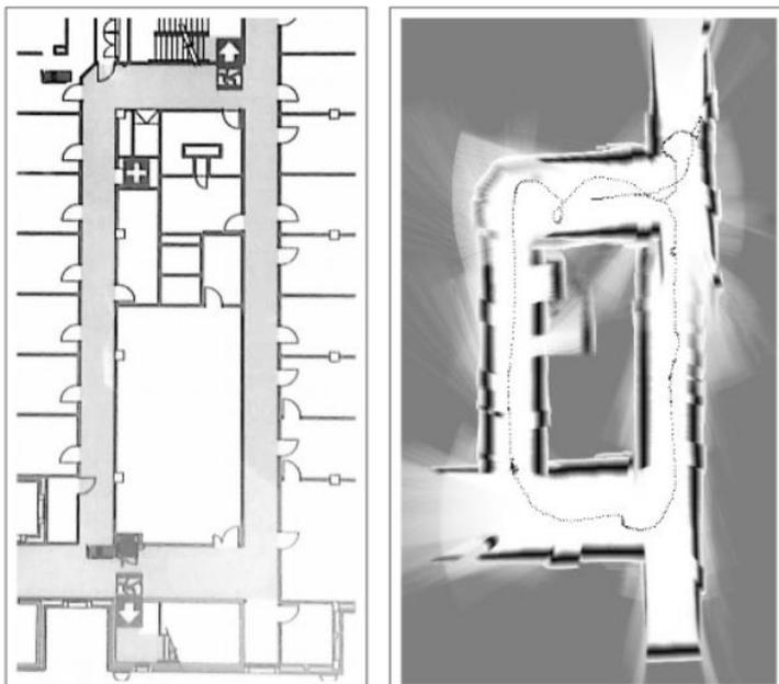
Figure 28: LIDAR SLAM Map of EECE 4th Floor UWA [3]
