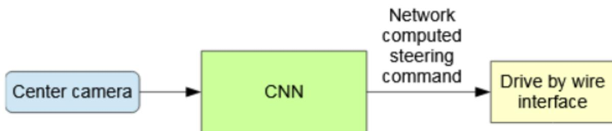
Figure 1: NVIDIA DAVE-2 End-to-End Driving Pipeline [1]
