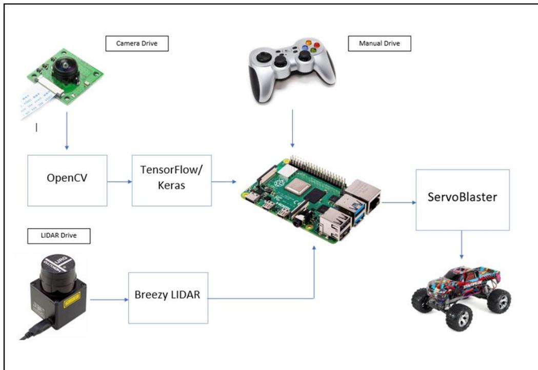
Figure 17: Simplified Control Flow for ModelCar-2
