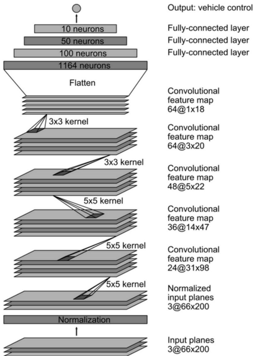
Figure 2: NVIDIA PilotNet Architecture [1]
