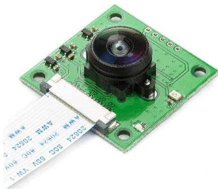
Figure 6: 5MP OV5647 Digital Camera
