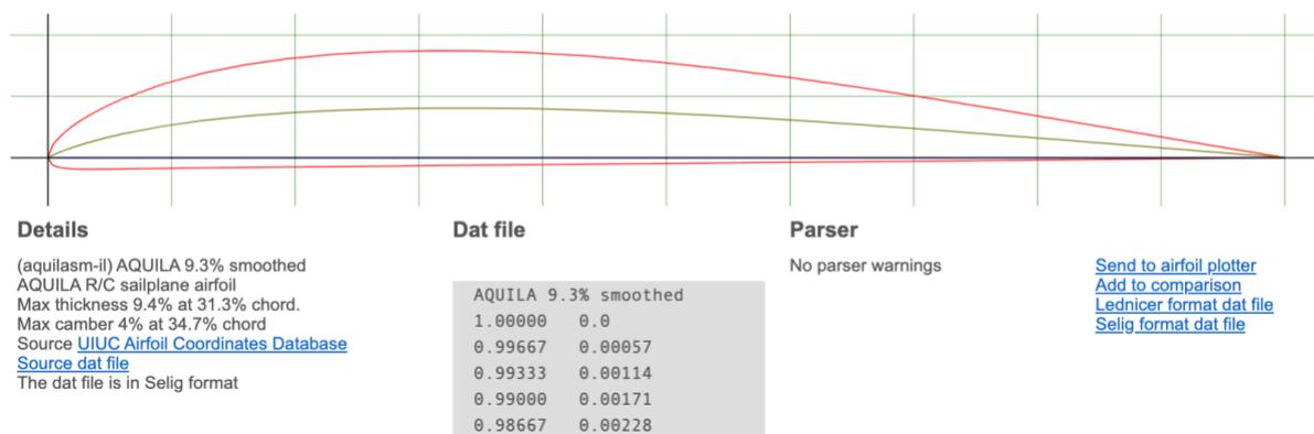
Figure 11: Ei-Foil Aquila 9.3 hydrofoil profile [33]
