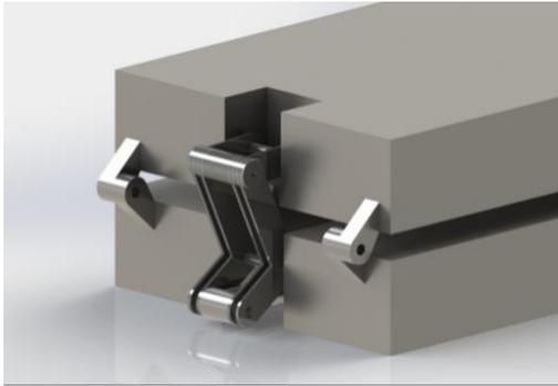
Figure 20: 180 degree scissor mechanism folded [48]
