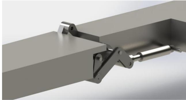
Figure 21: 180 degree scissor mechanism extended half view [48]
