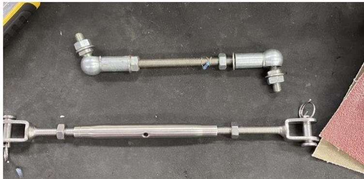
Figure 33: Turn Buckle Mechanisms
