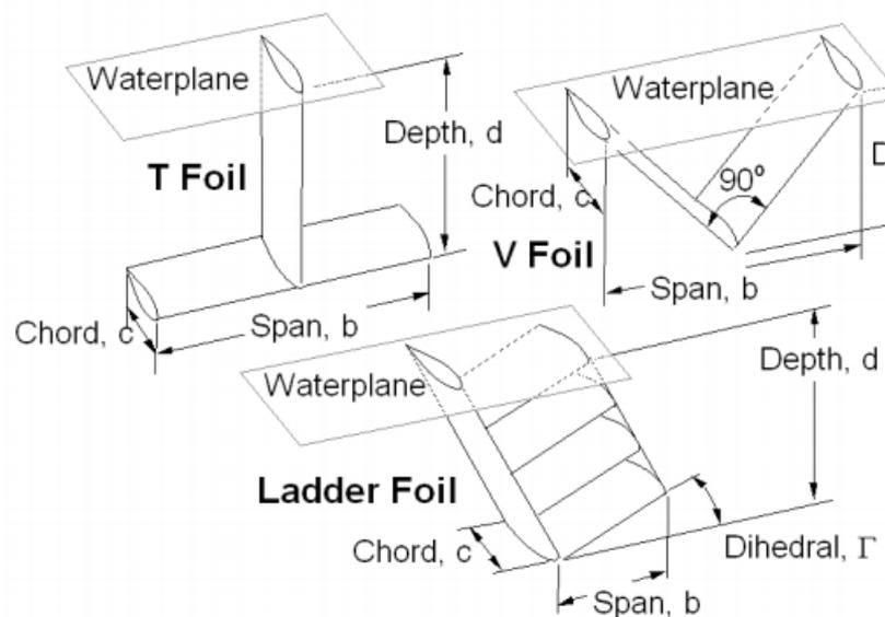
Figure 9: Hydrofoil shapes [32]
