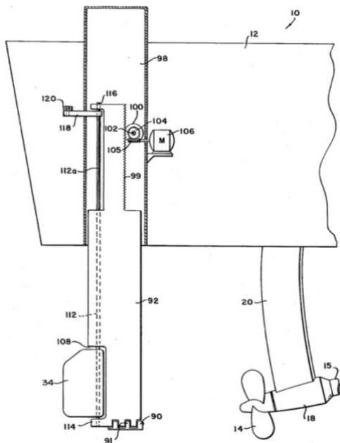
Figure 22: Rack and pinion mechanism retracted hydrofoil system [49]
