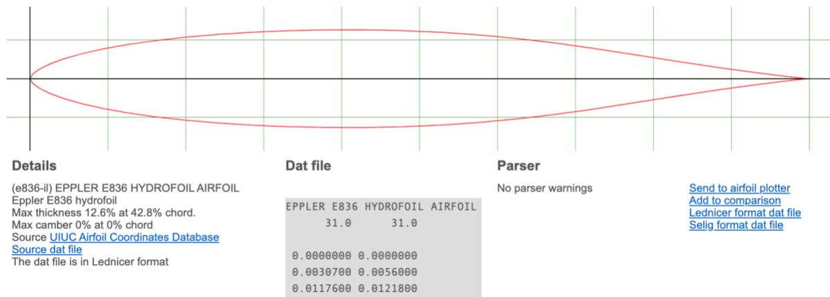
Figure 12: Ei-Foil Eppler 836 hydrofoil profile [33]
