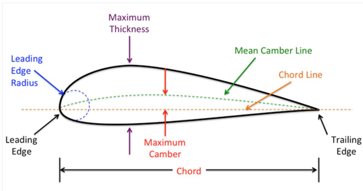
Figure 7: Aerofoil diagram [27]
