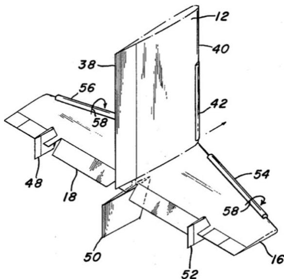
Figure 15: Hydrofoil fixed strut steering control [43]
