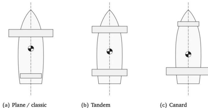
Figure 10: Hydrofoil configurations longitudinal [21]
