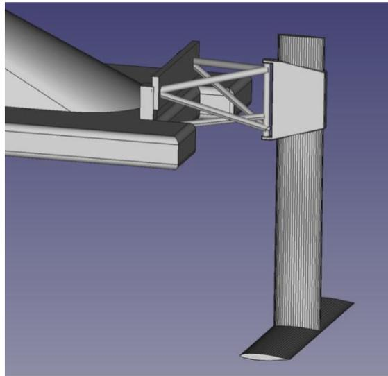
Figure 17: Simplified Basic CAD model of the Ei-Foil Rear
