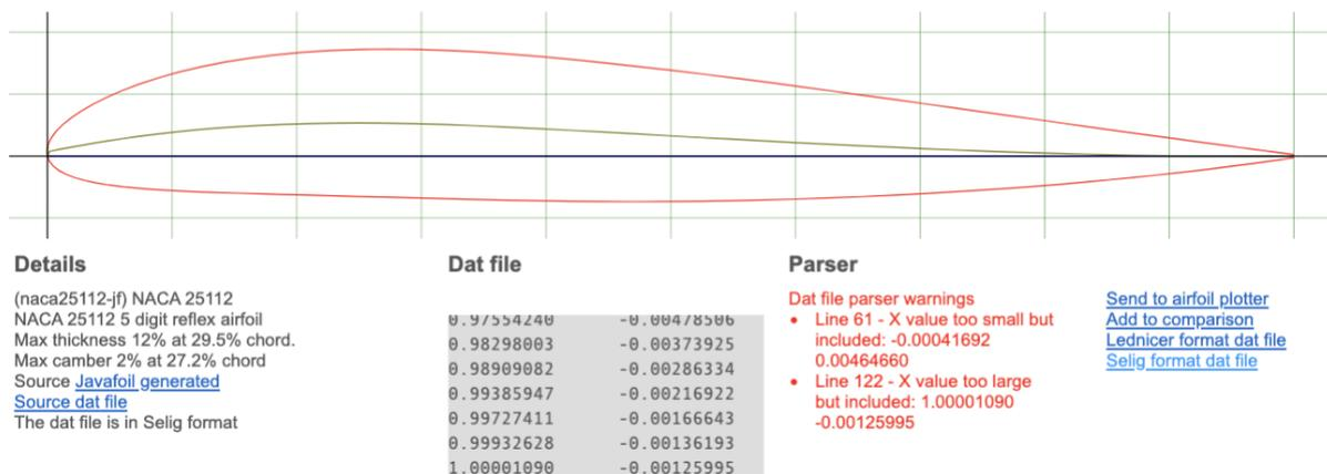
Figure 13: NACA 25112 foil profile [33]
