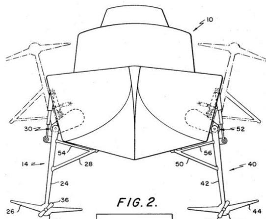
Figure 19: Folding mechanism hydrofoil retraction [47]
