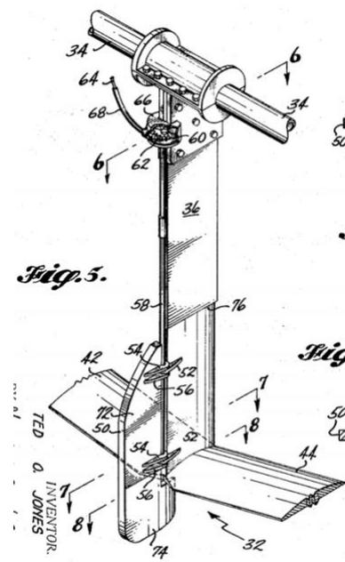
Figure 16: Rudder control on Surface Pierced Hydrofoil [45]
