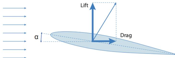
Figure 6: Lift and drag forces with angle of attack [21]
