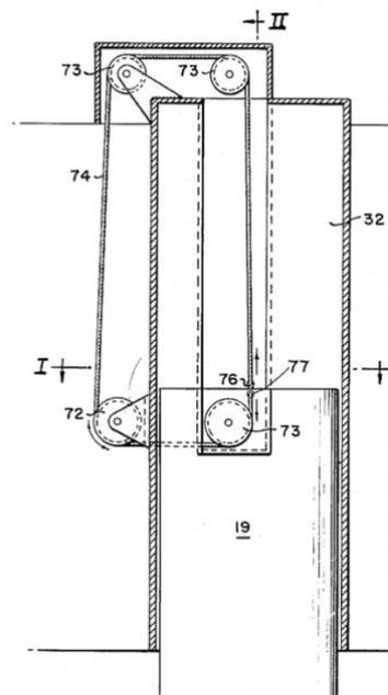
Figure 23: Pulley mechanism hydrofoil retraction system [50]
