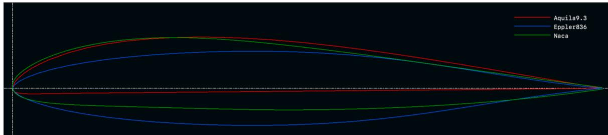
Figure 24: Foil profiles in XFLR5
