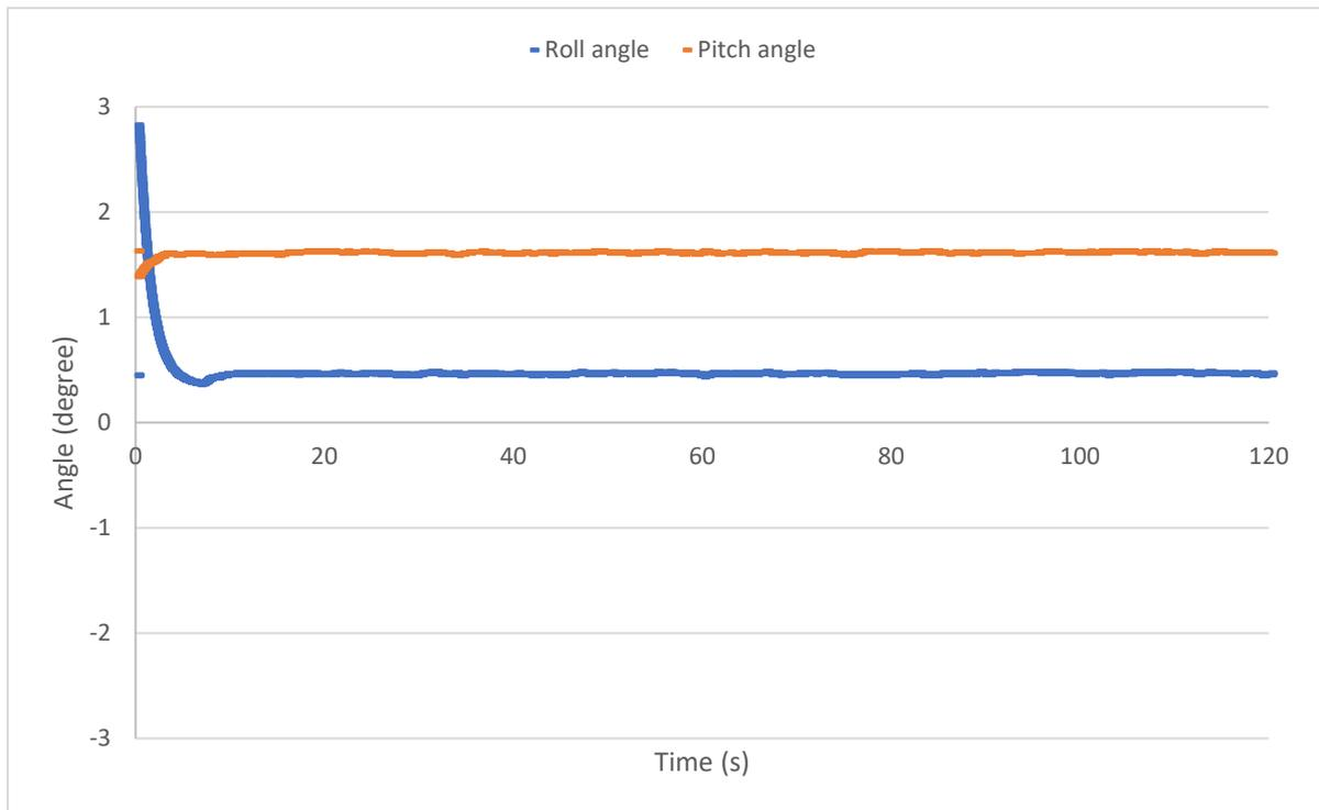
Figure 17 - PhidgetSpatial roll and pitch angle measurements of 120 seconds for trial system test
