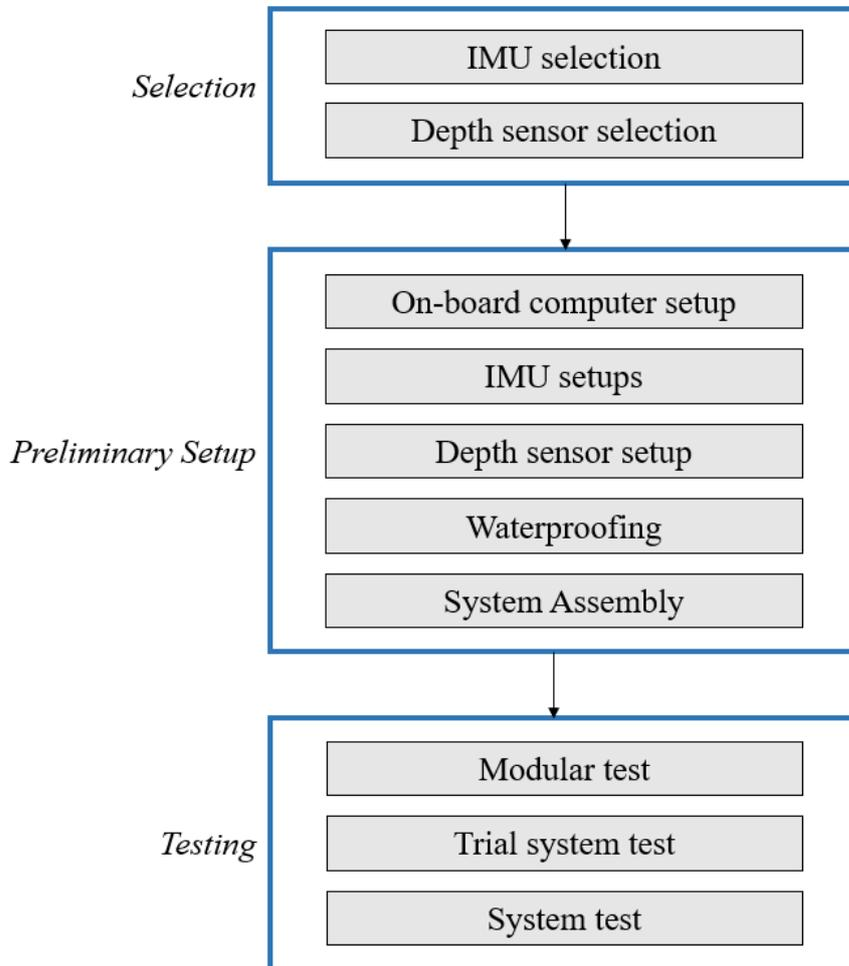
Figure 7 - ODS design process flow chart
