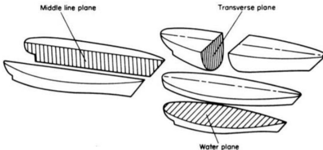
Figure 5 - Planes of a water vessel [12]
