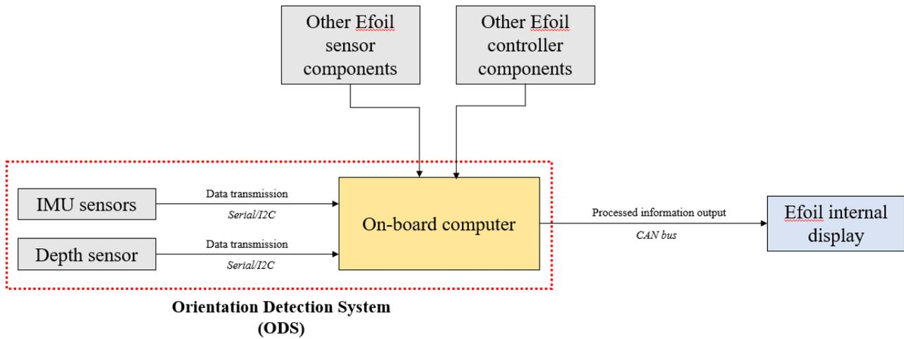
Figure 2 - Block representation of Efoil instrumentation
