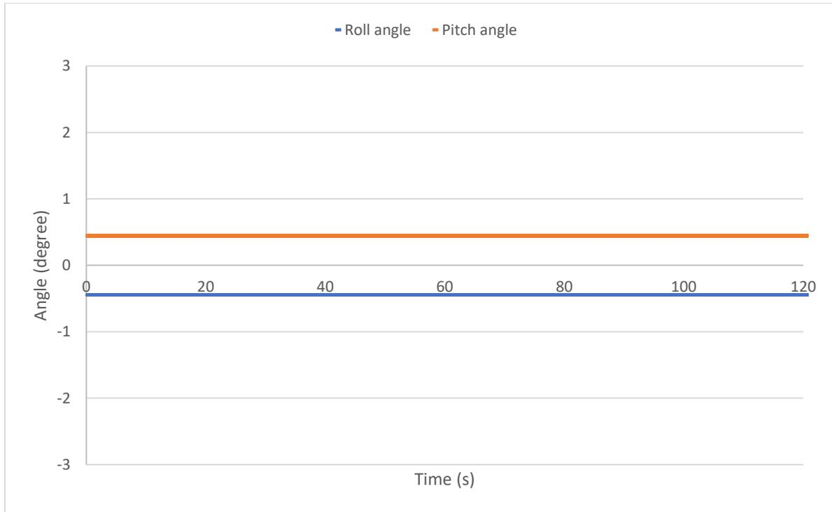
Figure 15 - DFRobot roll and pitch angle measurements of 120 seconds for trial system test
