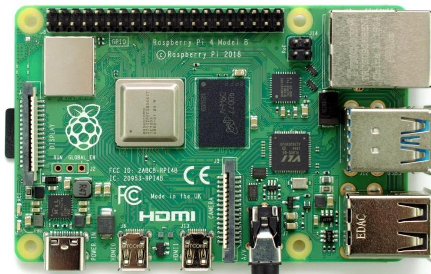
*Figure 8 - Topview of the Raspberry Pi 4 Model B board*
