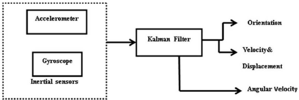
Figure 4 - Block illustration of filtering IMU outputs to obtain pose information [8]
