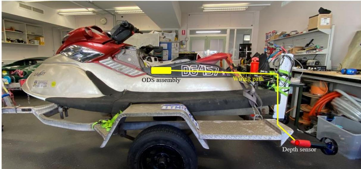
Figure 11 - Depth sensor wire connection within the Efoil
