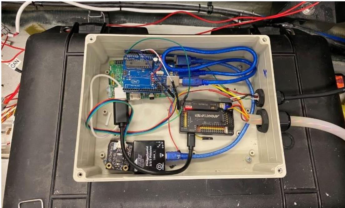
Figure 13 - Final assembly of ODS with cover off
