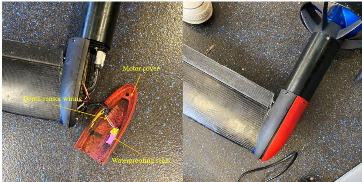
Figure 9 - Left, depth sensor setup within the Efoil motor cover. Right, reinstalled motor cover
