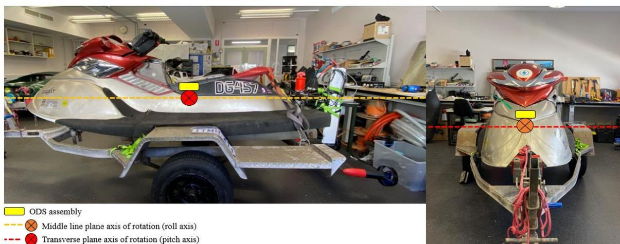
Figure 10 - ODS assembly location. Left, side view of the Efoil. Right, front view of the Efoil
