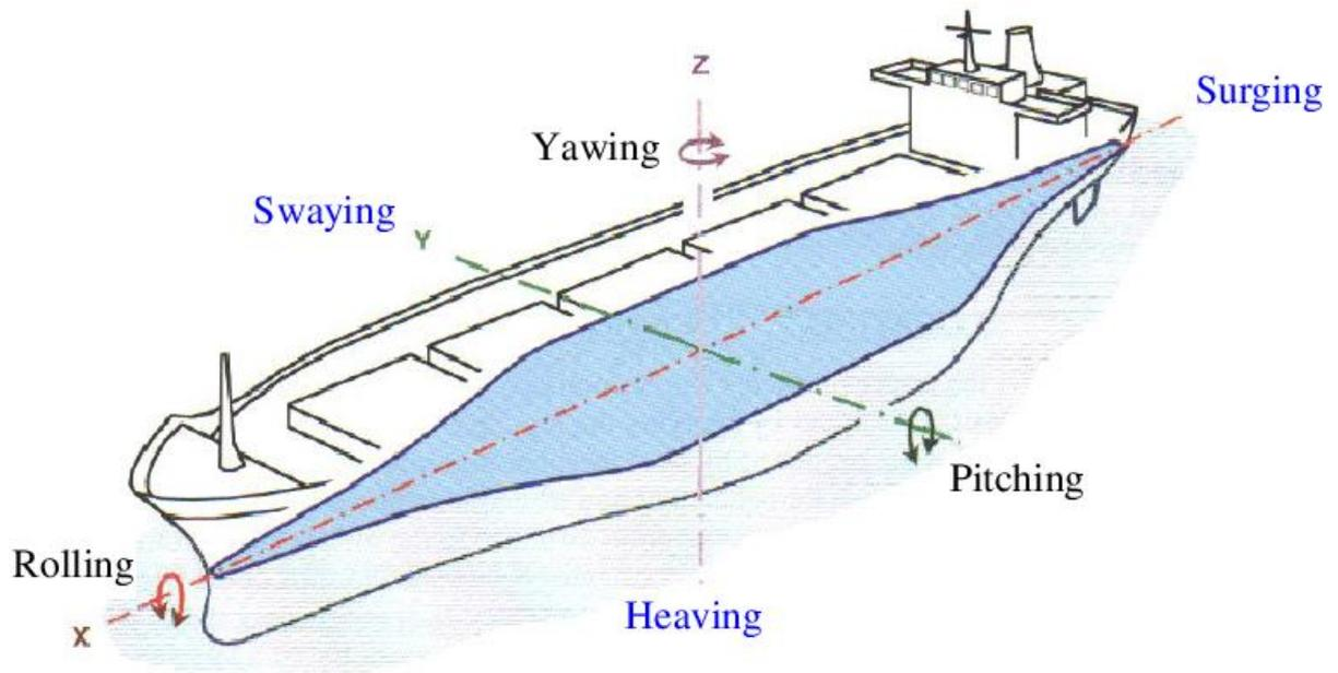
Figure 6 - Notation and sign conventions for water vessel motion description [13]
