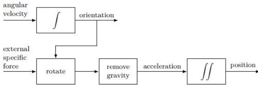
Figure 3 - Block illustration of dead reckoning [3]
