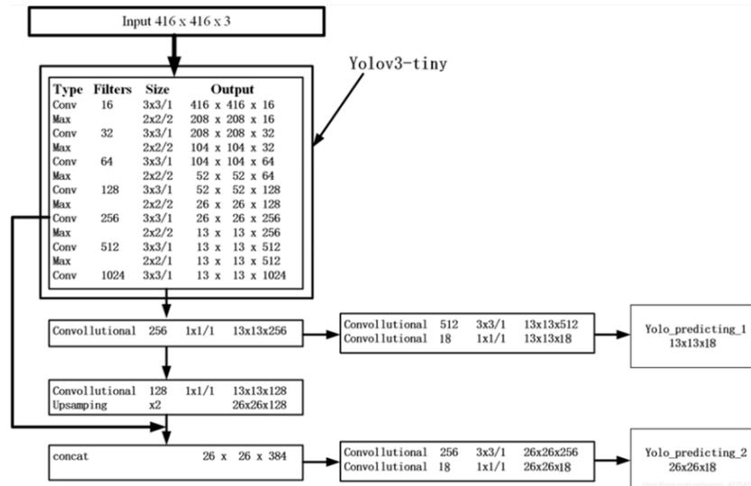
Figure 9. The Network Structure of YOLO v3 tiny for Cone Detection
