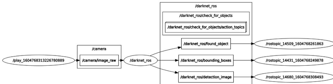
Figure 17. The Rqt Graph of Darknet ROS Node Structure for Cone Detection
