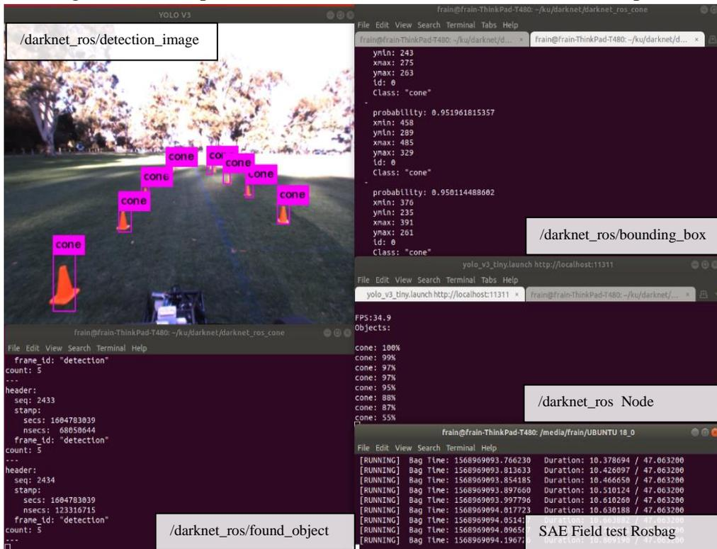
Figure 14. The ROS Implementation of Cone Detection
