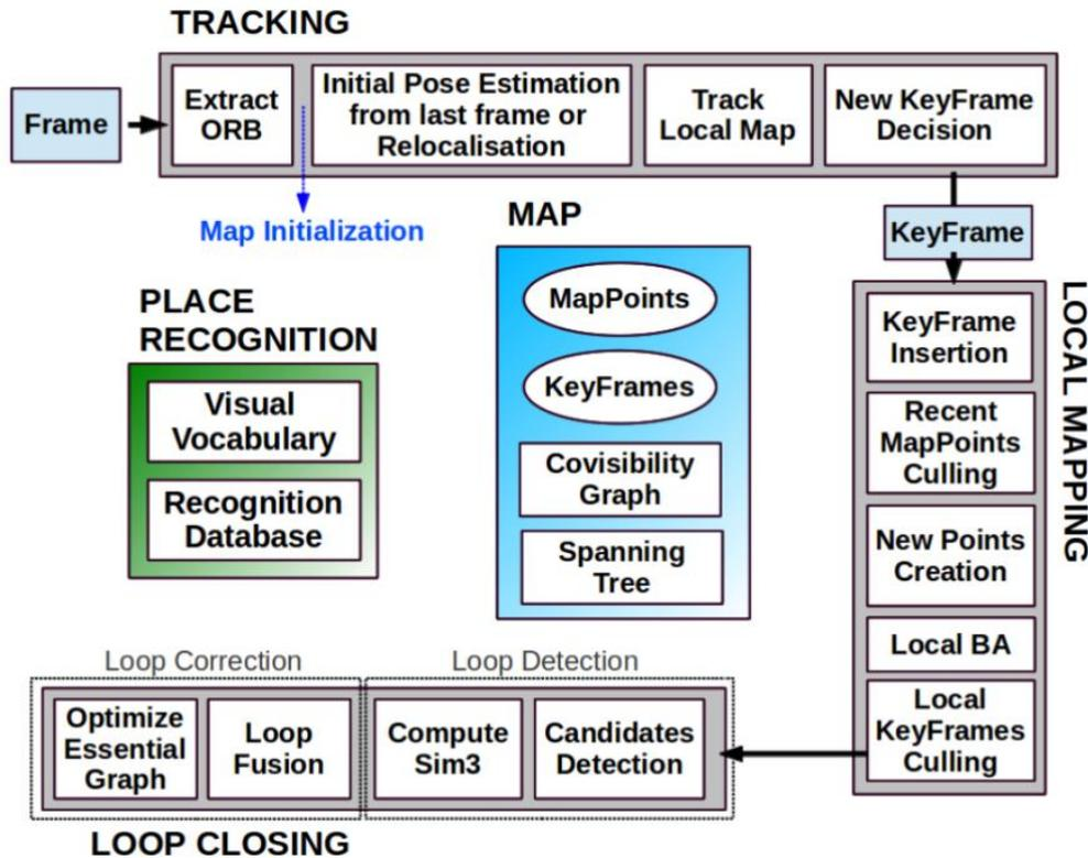
Figure 20. The Structure of ORB SLAM2 [42]
