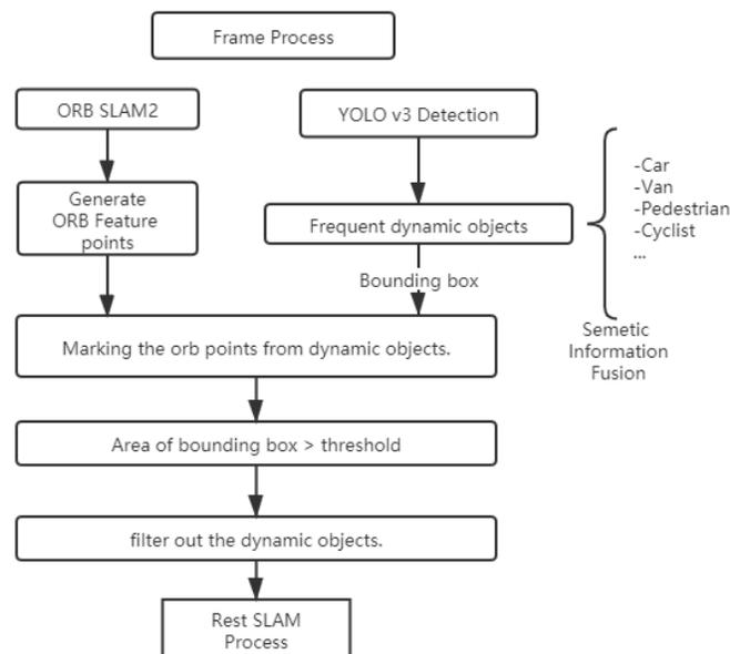
Figure 27. The Design Structure of Detection Mask SLAM
