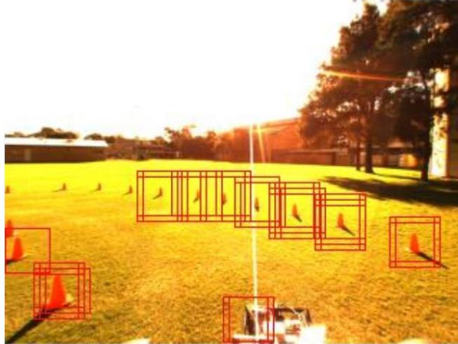
Figure 6. The Previous Detection Work with HOG+SVM
