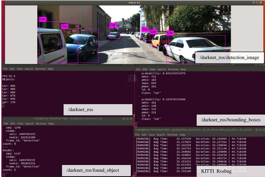
Figure 18. The ROS Implementation of On-road Detection
