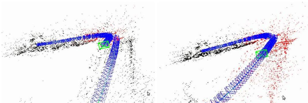
Figure 22. The comparison of ORB SLAM2 without Loop Closing (left) and with Loop Closing (right)
