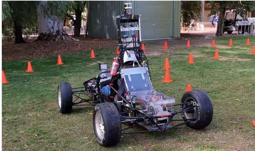
*Figure 2. The Autonomous SAE Electric Car*
