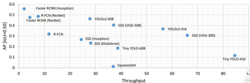
Figure 5. Summary of the Accuracy (AP) and Throughput (FPS) of Various CNN Models [22]
