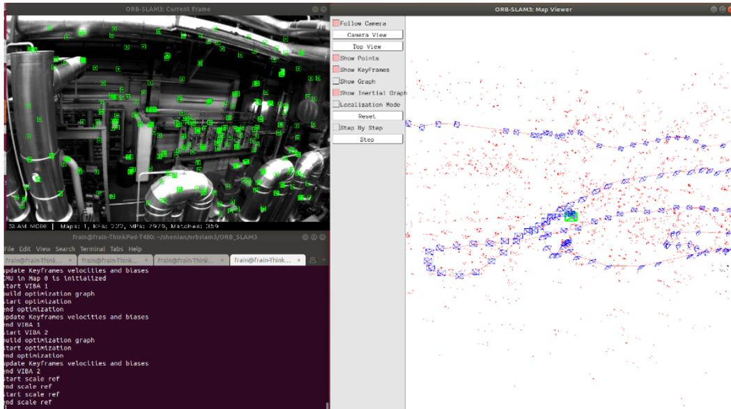
Figure 24. The Monocular ORB SLAM3 with IMU on EuRoC MH01 Dataset
