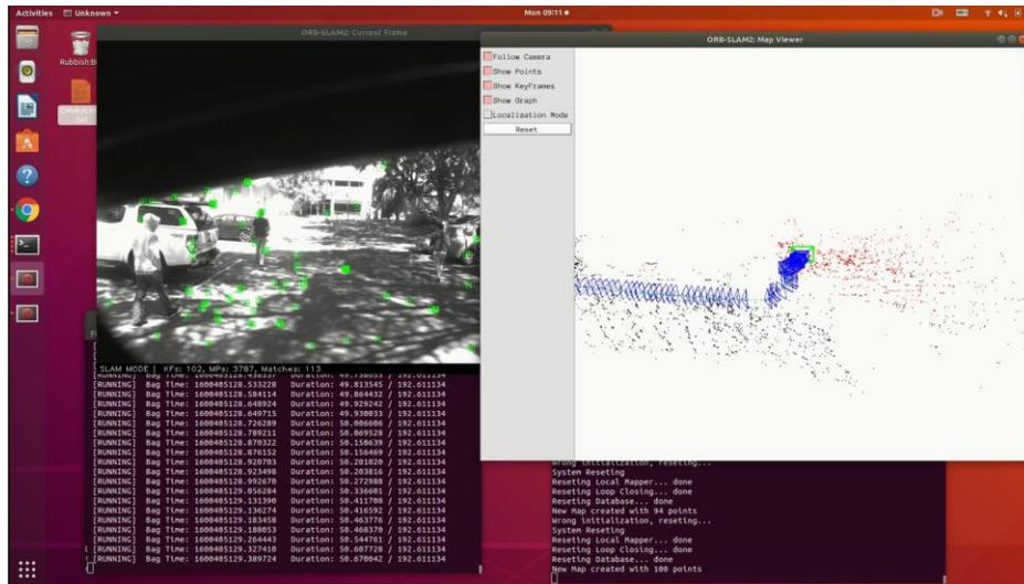
Figure 21. The Loop Closing Test for ORB SLAM2 on nUWay Bus
