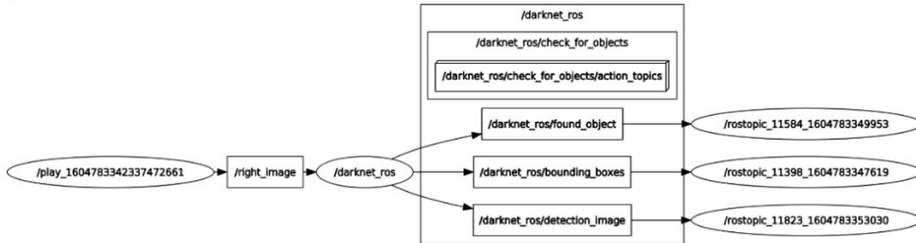
Figure 13. The Rqt Graph of Darknet ROS Node Structure for Cone Detection
