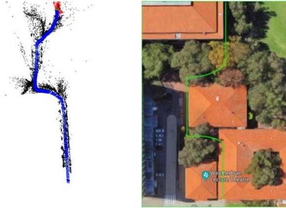
Figure 19. Previous SAE Result of ORB-SLAM2 without Loop Closing [8]
