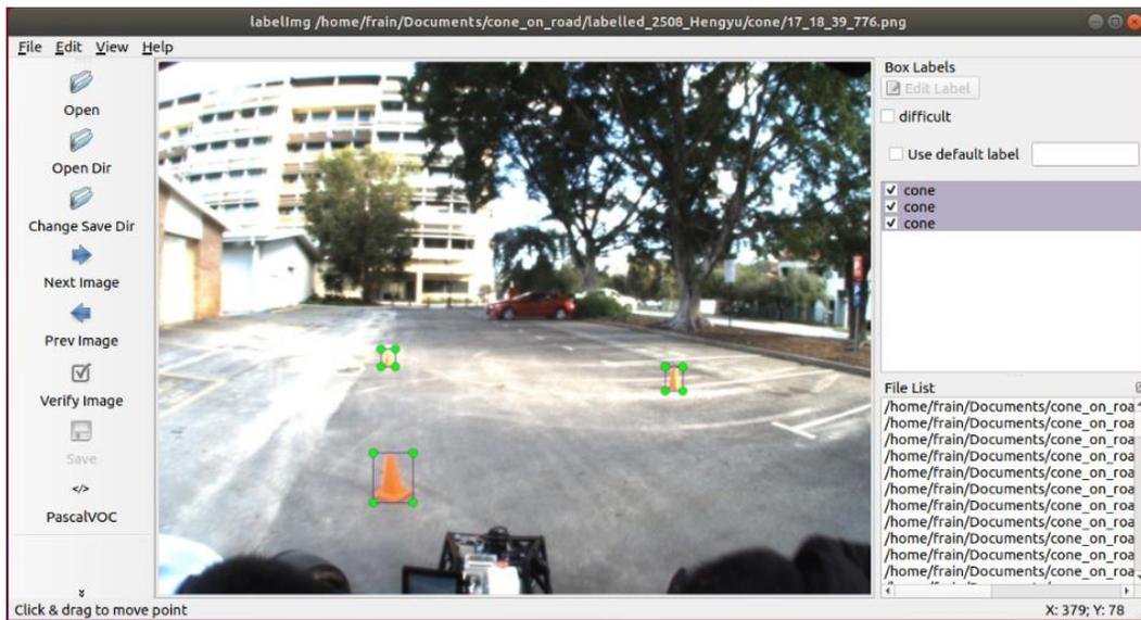
Figure 11. The Cone Labelling with LabelImg Library
