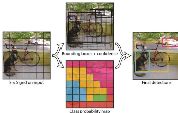
Figure 7. The Detection Structure of YOLO v1 Network [21]
