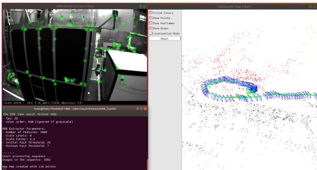
Figure 23. The Monocular ORB SLAM2 without IMU on EuRoC MH01 Dataset
